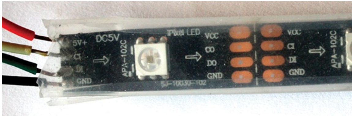
Figure 4-3: The arrows show the direction of the DotStar string.
