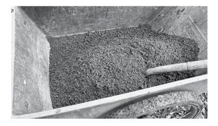
FIGURE 21.2. Clay from a deposit near the pond; it will be mixed with sand and water to make cob.
