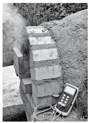
FIGURE 21.4. Thermometer connected to thermocouples shows real-time temperatures in the hearth, the top and back of the oven dome.
