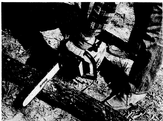
Fig. 9. Proper hand grip and proper stance.
