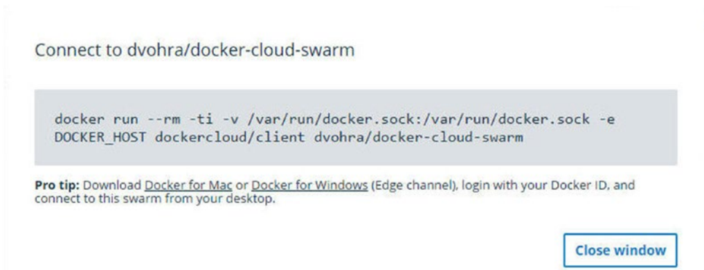
Figure 14-38. Listing and copying the docker run command to connect to the Swarm
