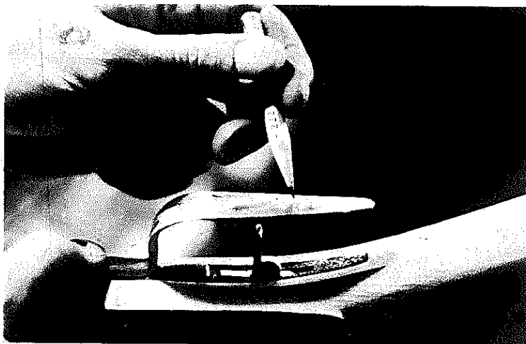
PLATE 284 Hershel points out where to bend the back of the trigger-guard. The part of the guard that is bent down will touch the trigger plate.
