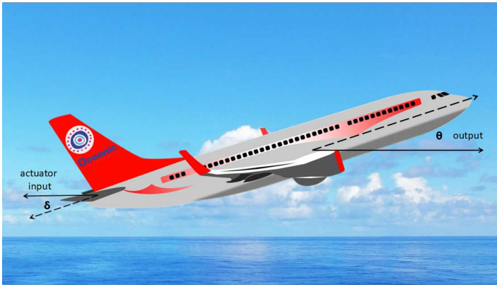
Input \delta and output \theta
