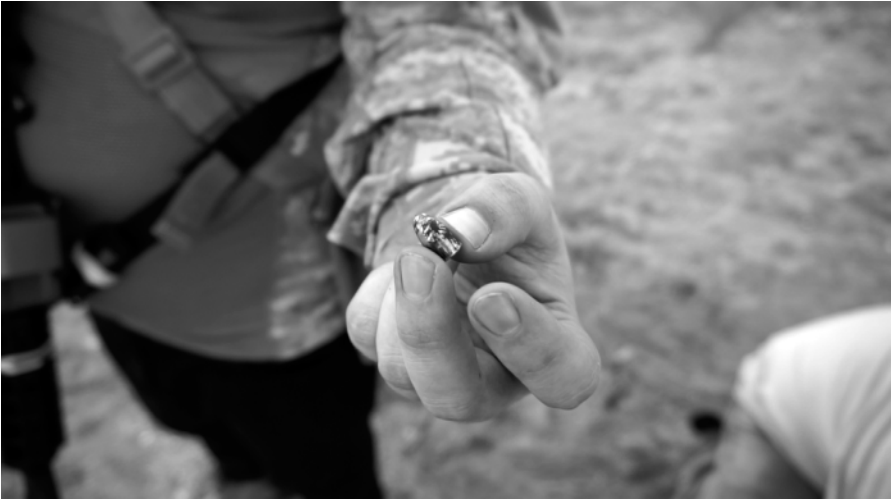
Figure 2.2. 9mm bullet stopped by discarded tires. UNSTOPPABLE, werunstoppable.com
