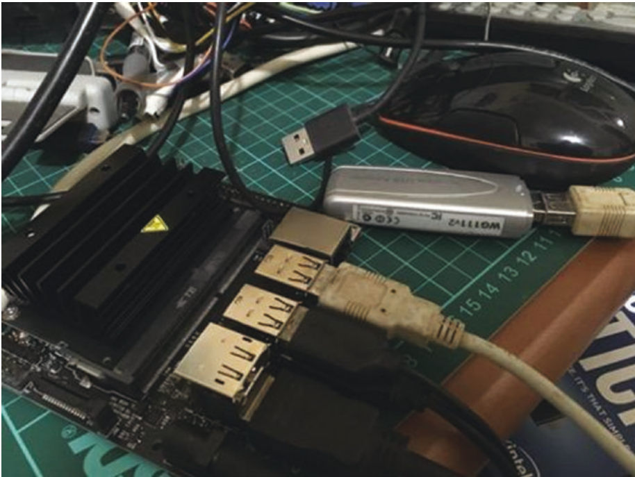
Figure 3-10. Plugging in Wi-Fi USB to NVIDIA Jetson Nano
