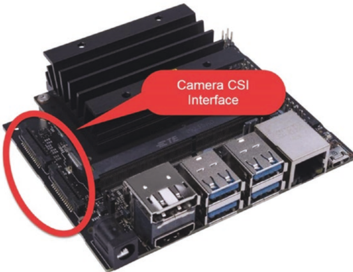
Figure 6-1. Camera CSI interface on NVIDIA Jetson Nano
