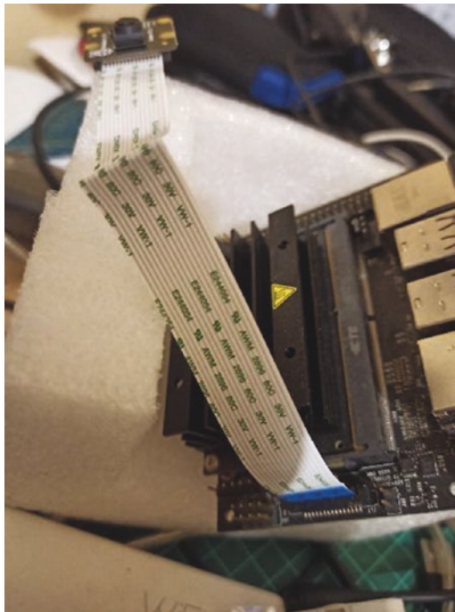
Figure 6-3. Attaching Raspberry Pi NoIR camera to NVIDIA Jetson Nano
