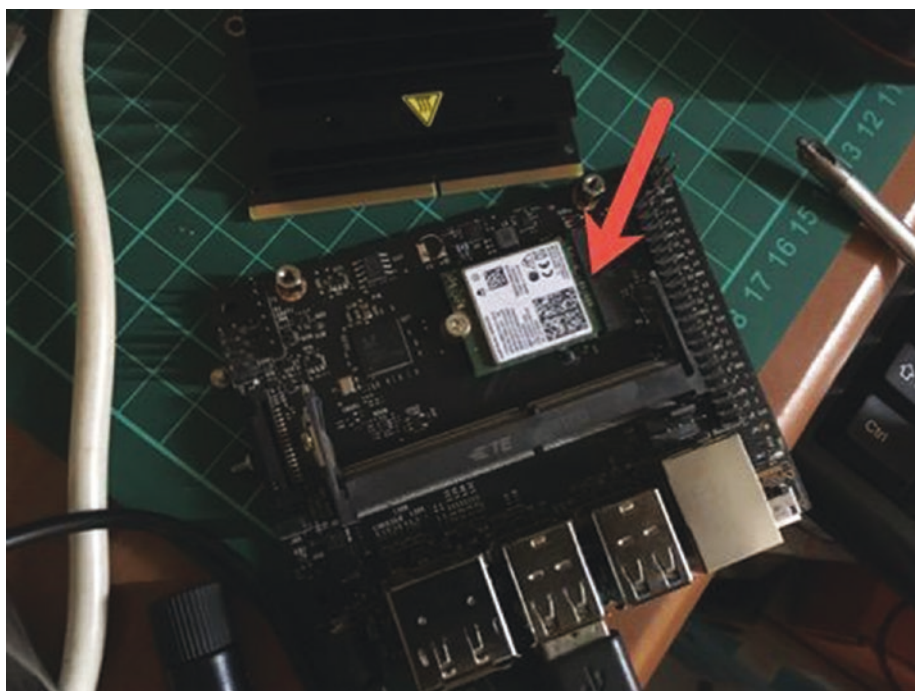
Figure 3-9. Attaching Wi-Fi module into NVIDIA Jetson Nano
