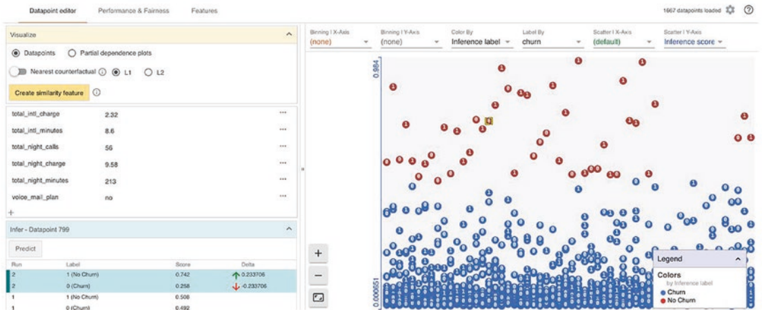
Figure 8-5. Change in the inference score due to a small value change in the features
