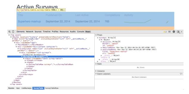
You can see your SurveyTable component get passed an array of surveys that contains timestamps. In the actual view, they're presented in a human readable format. Double-click one of the timestamps and type in a new value. This causes the component to update with the new value.
