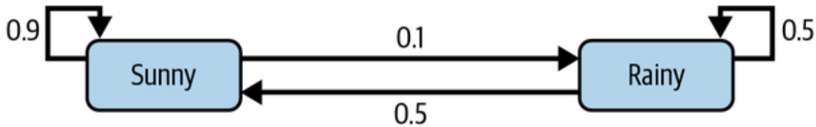
Figure 1-2. A graphical representation of a simple two-state weather prediction model
