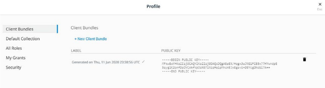
Figure 6-7. Generate a new client bundle
