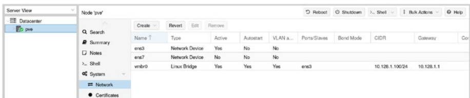
Figure 2-4. The network view for the lab host, which shows the two physical interfaces, ens3 and ens7 , and the vmbr0 bridge Proxmox created automatically when you installed the system
