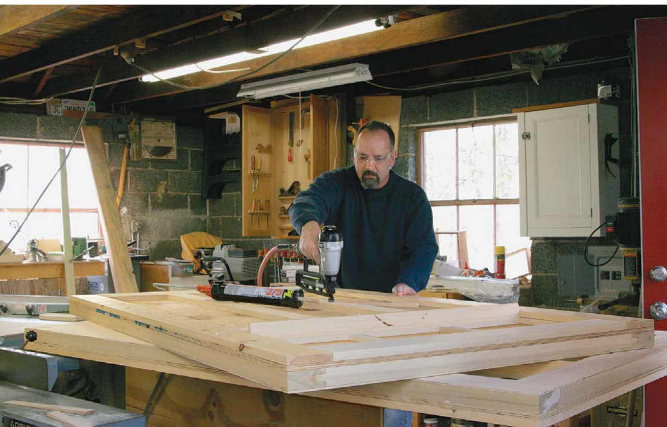
Pine dresses up the plywood. Pekovich applied flat pine pieces to create a frame-and-panel effect and an Arts and Crafts look.
