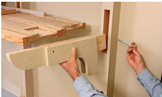
Simple mounting system. Lumber rests on a series of support arms that are bolted to stanchions.
