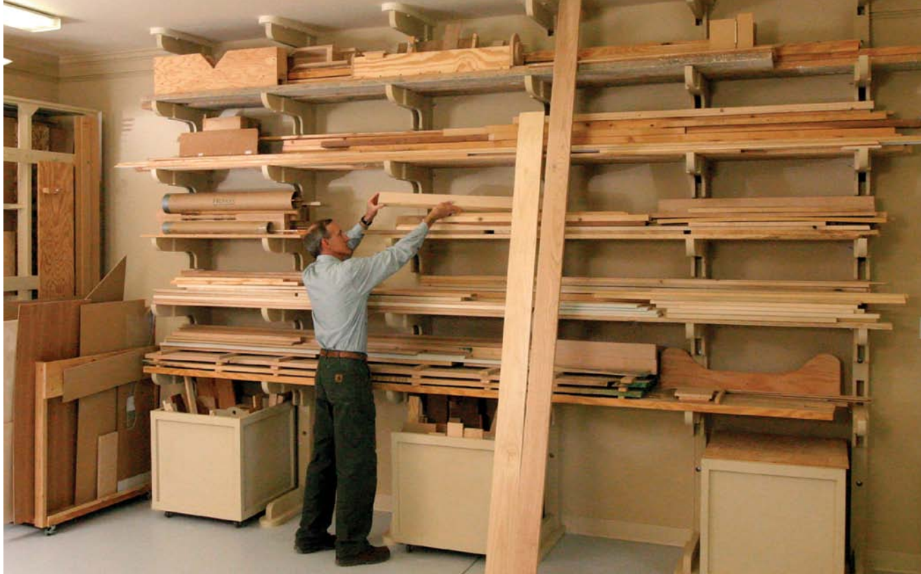
Lumber at the ready. A wall-mounted rack keeps lumber organized and accessible without taking up valuable floor space.
