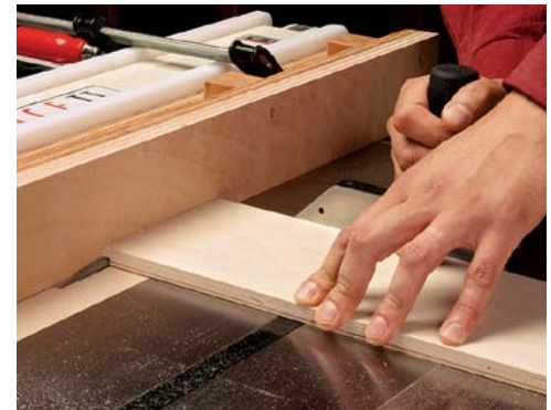
Rabbet the fronts and backs. With the dado head buried in a sacrificial fence, cut the rabbets for the corner joints.
