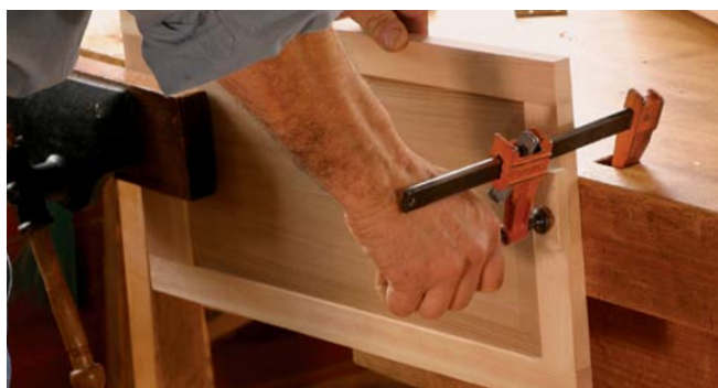
Hold wide workpieces on edge. The vise screw prevents a wide piece from going all the way through the vise (top). A clamp seated in a dog hole provides extra support (above).
