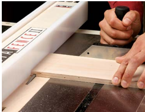
Dadoes in the sides. Use a miter gauge to guide the drawer sides safely along the rip fence.
