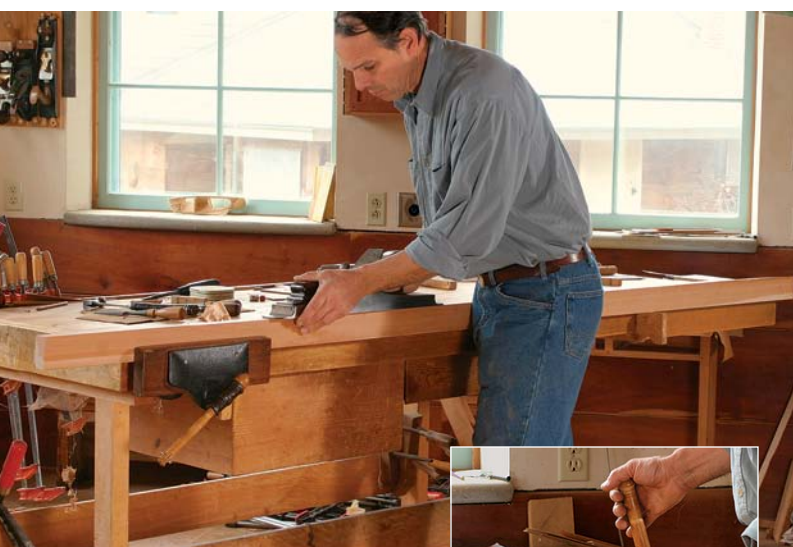
Secure long boards on edge. A block clamped in the tail vise supports the opposite end.
