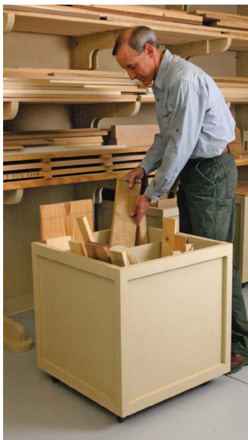
Rolling cart adds convenience. A framed plywood box on wheels provides the perfect place to store offcuts.
