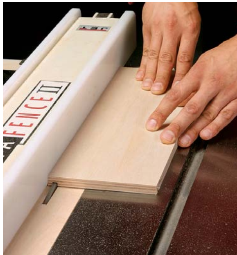
Grooves for the bottoms. Run the bottom of the sides, fronts, and backs against the fence to cut the groove for the bottom panel.
