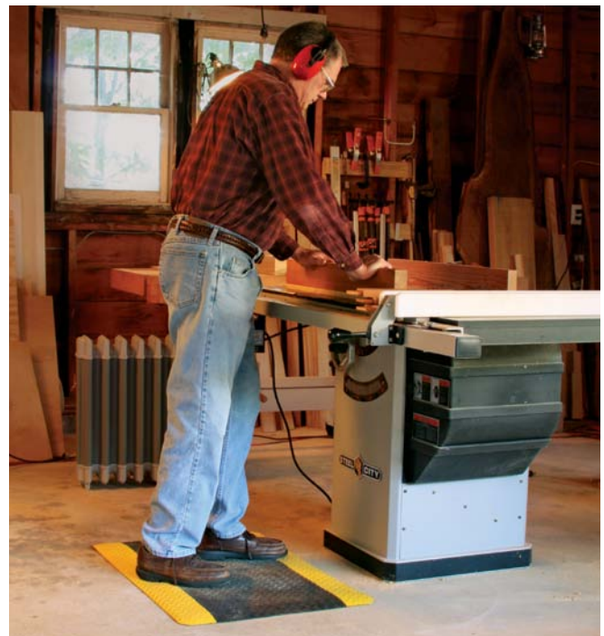
Insulation. Cold floor, warm feet. A mat is a barrier between your feet and a chilly concrete slab.
