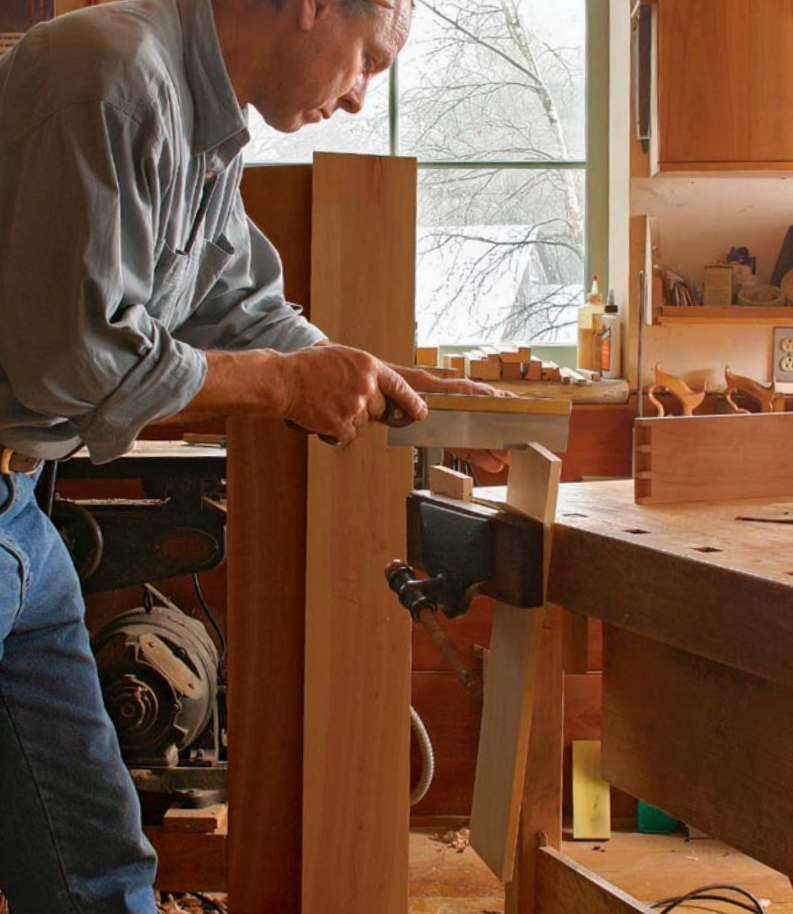
A front vise holds work vertically for sawing dovetails or planing end grain. A scrap piece of similar thickness, clamped in the opposite side of the vise, prevents the vise from racking.
