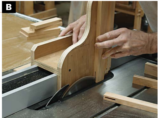
CUT THE BRIDLE with a tenoning jig. With the face side of each stile facing the tenoning jig, make a \frac{1}{8} -in.-wide cut, then adjust the fence to widen the cut to \frac{3}{16} in.
