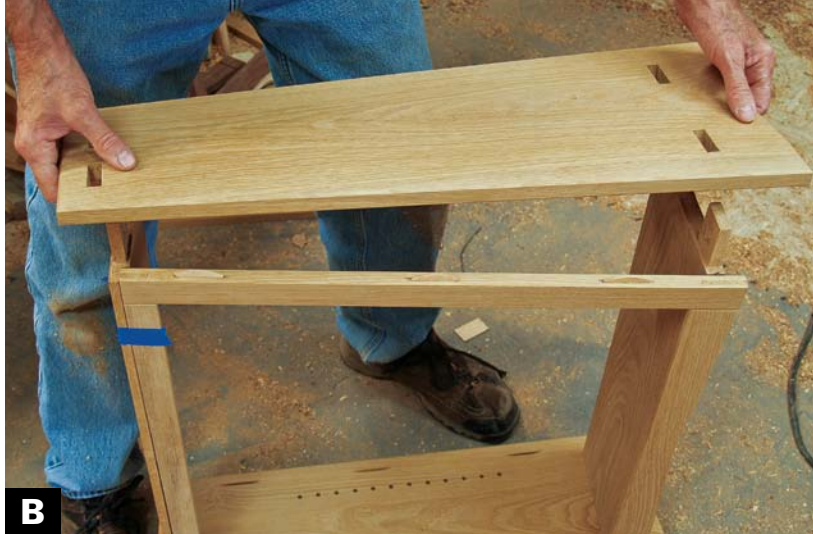
PUT THE WEDGES IN ONE SIDE to hold the parts tight while you align the other side over the tenons.
