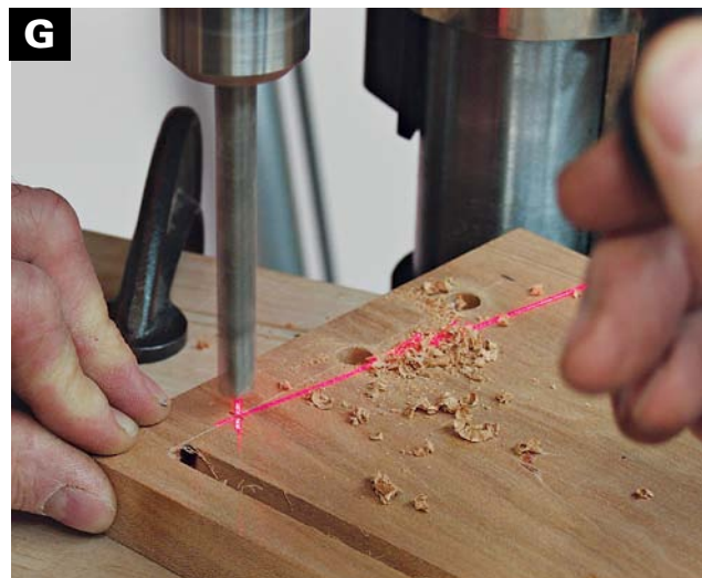
DRILL THE DOWEL HOLES ON THE DRILL PRESS. Using a brad point bit makes it easier to center the bit on your marks. Also drill the holes for the door post.
