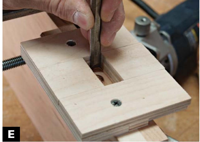
SQUARE UP THE CORNERS of the mortise with a corner chisel or straight chisel.
