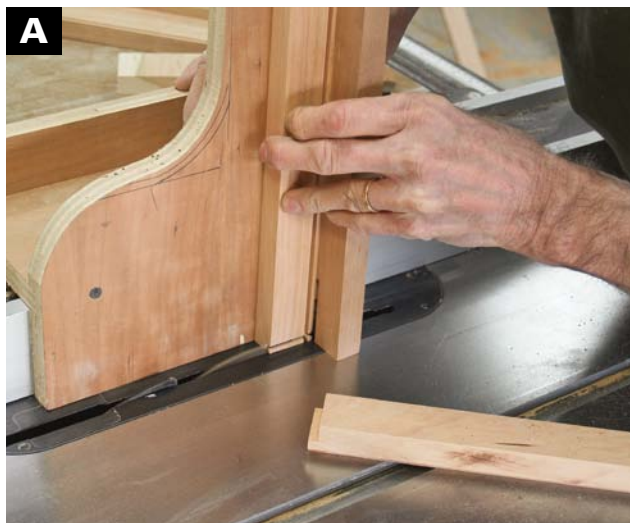
USE A TENONING JIG to cut the tongues on the bottom and shelf fronts. Size the tongues to fit the grooves in the carcass parts, \frac{1}{4} in. long \times \frac{1}{2} in. thick.
