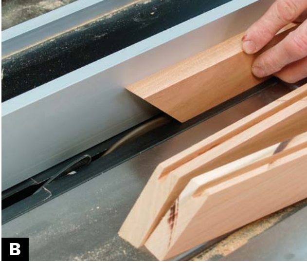
B CUT GROOVES IN THE INSIDE EDGES of the lower moldings to fit the tongues on the top.
