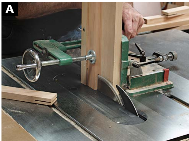
A CUT THE SLOTS AT THE ENDS of the door stiles on the tablesaw with a tenoning jig. I make a cut on each piece and then adjust the jig to widen the cut to \frac{1}{4} in.
