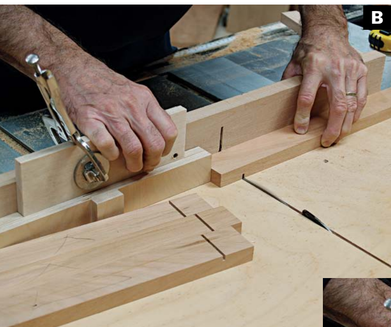
B MAKE A \frac{3}{16} -IN.-DEEP CUT in each end of the door rails with the outside face down on the surface of the sled.
