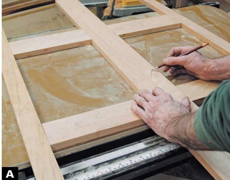
A ARRANGE THE STOCK FOR THE FRAME to achieve the best grain match. Mark the parts carefully so you'll remember where each goes.
