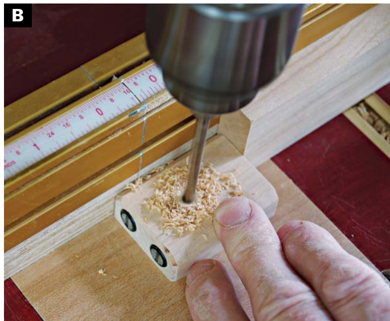
DRILL AND COUNTERSINK a hole for the mounting screw. Install the metal catches on the doors, then drive the screw to attach the stop.
