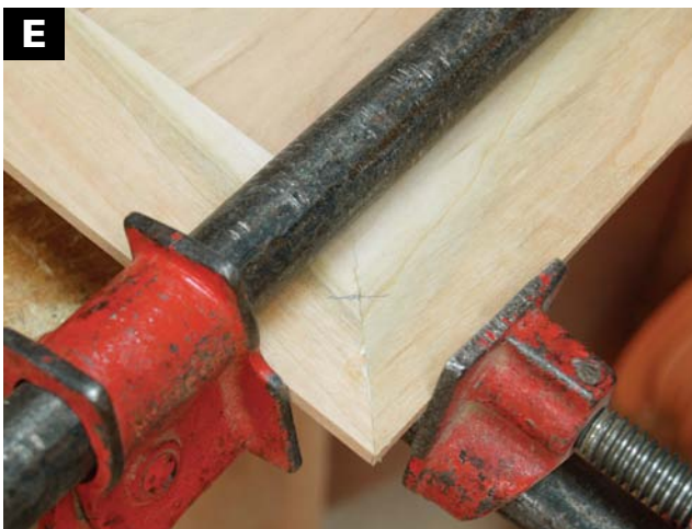
E USE BAR CLAMPS to pull the biscuited joints tight.
