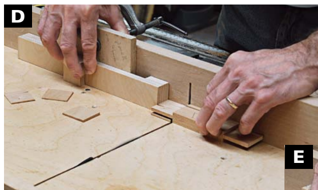
CUT THE SHOULDERS OF THE RAILS on the crosscut sled. Here, I'm using a special stop block to avoid trapping the cut-off between the blade and the stop. Easily made from scrap wood, the stop moves into position to set the correct distance from the blade, then moves away for the cut.
