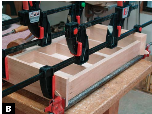
PULL THE JOINTS TOGETHER with clamps after the biscuits and glue are in place.
