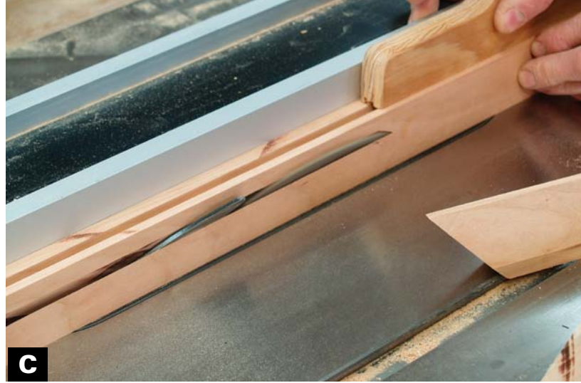
C TILT THE TABLESAW BLADE to cut the molding parts to shape. Use a push block for safety.
