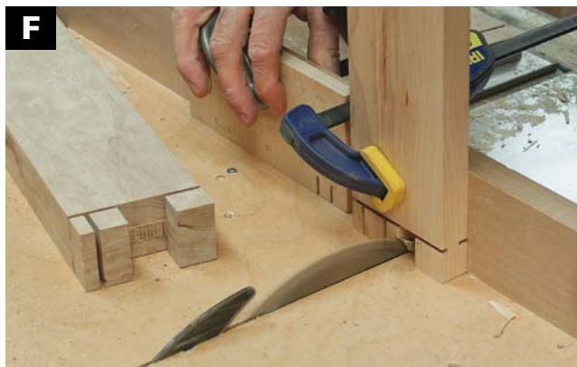
REMOVE THE WASTE between the double tenons by taking repetitive passes over the blade. Each cut removes \frac{1}{8} in.
