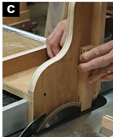
TO LAY OUT the rail tenons, use the bridle in the stile for the setup. Cut on the waste side of the transferred line. Make your first cut with the face side against the jig. Then move the fence to cut the other side, again with the face side of the stock against the body of the jig.
