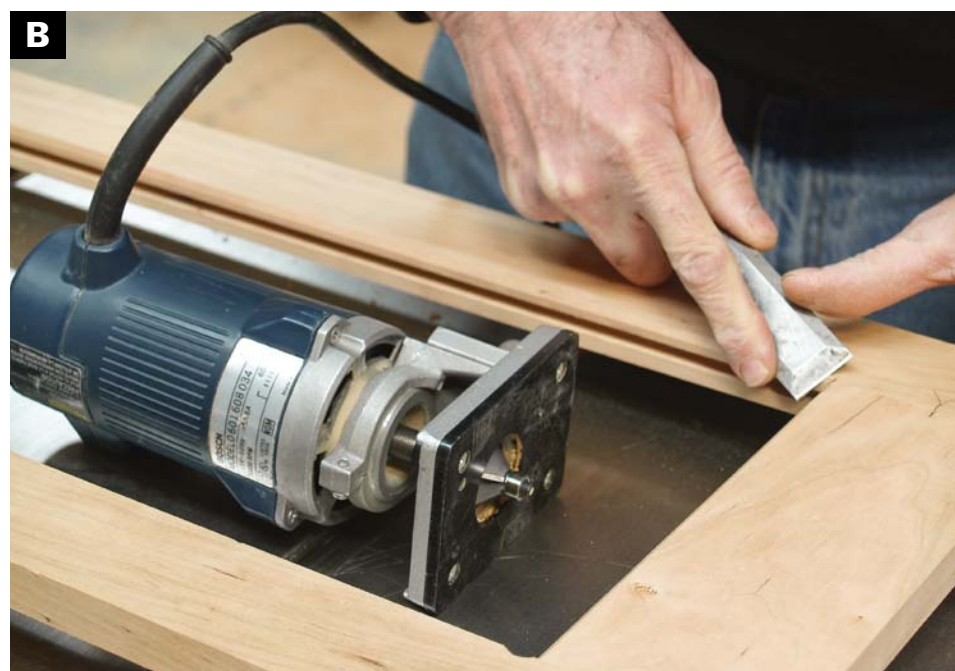
ASSEMBLE THE FRAME with dry biscuits and hold it together with clamps. Use a hand-held router with a 45° chamfering bit to rout the inside edges. Cut from both sides with a sharp chisel to finish the corner cut.
