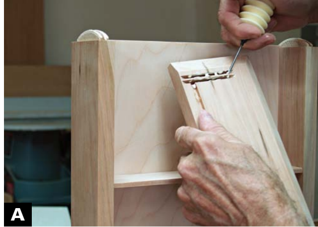
APPLY GLUE IN THE BISCUIT SLOTS and then insert the biscuits.
