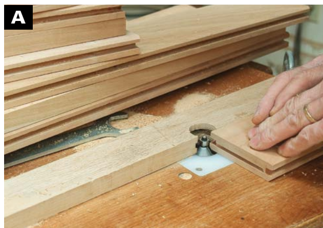
USE A 45° CHAMFERING BIT mounted in the router table to rout the inside edges of the rails and stiles.
