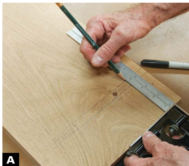
CAREFULLY LAY OUT THE MORTISES in the sides. I shade the area to be removed so I can double-check the setup on the mortiser.
