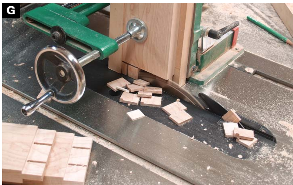
REMOVE THE WASTE between the double tenons by taking repetitive passes over the blade. Each cut removes \frac{1}{8} in.
