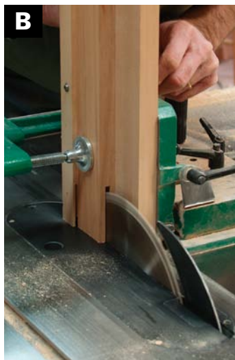
B CUT THE BRIDLE SLOTS with a tenoning jig. Keep the back face of the frame against the jig. Widen the slot to \frac{1}{4} in. on a second pass.
