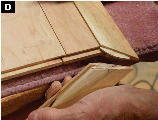
D TO ASSEMBLE THE MOLDINGS , use the assembled top unit to help hold the parts in position as the glue sets.
