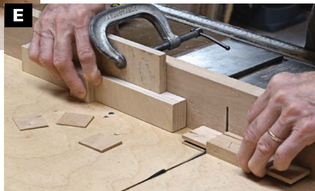
CUT THE SHOULDERS OF THE RAILS on the crosscut sled. Here, I'm using a special stop block to avoid trapping the cut-off between the blade and the stop. Easily made from scrap wood, the stop moves into position to set the correct distance from the blade, then moves away for the cut.
