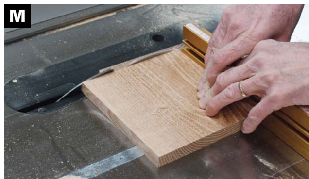
CUT A 15° ANGLE where the two roof sections intersect. Cut the sections to length with a crosscut sled.
