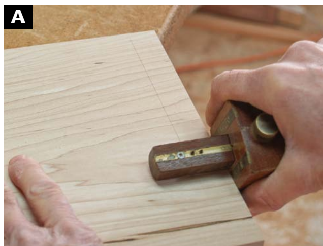
LAY A GAUGE LINE on the cabinet top, bottom, and sides to define the depth of your pins and tails.
