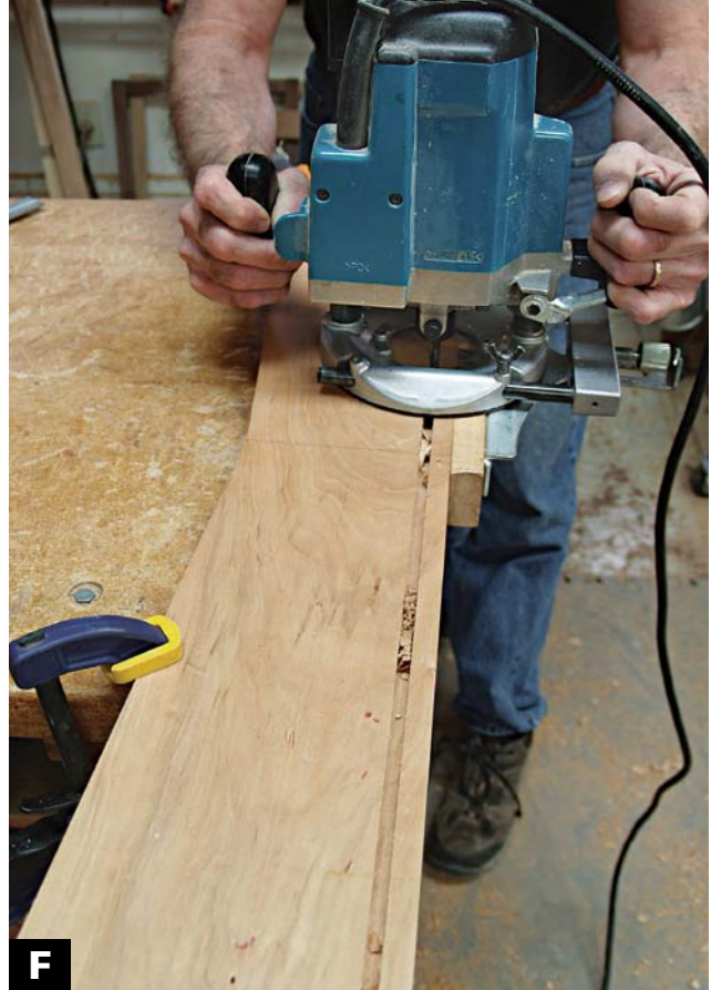
ROUT THE GROOVE FOR THE BACK on the inside surfaces of the top and bottom with a plunge router and edge guide.
