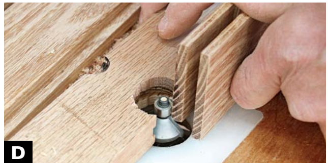
D ROUT THE EDGES OF THE DOOR SLATS with a \frac{1}{8} -in. roundover bit. Adjust the height to rout the "short" side.
