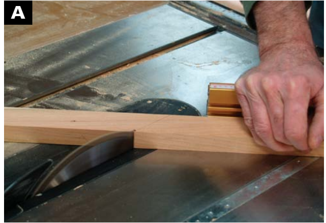
TO MAKE THE PARTS FOR THE TOP MOLDINGS, use a miter gauge set to 45° and cut on the tablesaw.
