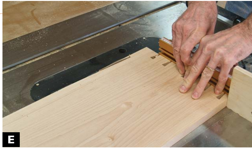
CUT THE 3^\circ ANGLE on the top, bottom, and shelf from the front center to each end. I use a precision miter gauge and stop block to position each cut.
