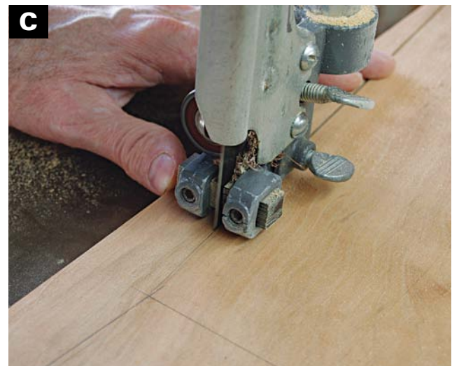
CUT THE FRONT PROFILE on the bandsaw. Stay just outside your line to allow smoothing after the cut.
