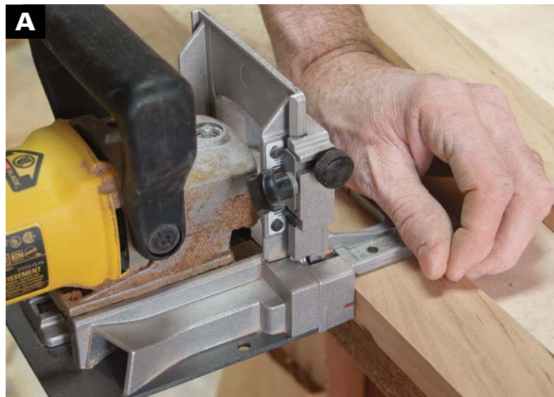
CUT SLOTS for #20 biscuits in the side rails with a biscuit joiner.
