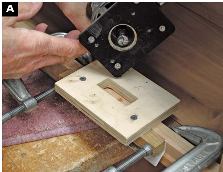
ROUT THE HINGE MORTISES using a shopmade hinge template. Note the card stock used to shim the position of the template for routing the mortises in the doors.
