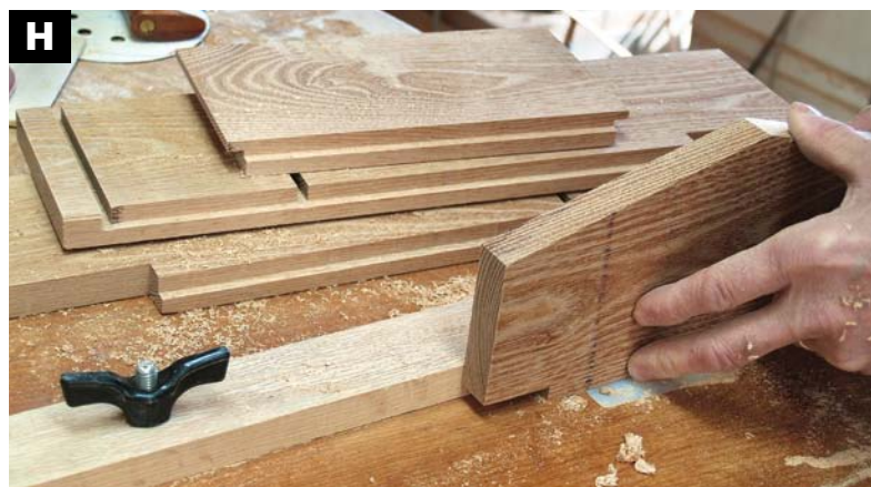
ROUT THE MATCHING RABBET in the back gable with the part standing on edge.
