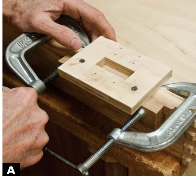
A HINGE-ROUTING TEMPLATE makes it easy to rout the hinge mortise in the cabinet sides and doors.
