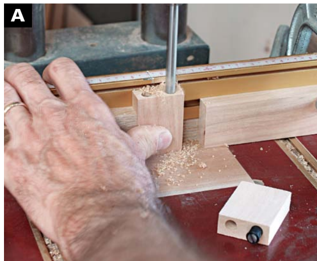
DRILL FOR THE MAGNETIC CATCHES with a drill press. Measure to make sure to drill deep enough.
