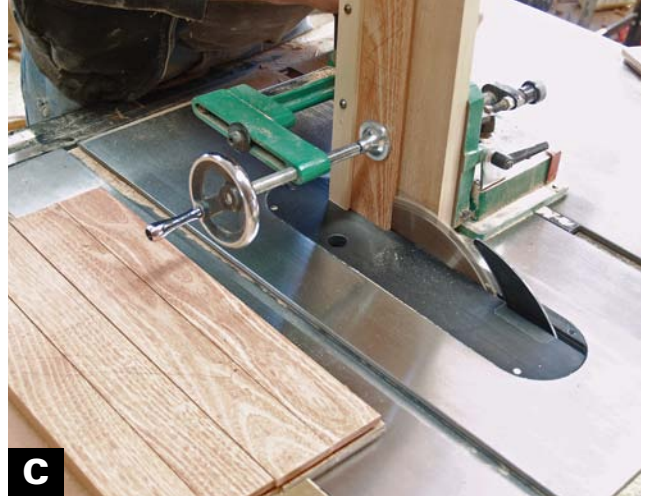
C USE A TENONING JIG TO CUT THE SLOTS in each end of the door slats.
