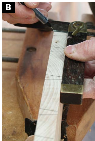
MEASURE AND MARK the position of the pins. Use a sliding T-bevel to lay them out at the correct angle. I use a fine-tipped black pen for the clearest mark.
