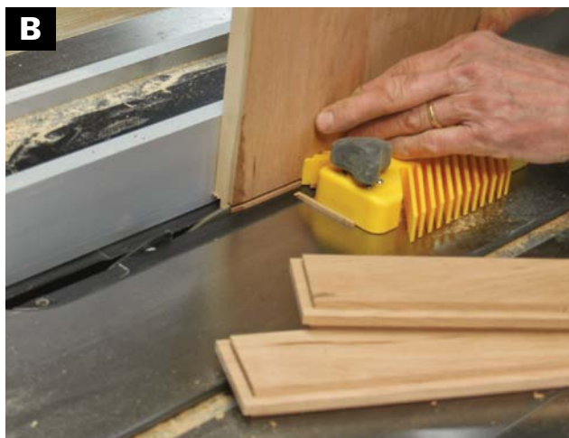
MAKE THE CUTS ON THE ENDS first and then the sides. The front and back parts of the top are also shown.
