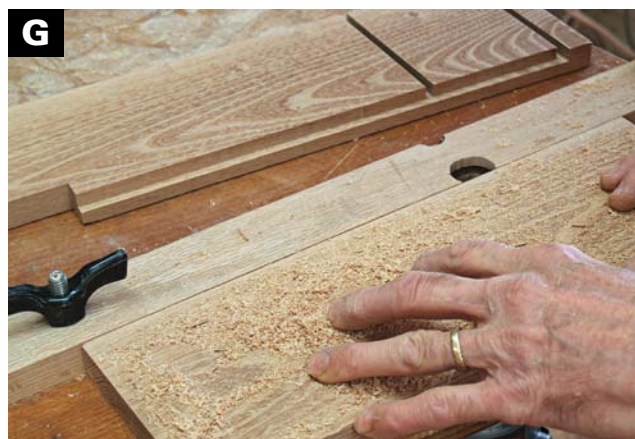
ROUT RABBETS ON THE INSIDE BACK EDGES of the sides for the back panel. I use a stop on the router table fence to keep the cut from going all the way along the back edge.
