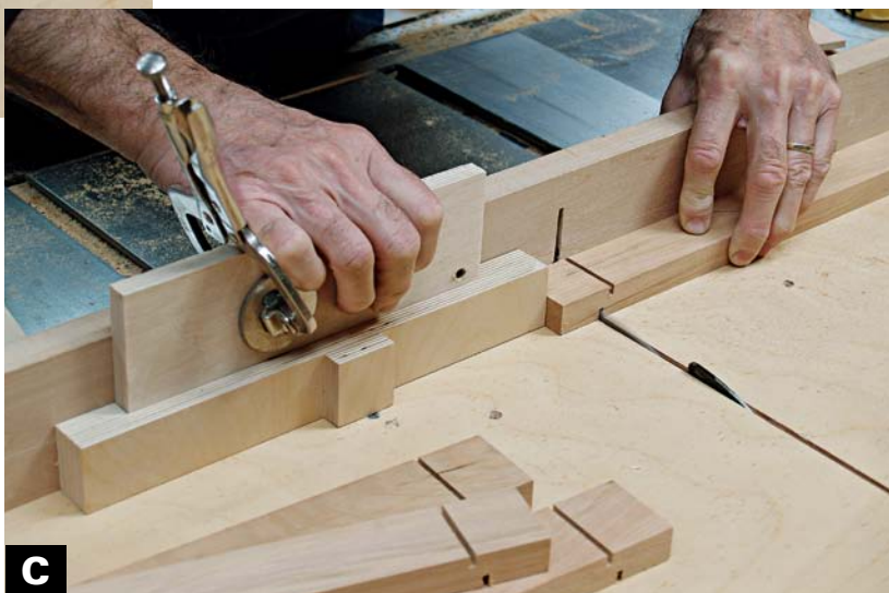
B MAKE A \frac{3}{16} -IN.-DEEP CUT in each end of the door rails with the outside face down on the surface of the sled.
