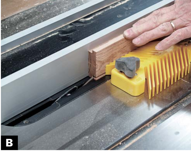
B COMPLETE THE LAP JOINT by adjusting the fence and blade height and cutting the stock on edge.
