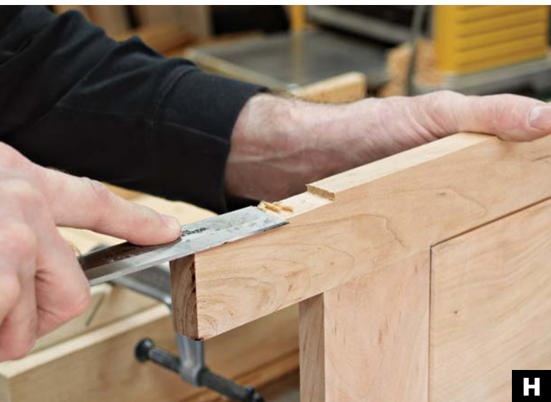
CLEAN UP THE NOTCH for the base molding with a sharp chisel. You can rough out the notch on the tablesaw with the blade raised to \frac{1}{8} in. and a stop block positioned to make the first cut at 3\frac{1}{2} in. from the blade.
