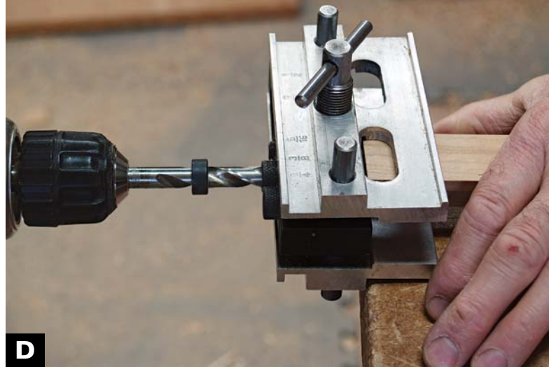
D DRILL DOWEL HOLES at each end of the door post. Very careful alignment is critical so that the door stop is perfectly centered and vertical in the finished cabinet.
