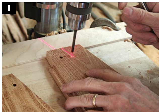
DRILL \frac{1}{4} -IN. HOLES FOR THE DOWELS in the front and back gables 1 in. on center from both sides. Set the drill press to drill through the stock.
