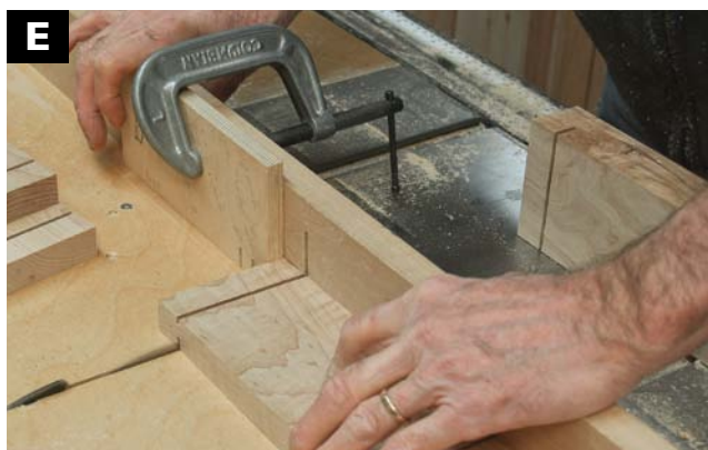
CUT THE TENON SHOULDERS on a crosscut sled. Set a stop block to establish a tenon length of 1 in.
