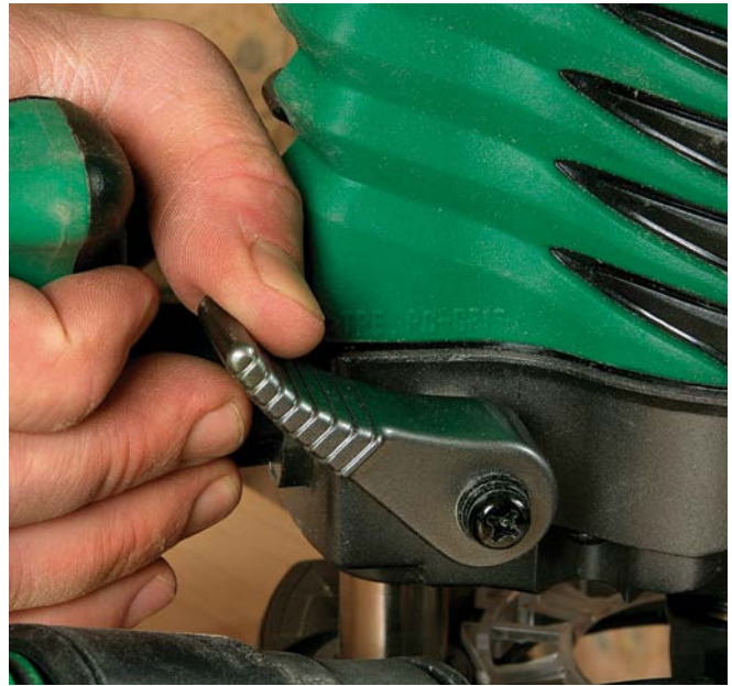
Levers control plunge on most routers. The best ones, like on the Hitachi, can be reached without letting go of the handle, and require little force.
