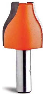
Panels. A vertical panel-raising bit is lighter than the horizontal type, reducing vibration and wear on the router when raising a panel.
