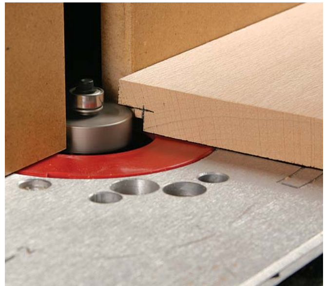
Cut rabbets in passes. Set the fence at the shoulder width and raise the bit incrementally.
