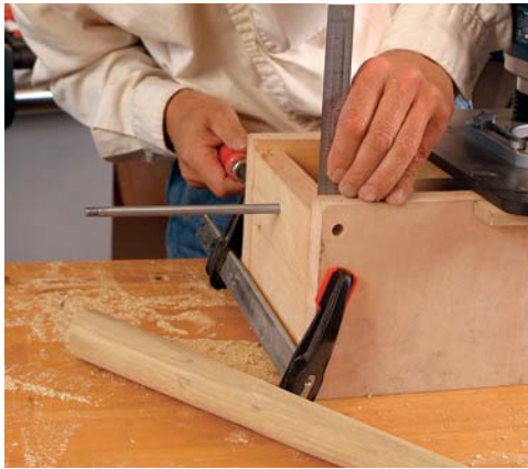
Tapered turnings. Lower the hole at one end of the jig to taper the turned workpiece.
