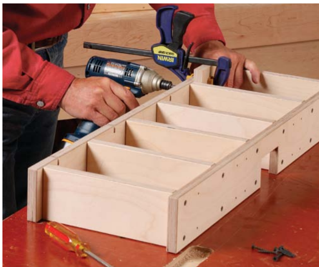
Ribs make the fence rigid. Clamp a plywood spacer next to the rib so that it remains vertical as you screw it in place.
