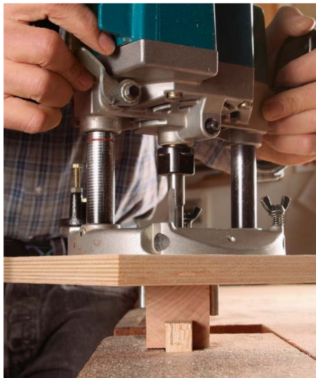
Rotate the router. When the pins touch the sides of the workpiece, the router bit is centered.
