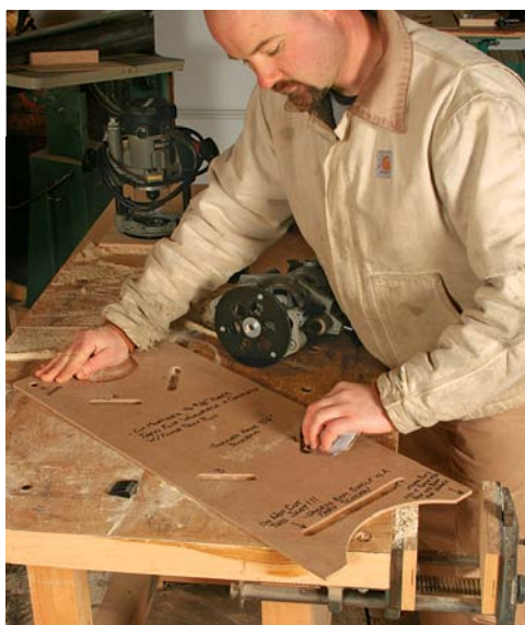
One template, multiple cuts. Paolini designed this template so he could make angled cuts for through-mortises as well as decorative curved cutouts on the ends of a book rack.
