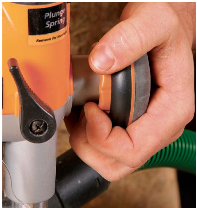
Triton offers a second way to plunge. Pull in the orange lock collar and twist the handle to lower the body on a rack-and-pinion gear. It's a nice way to get precise plunge control.
