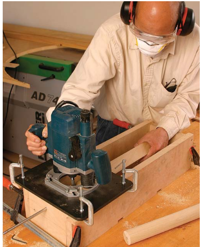
Router-cut turnings. By guiding the router back and forth while turning the workpiece, a square blank gradually becomes a cylinder.
