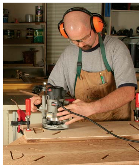
One template, multiple cuts. Paolini designed this template so he could make angled cuts for through-mortises as well as decorative curved cutouts on the ends of a book rack.
