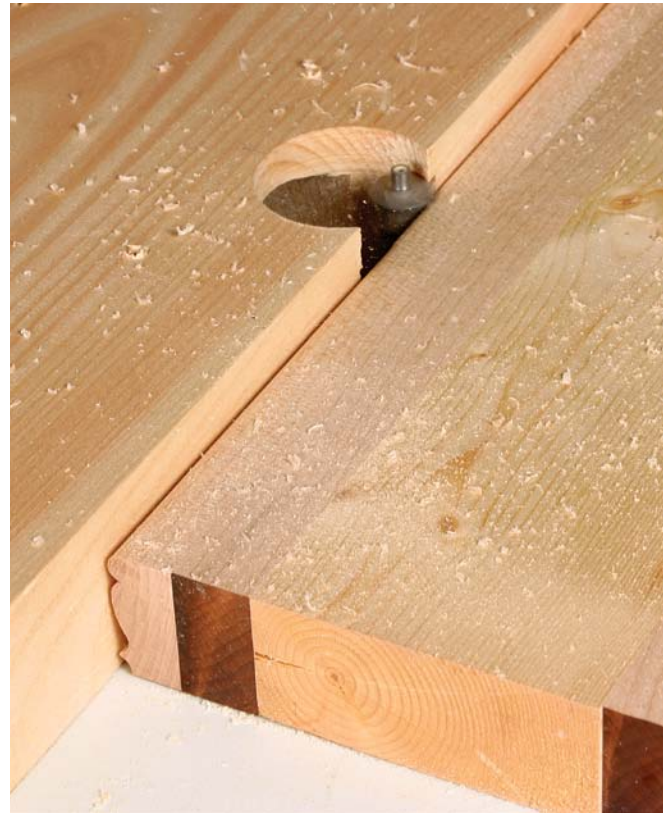
Running smoothly. The offset fence supports the work on the outfeed side and makes for a smooth cut.
