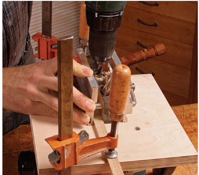
4. Rotate the jig. After drilling the first hole, spin the jig 180° to locate the opposite hole.
