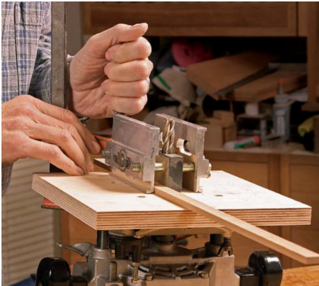
3. Register the jig on a straight strip. Clamp the strip in place and align the jig with it before marking and drilling the first hole.
