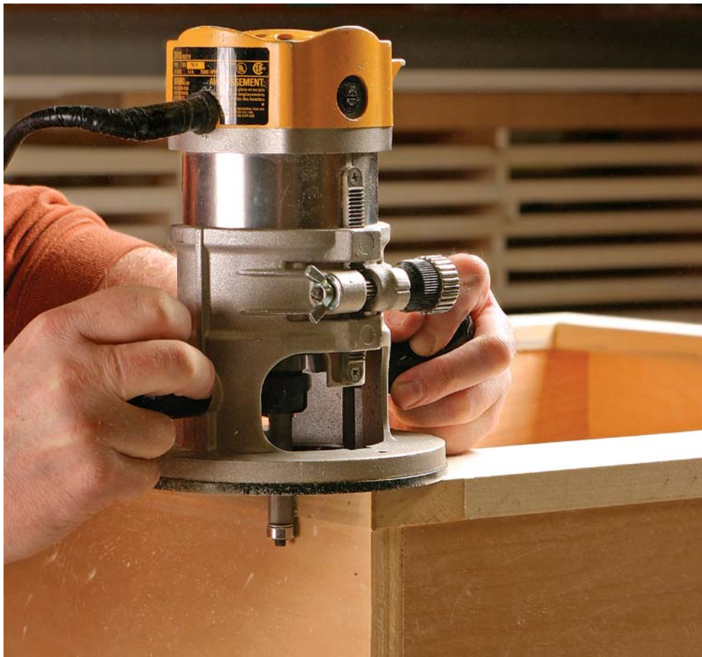
Trim face frames flush to case. The bearing on a flush-trimming bit is the same diameter as the cutter, allowing you to bring a frame flush to a carcass using a handheld router.
