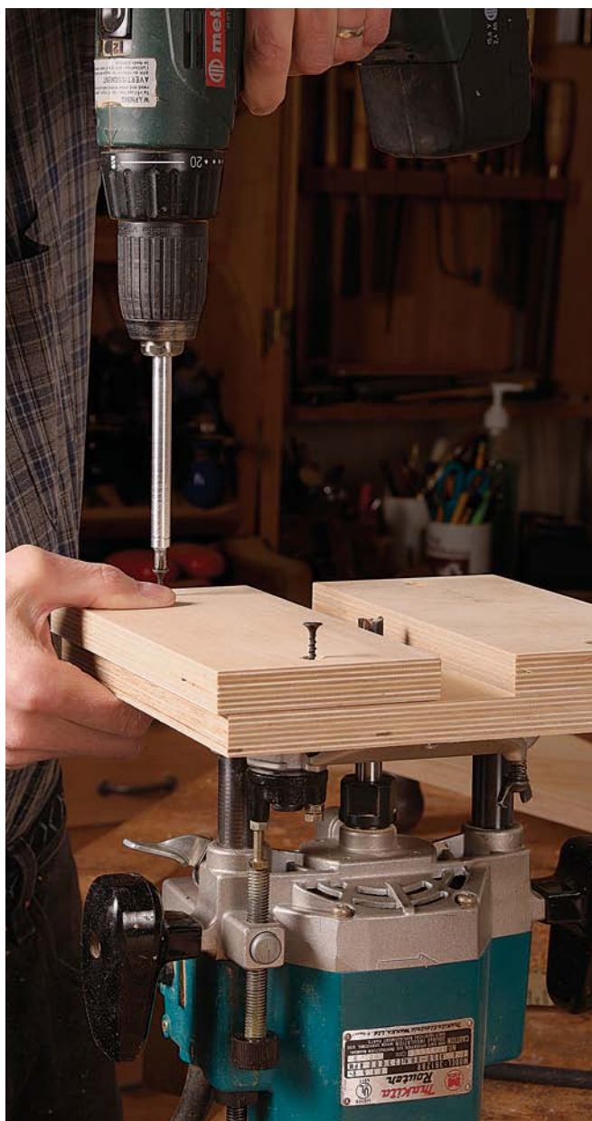
Smaller flush-trimming base. This square base is great for flush-trimming tenons and pegs. It offers support for the router on both sides of the bit.
