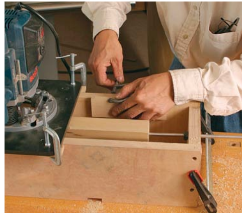
Stopped turnings. Clamp blocks to the side of the jig to leave a square section on the turning.
