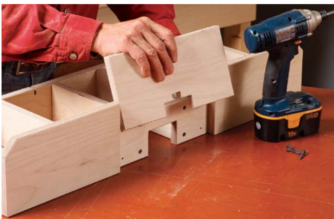
Insert is replaceable. Four screws hold it in place from behind. Make one for each of your most common bits to eliminate tearout. The tall fences on both sides can be replaced, too.
