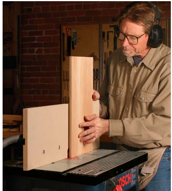
Use a tall auxiliary fence and raise the bit incrementally for a clean cut. Cut the end grain first, then the long grain. This removes any torn-out end grain at the corners.
