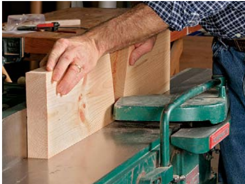
An offset fence in one easy step. Simply joint the infeed edge, stopping at the bit cutout.
