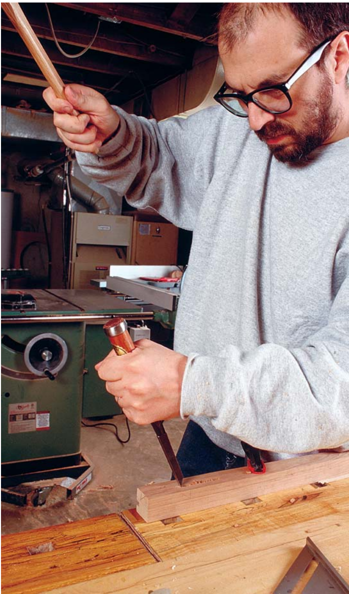
Photo F: Use a mortising chisel and mallet to cut the leg mortises. Begin by making a series of V-cuts, moving outward from the center of the mortise toward the ends.
