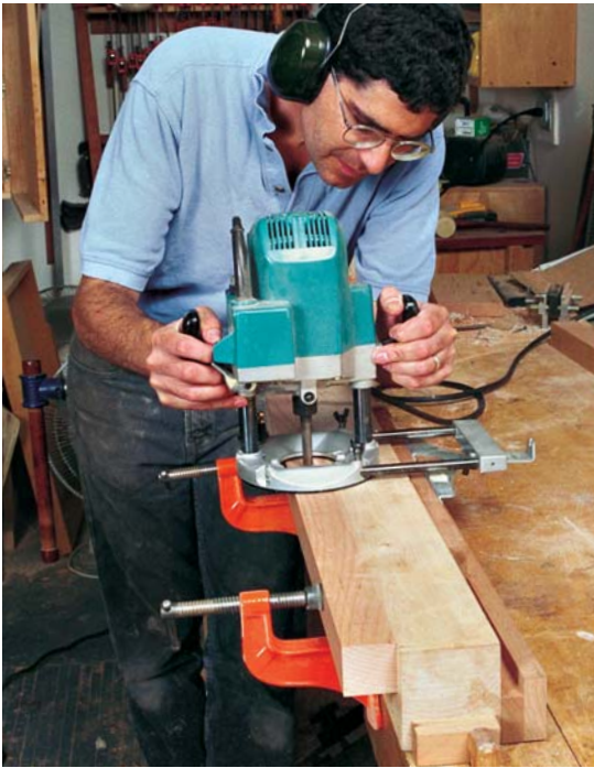
With the post clamped to the mortising block, the router is steady and easy to handle.
