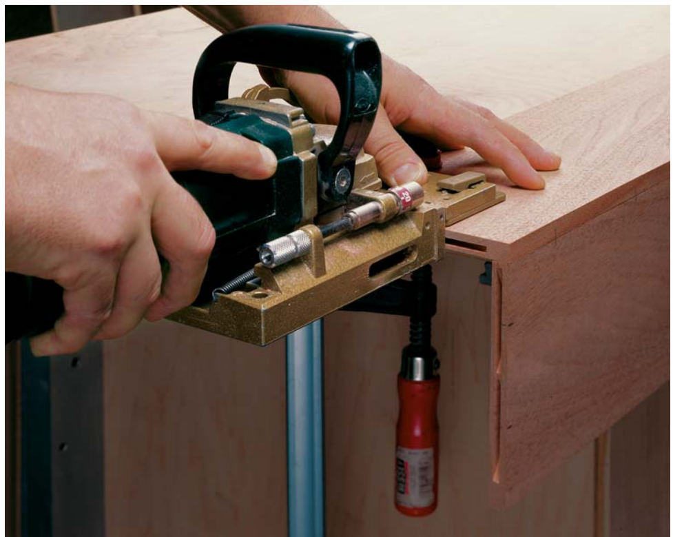
Photo E: Cut four biscuits in the end of each V-shelf, registering the joiner off the shelf backs. Leave the layout lines.
