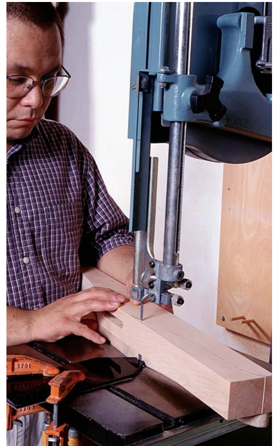
Photo F: The pattern taped to the bottom of the workpiece rubs against the Plexiglas guide, creating identical pieces that can be easily cleaned up using a drum sander.
