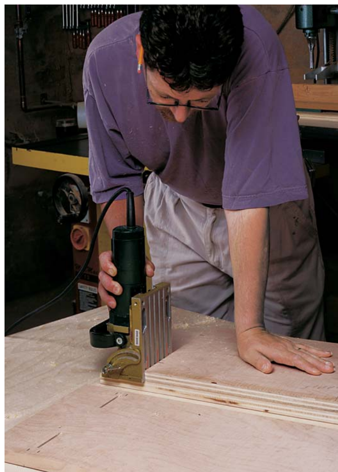
Photo D: Use a shelf as a stop block, aligned on the edge of where the shelf intersects the side, to support the biscuit joiner when cutting the slots in the sides.
