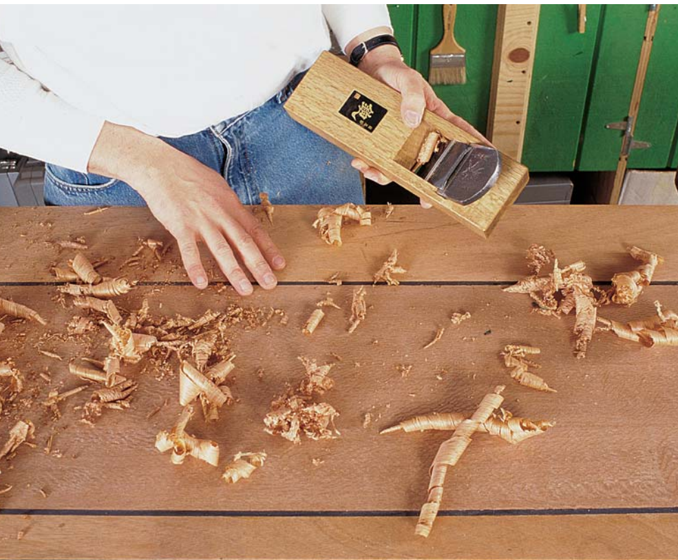
Photo C: Use a smoothing plane to level the frame to the panel. To prevent planing through the thin veneer, use a sharp scraper for your final passes.
