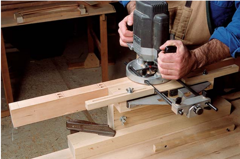
Photo B: The post is aligned in the fixture and clamped to its face. When cutting the mortise, use the edge guide to reference the fixture's back edge; the stops limit the router's travel, thus controlling the length of the mortises.
