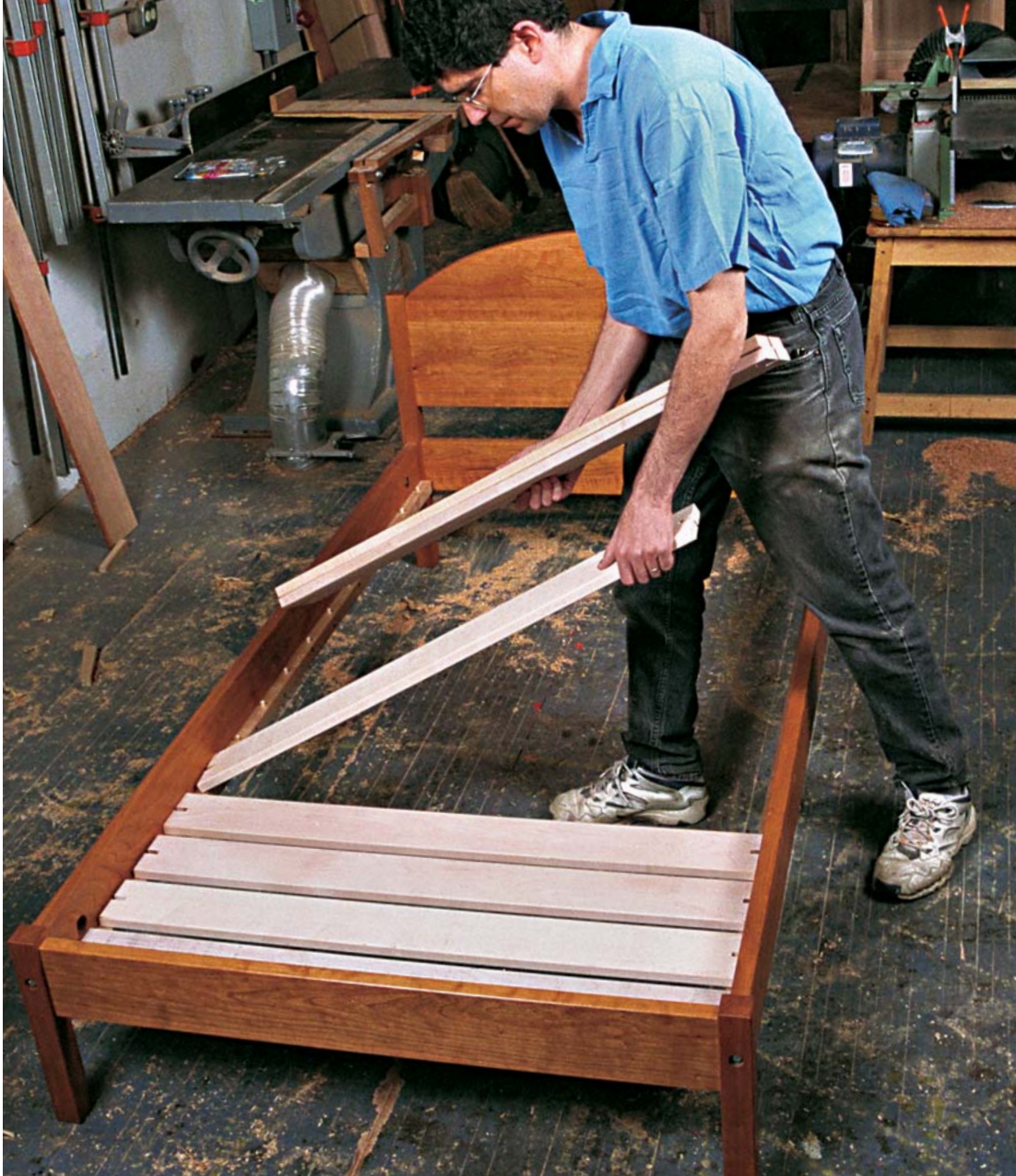
Photo J: Drop the slats into place with the notches around the locating pins in the cleats to complete the bed.
