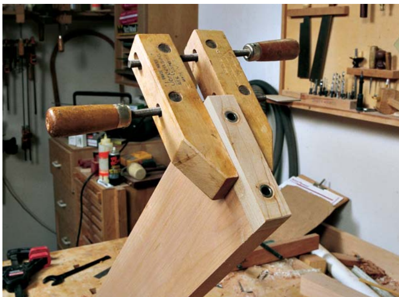
Photo G: To cut the \frac{5}{16} -in.-dowel alignment holes in the side rails, use the same drilling guide you used for the posts.
