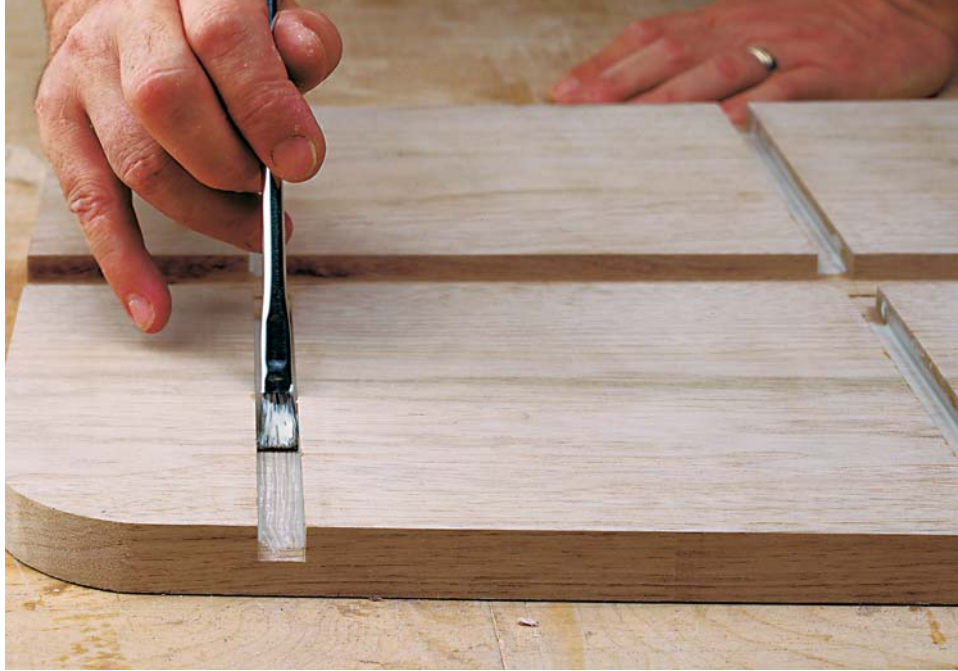
Photo J: An acid brush is small enough to spread glue evenly in the dados of the sides.
