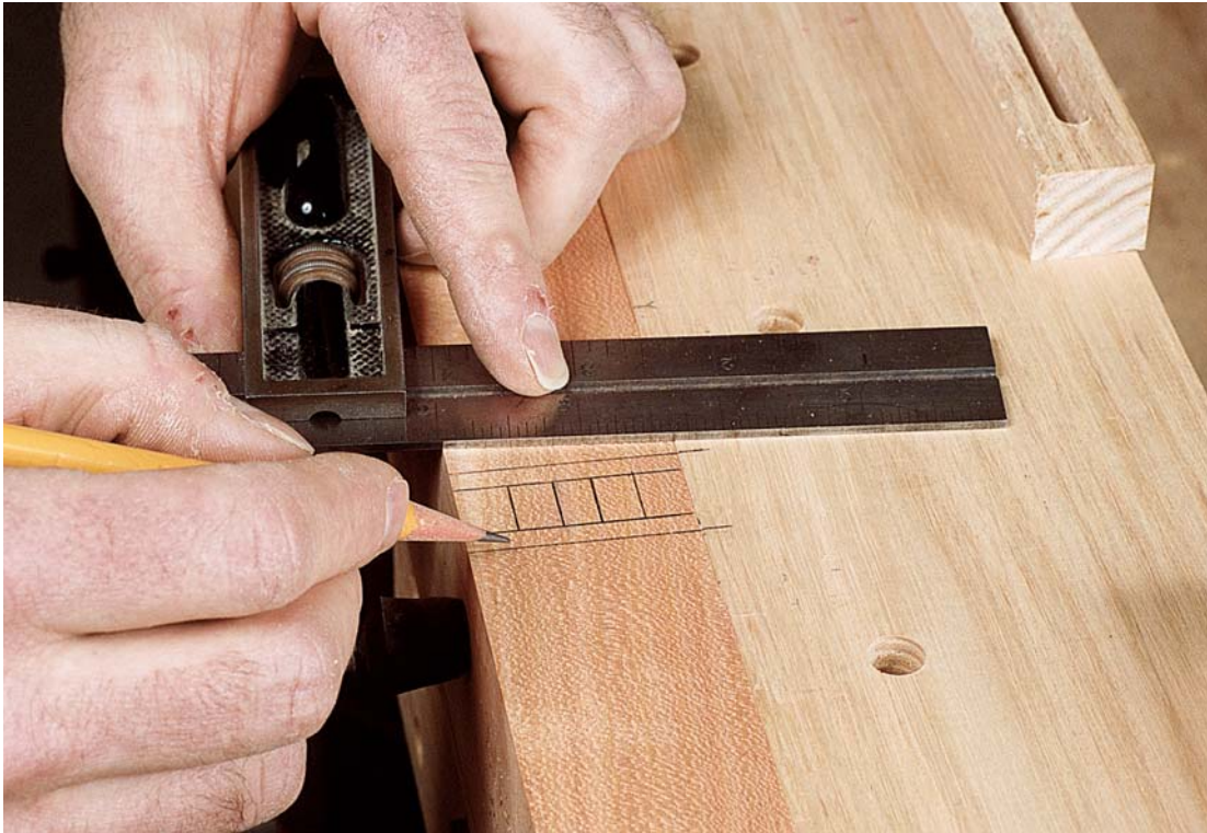
Photo A: Lay out one pair of mortises on a post to help you set up the router, edge guide, and fixture. Extend the lines delineating the rail edges onto the mortising fixture to use when positioning the post for each pair of mortises.
