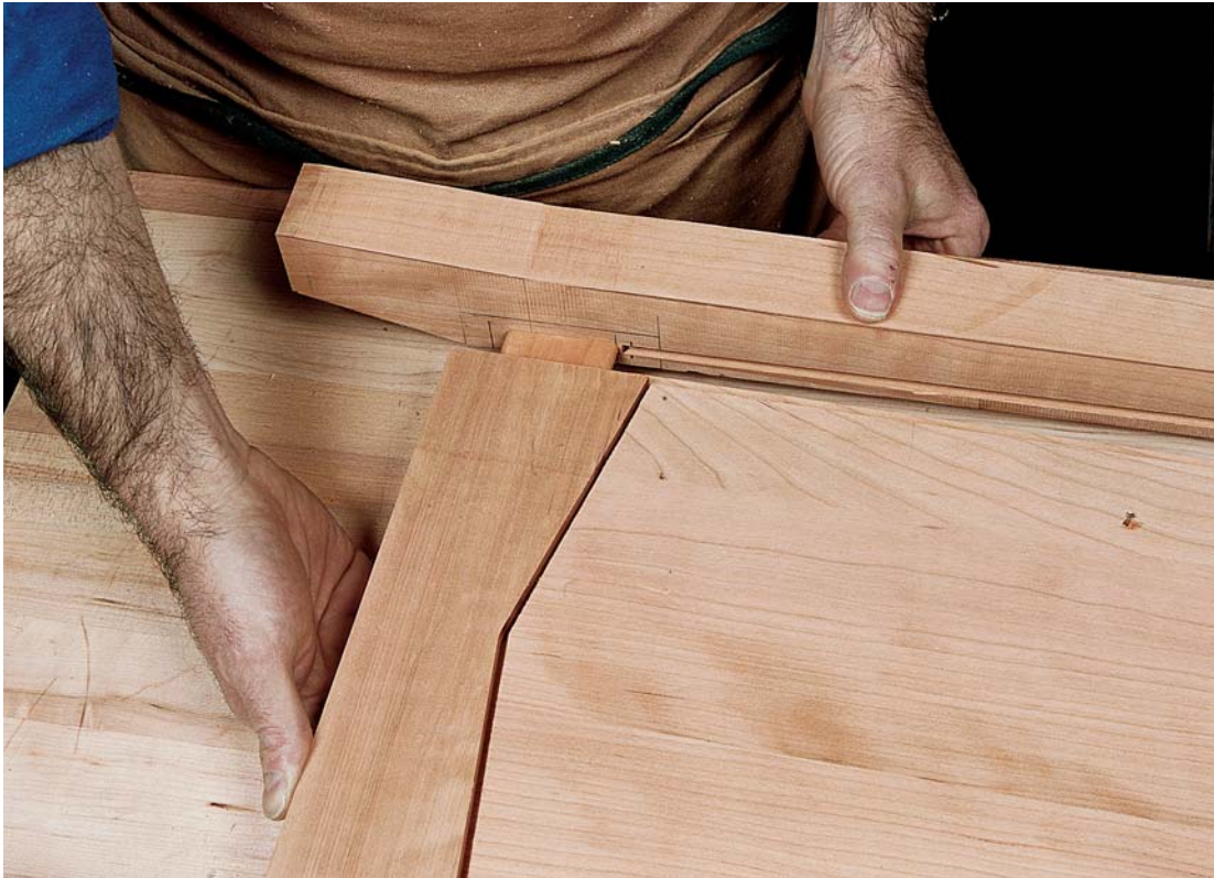
Photo H: Assemble each case side by capturing the panel between the rails and carefully engaging the tenons and panel edge in a post's mortises and panel groove.
