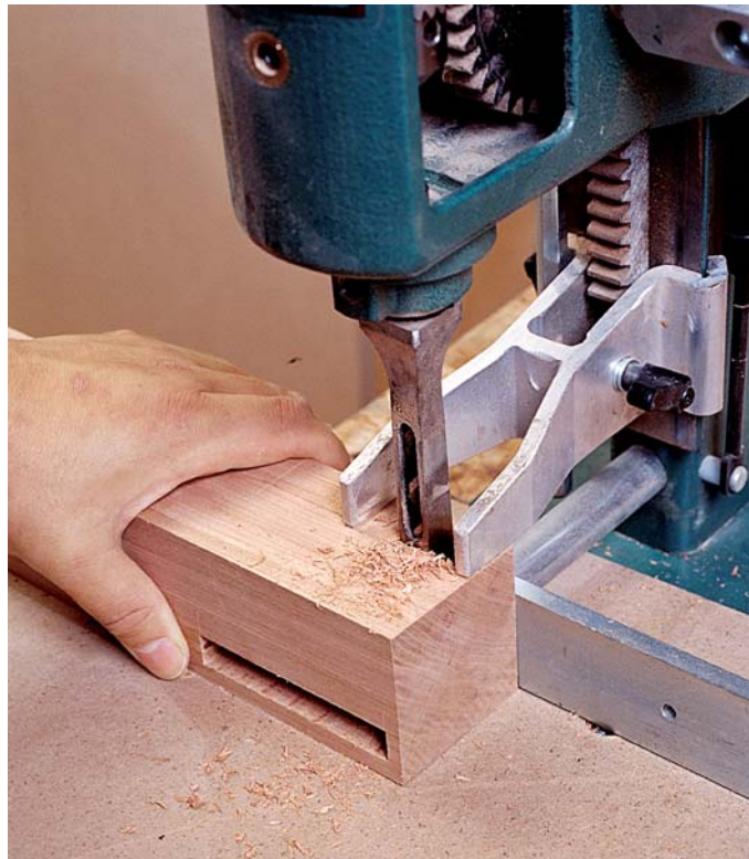
Photo H: Use the mortising machine to mill the mortises.
