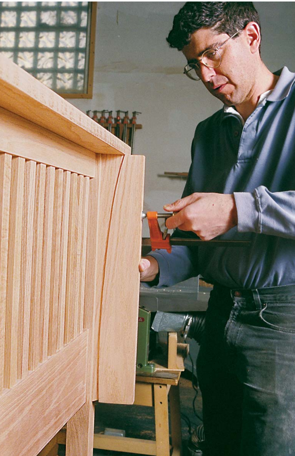
Photo M: Using the cutoff from bandsawing the wing as a caul makes it easy to clamp the wing in place and ensures even pressure.
