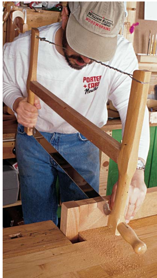
Photo J: After gluing up the long apron and leg assemblies, cut the half-lap notches in all of the aprons.
