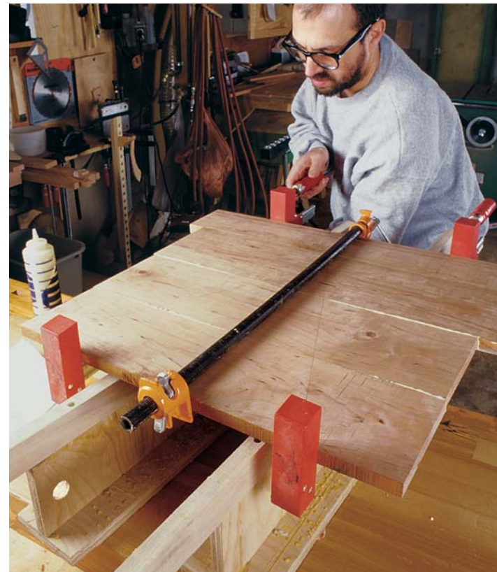
Photo B: Clamping stands allow easy access to the clamps when edge joining boards. The weight of the clamps on the top also helps pull the panel flat.
