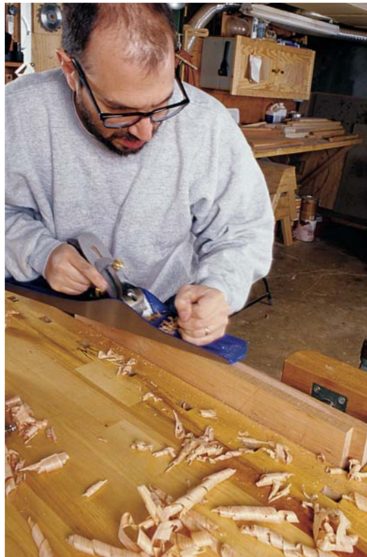
Photo A: To joint boards by hand, align two adjacent edges in the vise and plane them at the same time.
