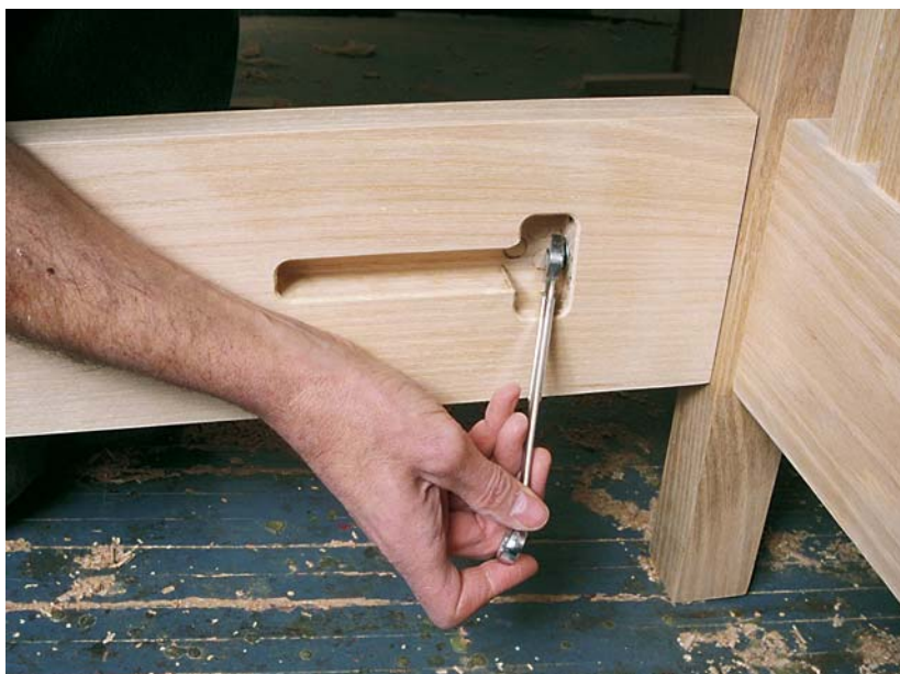
Photo P: Then tighten the bolt with an open-end wrench. The space at the top of the T leaves room to rotate the wrench.
