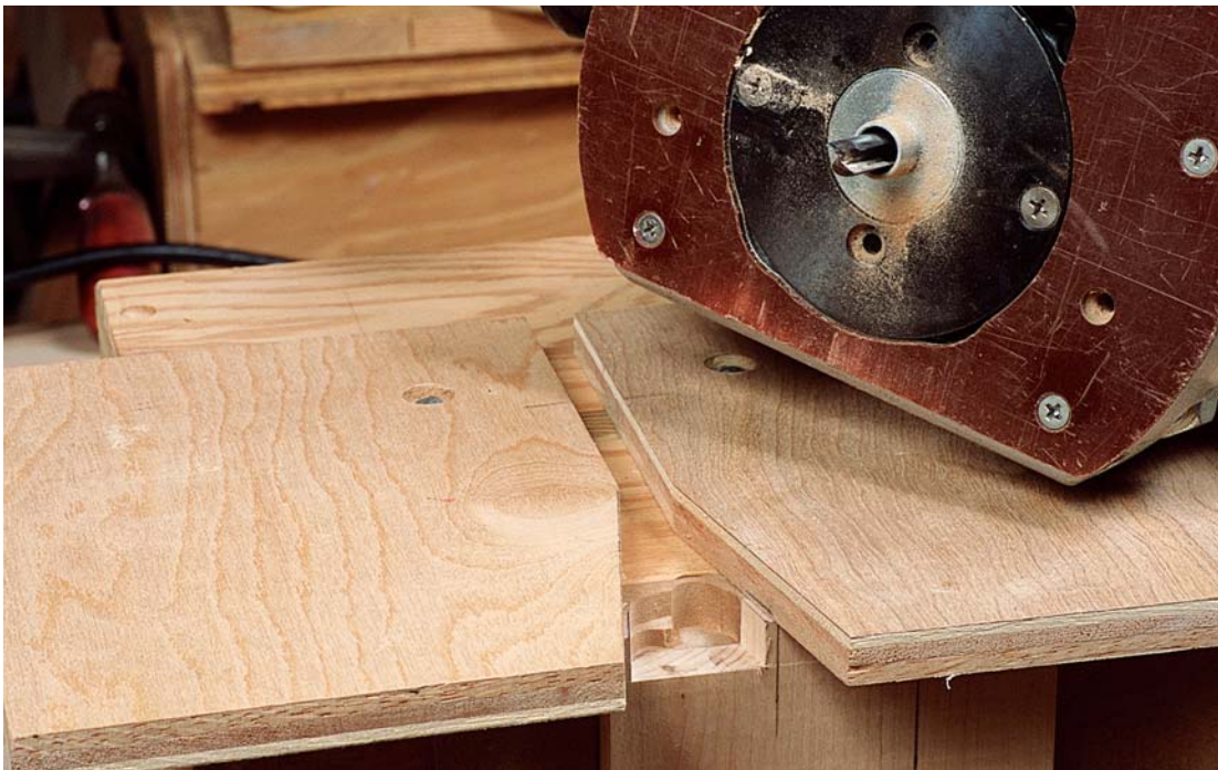
Photo P: The pins on the drawer backs are routed using Burton's shopmade adjustable pin-cutting template.
