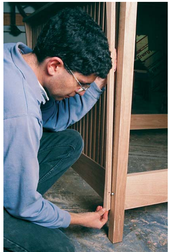
Photo L: A recess in the back of the wing allows room for the bolt to come through the leg. Without it, the bolt will break the wing right off when you tighten it during assembly.
