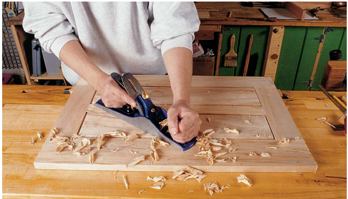
Photo G: Plane the top surface of the drawer bottom to ensure that the panels and frame members are flush.
