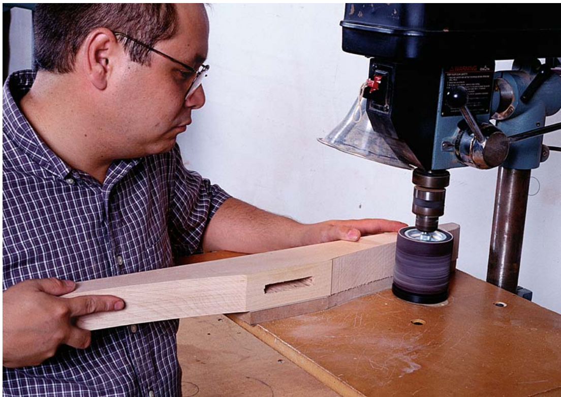
Photo G: The Robo-sander™ has a bottom-mounted bearing that rubs against the pattern, sanding the workpiece to the precise shape.
