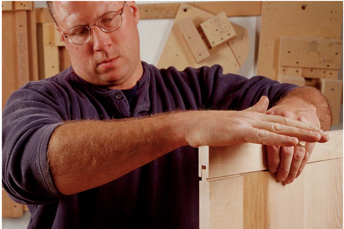
Photo H: The tongue on each end of the pull-out board should fit snugly into the groove on the breadboard end, but not so tightly that you have to pound it in with a hammer.
