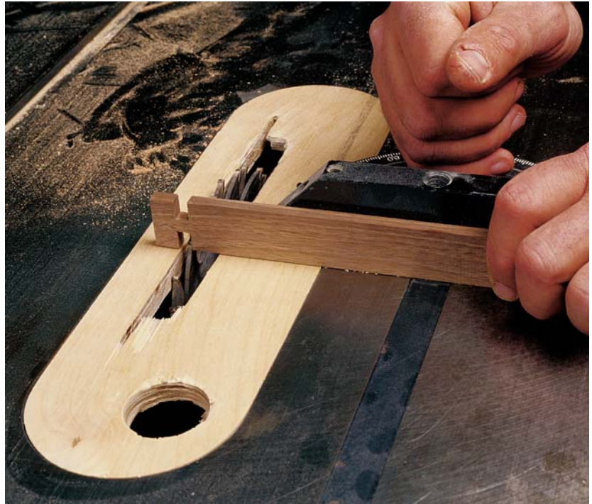
Photo L: To make the tenon on the pull, cut two opposing notches in the pull stock, then crosscut the pull free.
