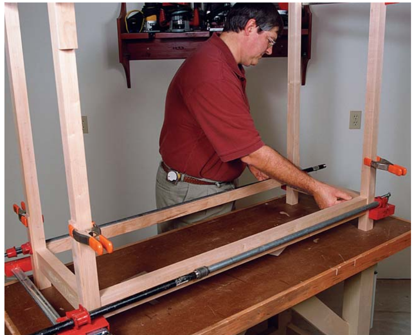
Photo C: A dry run allows you to check the fit of the joints and determine the dimensions for the side, bottom, and back panels. Clamp the sides; then join them to the front and back rails.
