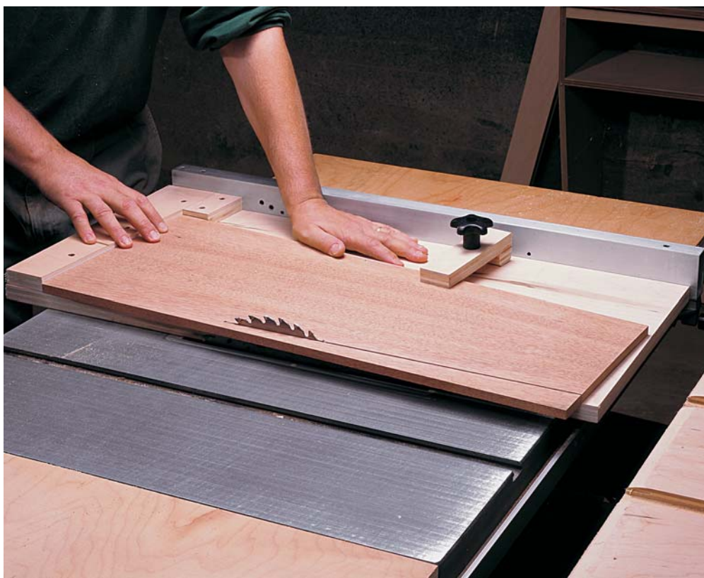
Photo A: A simple taper jig cuts the angle on the side. With the registration block, it also ensures the sides are uniformly wide.
