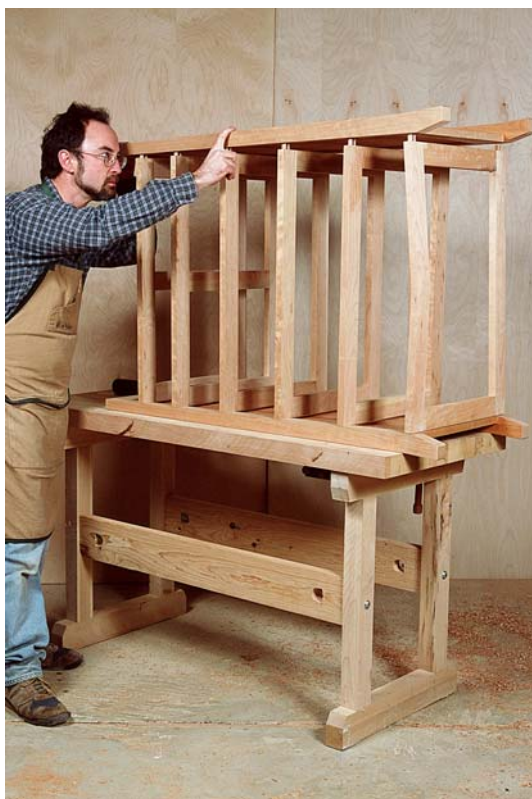
Photo K: Case assembly begins with the side flat on the bench. After joining all the web frames to it, set the second side in place and methodically start all the tenons into their mortises.
