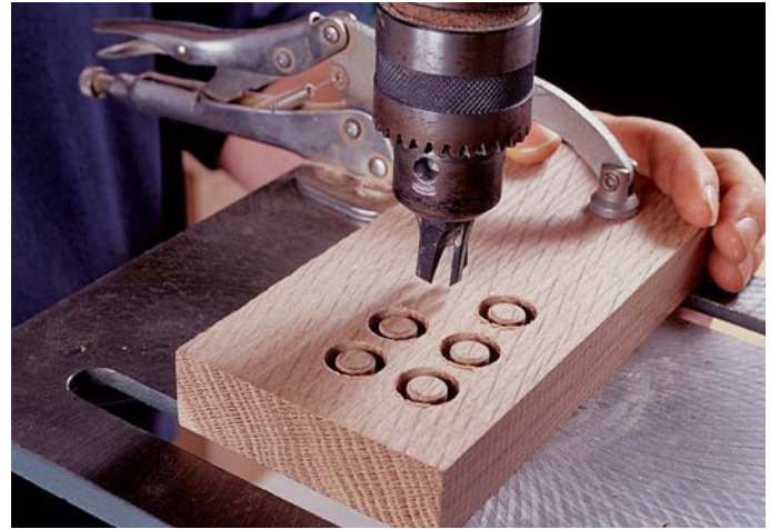
Photo D: If you cut your own plugs, you can match the grain direction and make the plugs almost invisible. Clamp the stock to the drill-press table so the workpiece doesn't spin.
