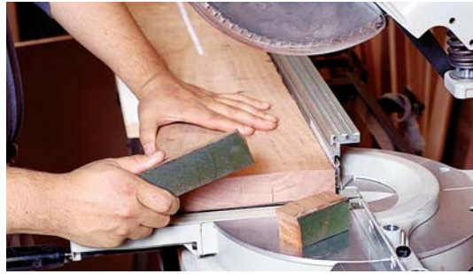
Photo B: Knock the cutoff against the saw table to determine whether it is solid.
