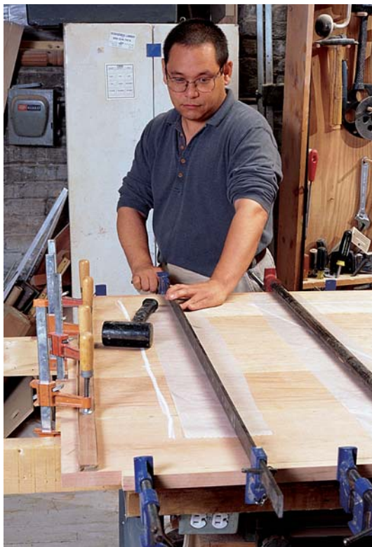
Photo G: When you glue up the tabletop, use clamp blocks to protect the edges, clamp cauls to keep the tabletop even, tape to keep the cauls from sticking, and waxed paper to keep the metal clamps from leaving oxidation marks on the boards.
