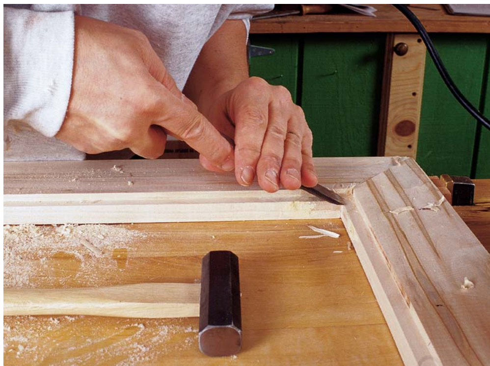
Photo C: Clean up the bottom of the rabbet corner with a chisel.
