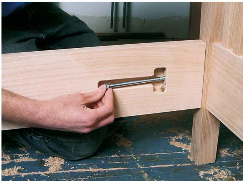
Photo O: To assemble the bed with T-slots, first insert the bolt and washer into the hole and push them forward.
