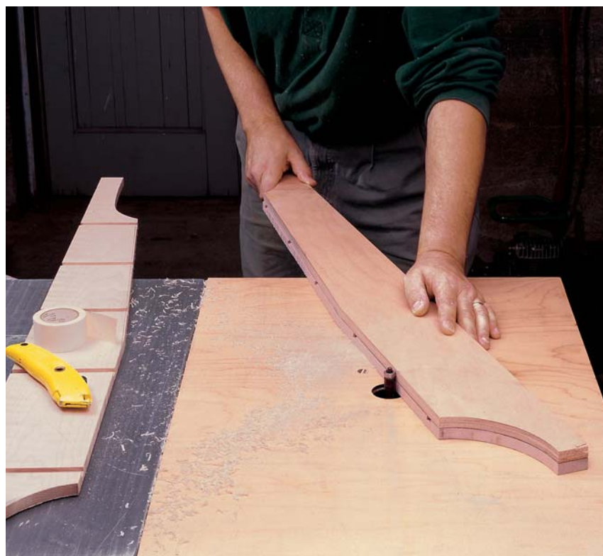
Photo D: The plywood pattern helps you rout a smooth near-perfect edge on the profile of the sides.
