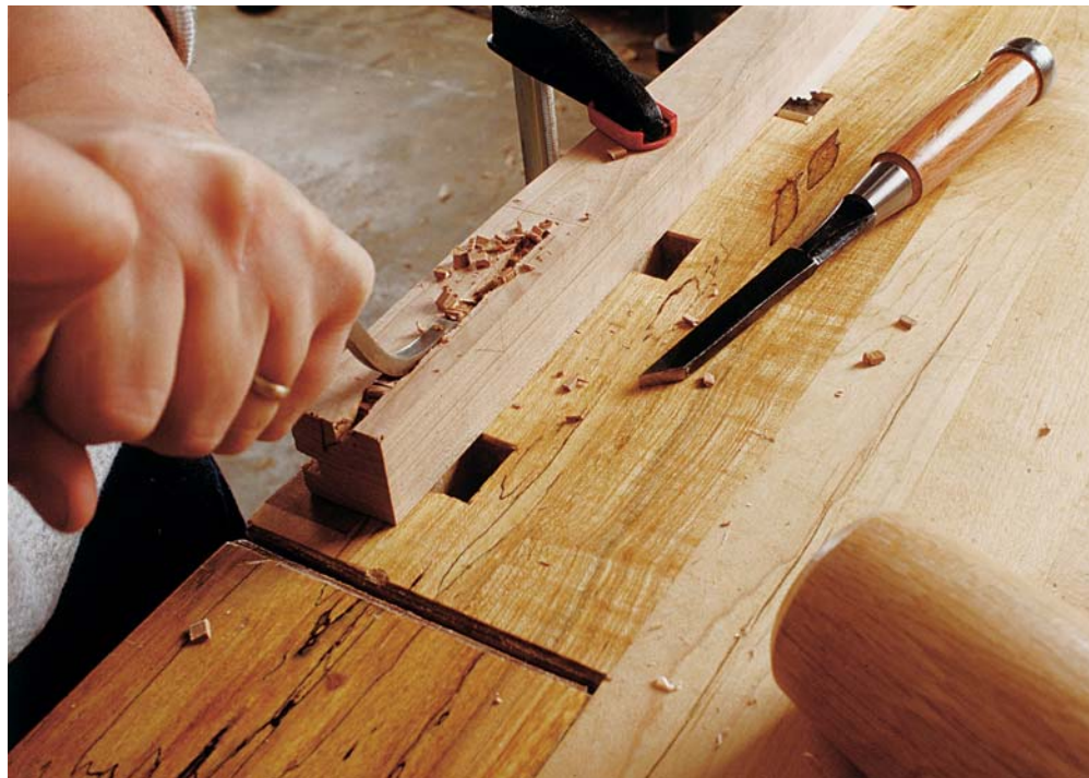
Photo G: Even up the depth of the mortise with a swan-neck chisel.
