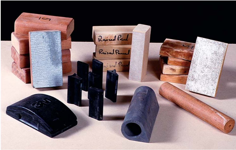
Photo K: Having a variety of shopmade and commercial sanding blocks in different shapes and sizes is useful when hand-sanding.
