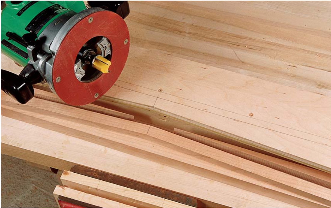
Photo I: The V-shape of the bottom rail is routed into a thick workpiece. Secure the work and the template, which is screwed to a fence, in a vise for routing. The rail's bottom edge is then cut to shape on the bandsaw.
