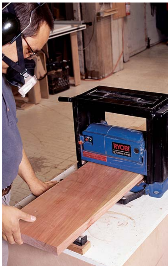
Photo E: Use the same setting to plane all of the boards so that you will achieve a uniform thickness.
