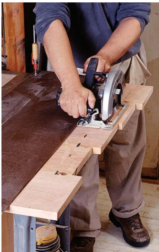
Photo N: The tabletop panel faces down when you crosscut it using a circular saw and straightedge.
