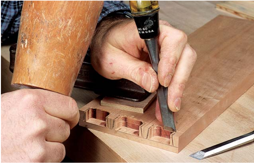
Photo O: The final paring is done with a pair of custom-ground chisels: one for the left, one for the right.
