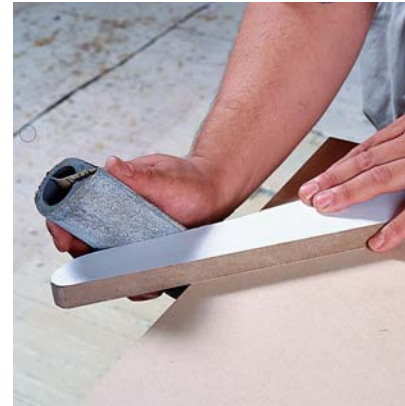
Photo E: Leave the line when cutting out the waste. Then use a sanding block to sand down to the line, fairing the curve as you go.
