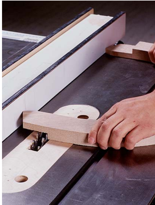
Photo F: Run the harp against the fence and cut the top shoulders square.
