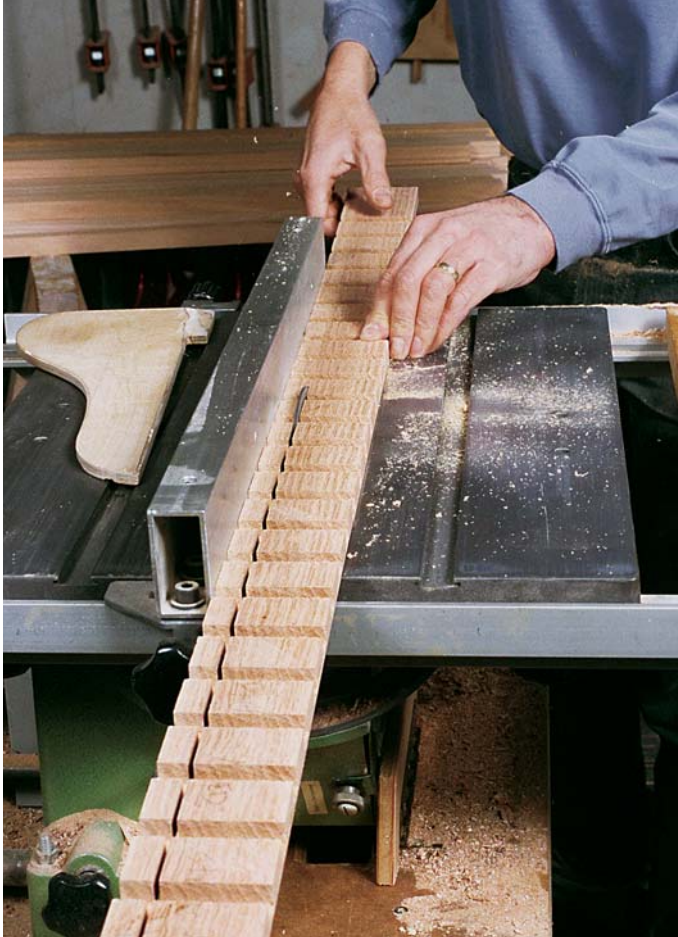
Photo B: Use a push stick to guide the thin and fragile strips past the blade, and use an outfeed roller (not shown in photo) if you don't have a helper.
