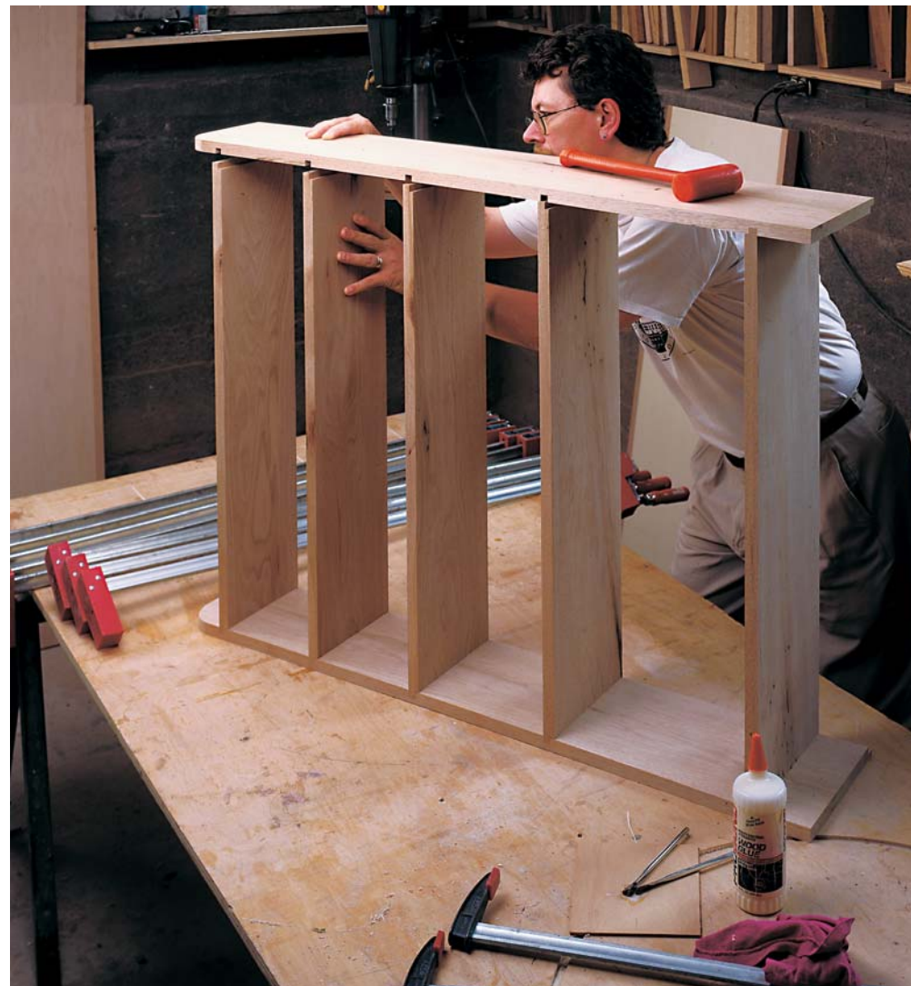
Photo K: Glue-up can be a hectic time, so make sure you have all the clamps and pieces ready to go and proceed in a quick but orderly fashion.
