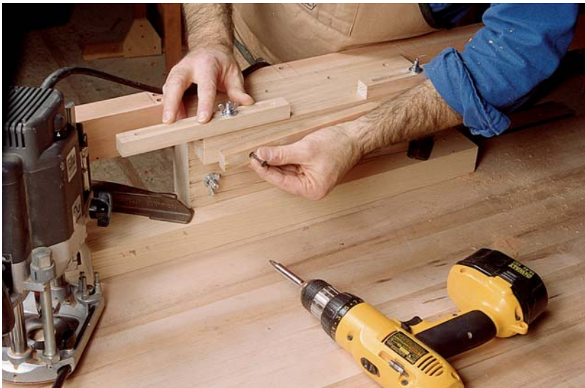
Photo C: Screw a spacer to the fixture's back edge to shift the position of the bit \frac{5}{8} in. closer to the fixture. This allows you to rout both mortises in a pair with one router/edge-guide setup.
