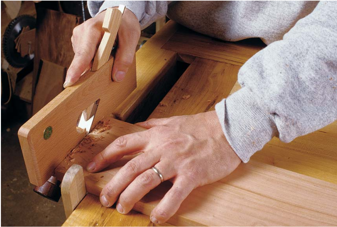
Photo J: Planing the tenon shoulders with a rabbet plane allows fine-tuning of the tenon thickness for a perfect fit in the mortise.
