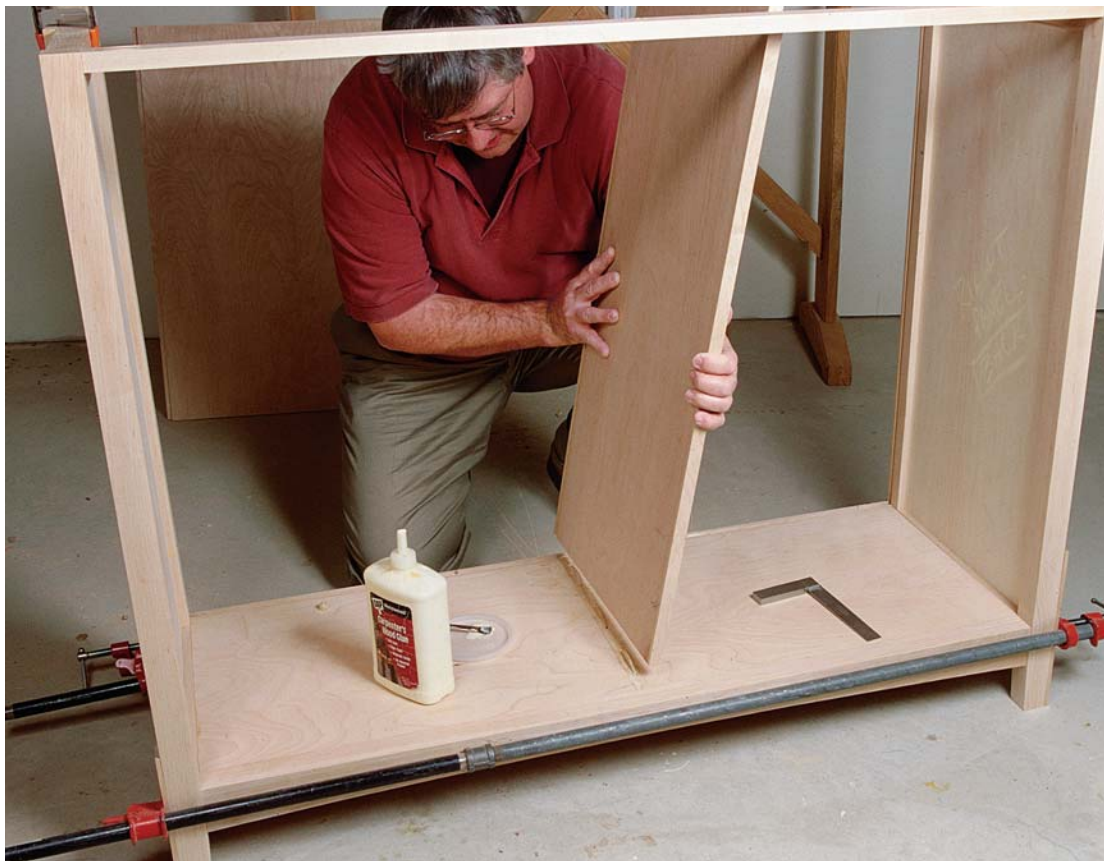
Photo F: Glue biscuits in the slots in the case bottom and maneuver the partition into place, nestled under the front rail.
