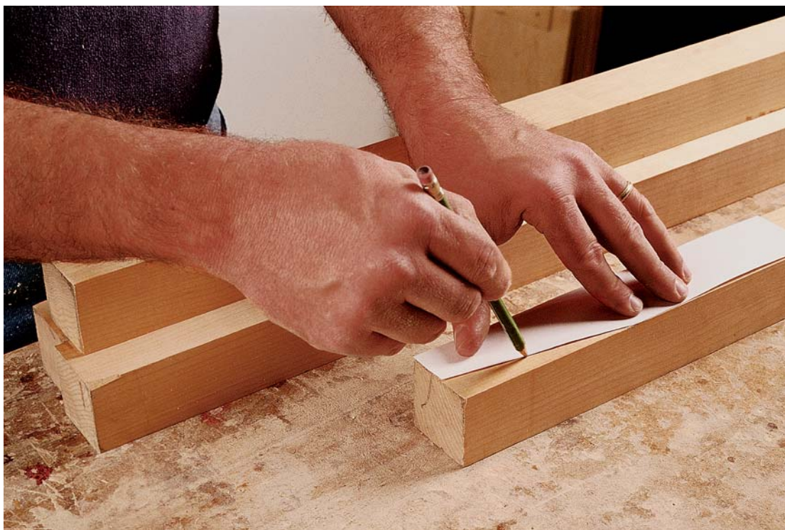
Photo A: A stiff pattern ensures that the taper on each leg will be uniform.
