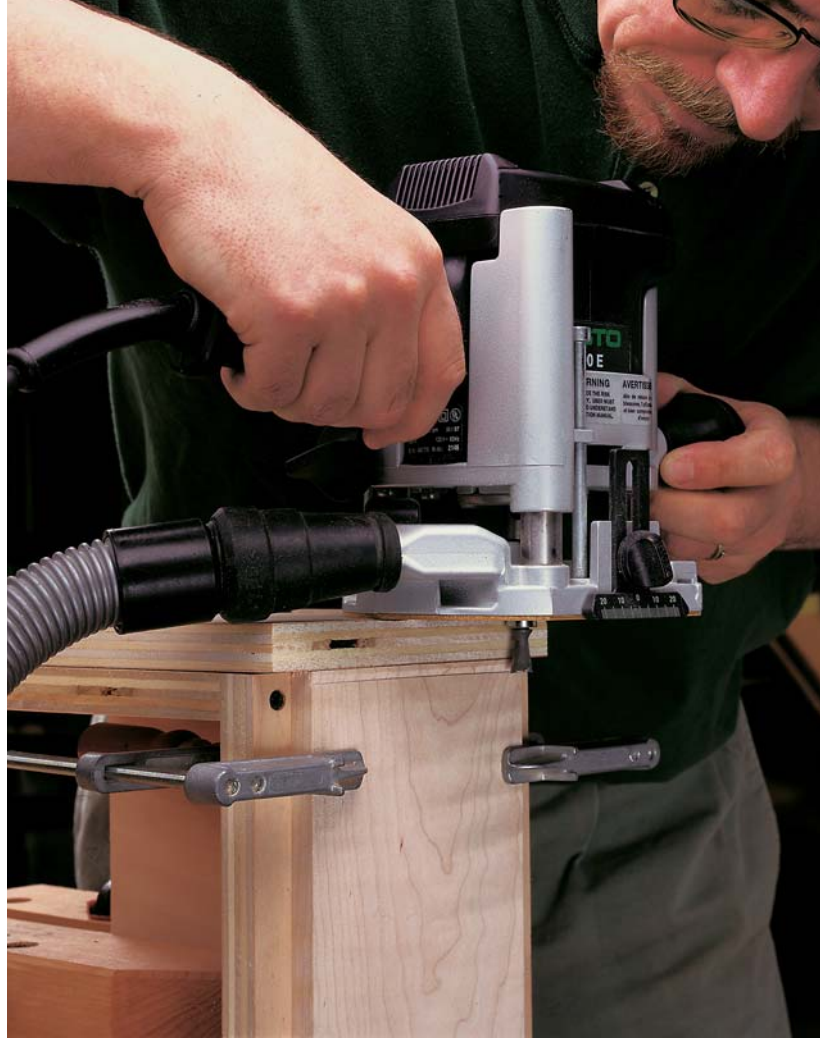
Photo B: The jig for routing tails holds the shelf vertical and cuts one side of the tail at a time. It is accurate, if a little fussy to set up.
