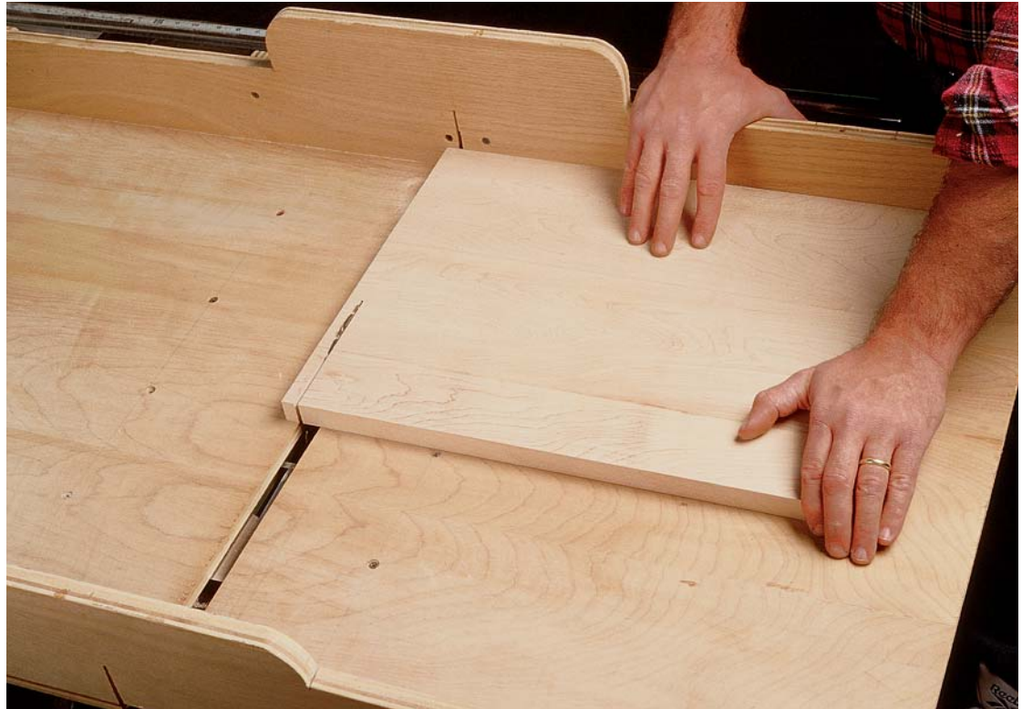
Photo D: A tablesaw crosscut sled allows you to crosscut wide panels squarely.
