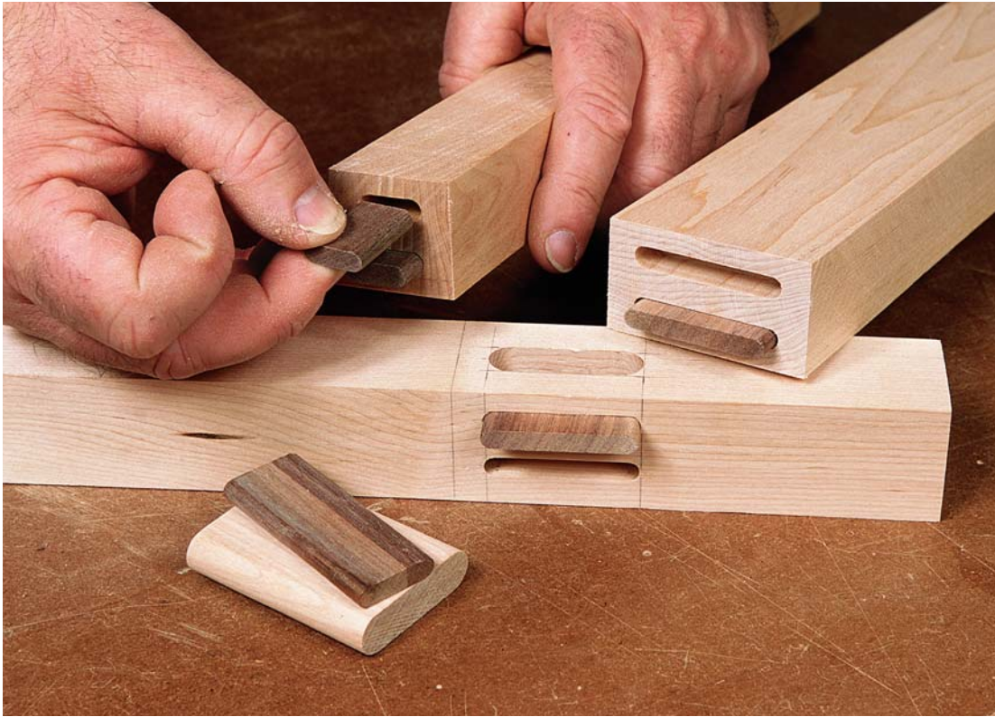
Photo B: A loose tenon is easy to fit snugly in its mortise. Prepare a long strip to the proper thickness and width, bullnose the edges on the router table, and crosscut individual slips.
