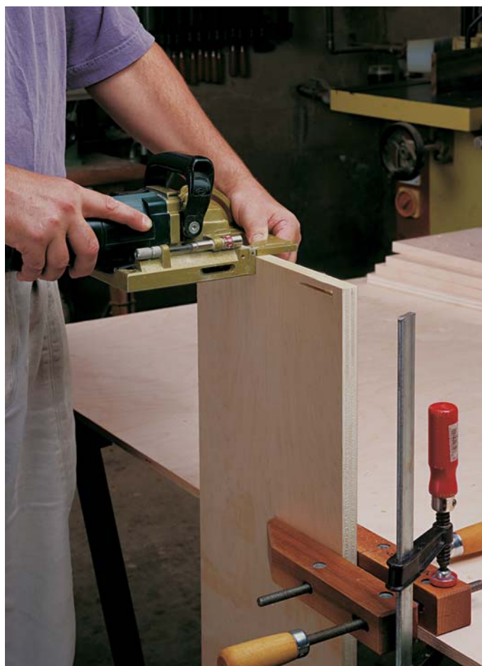
Photo C: The biscuit slots in the top are cut on the edge but at a right angle. This is a difficult kind of cut to keep stable, so go slowly and carefully.
