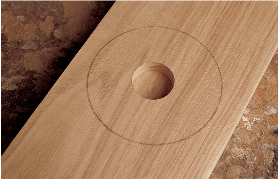
Photo I: To establish the perimeter and depth of the pull recess, draw its outer diameter, then drill a flat-bottomed hole in the center.
