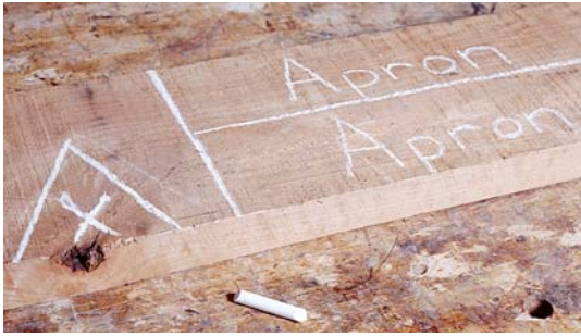
Photo A: Mark up the boards for the rough cut.
