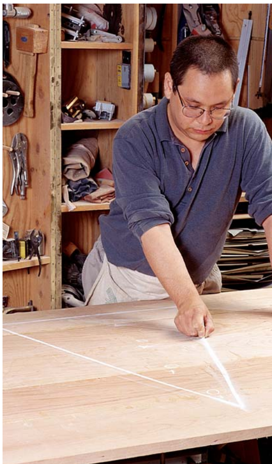
Photo F: Drawing a triangle across the tabletop boards helps you line them up the way you want them.
