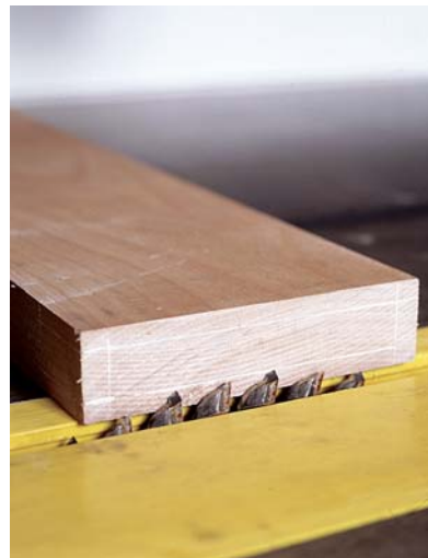
Photo J: Adjust the blade height to match the knife mark on the end grain of the apron.
