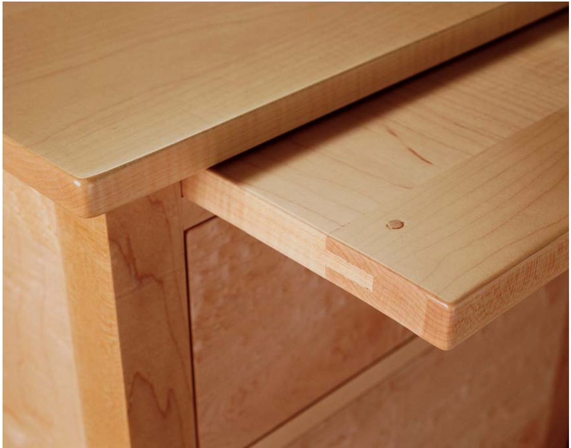
Photo F: The front edge of the pull-out board is feathered back with a sander to maintain a tight fit at the front while allowing for cross-grain expansion and contraction of the board inside the case.
