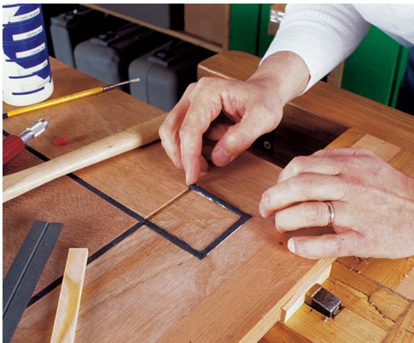
Photo G: Apply the inlay strips into the groove, fitting and gluing one piece at a time to ensure tight butt joints.
