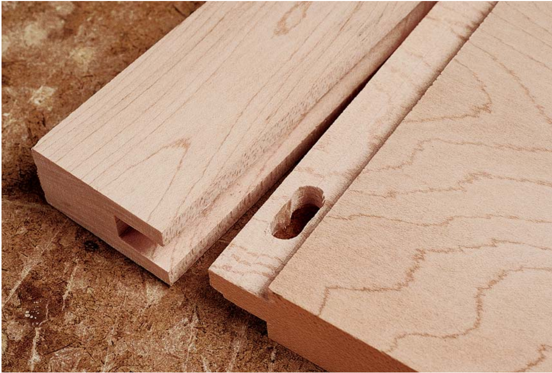
Photo I: Elongated holes in the pull-out board tongue allow the board to expand and contract around the pegs without splitting.
