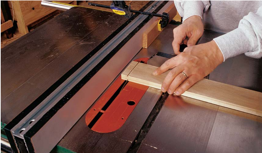
Photo E: The first step in cutting the tenon on the drawer bottom's center frame member is to saw the shoulders.
