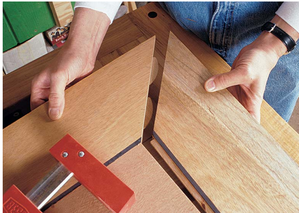
Photo B: Dry-assemble all of the top pieces together before glue-up to make sure they fit tightly.
