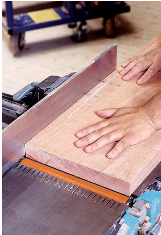
Photo D: Before you rip boards using a table saw, you must face-joint them to minimize the risk of kickback.
