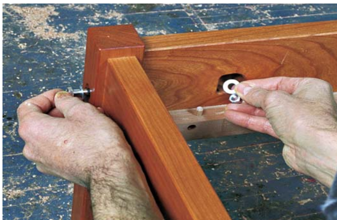
Photo H: To put the bed bolt joints together, insert a bolt with washer from the outside of the bed, until it just reaches into the nut recess. Then place the washer and nut over the end of the bolt, and start turning.
