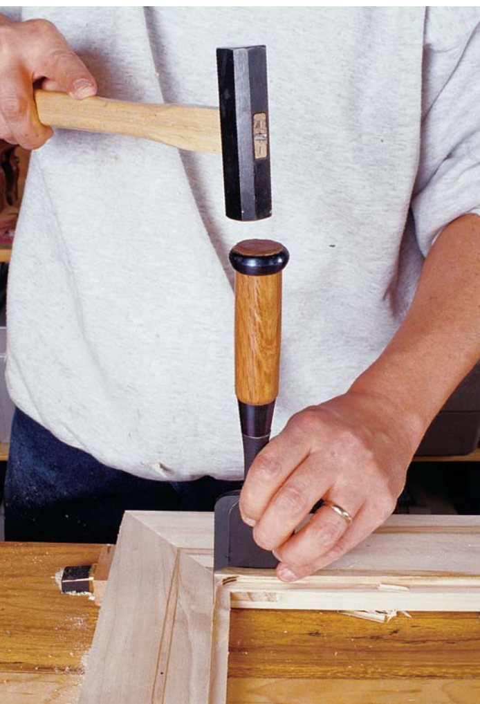
Photo B: The first step in squaring up the corners of the rabbet is to cut the wall using a wide chisel.
