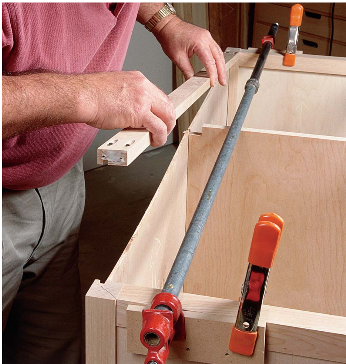
Photo G: Mount the top back rail as soon as the back panels are seated. Get a corner of one panel started in the rail's panel groove, and lower the rail into place.
