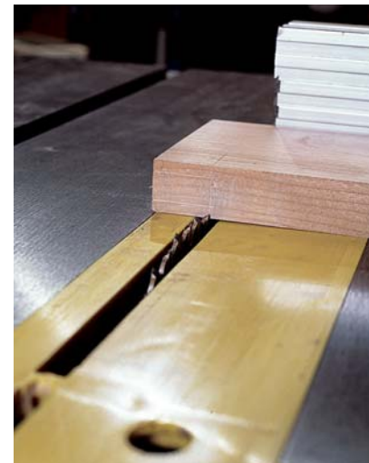
Photo K: The apron piece is positioned so that the edge of the blade meets the mark you made with the knife.
