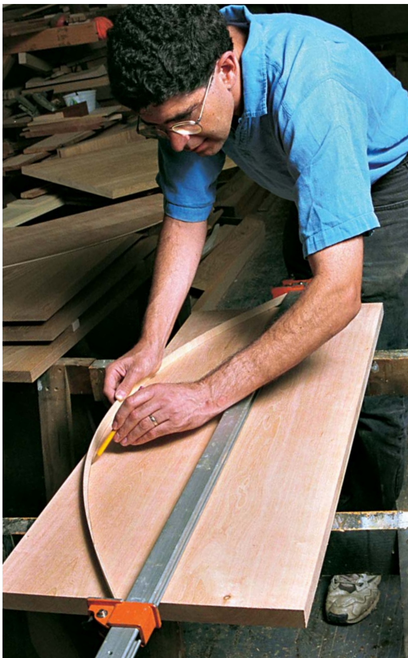
Photo C: Springing an evenly thin piece of wood into a gentle curve is an easy way to lay out the top of the headboard. You can loosen or tighten the clamp to fine-tune the shape.
