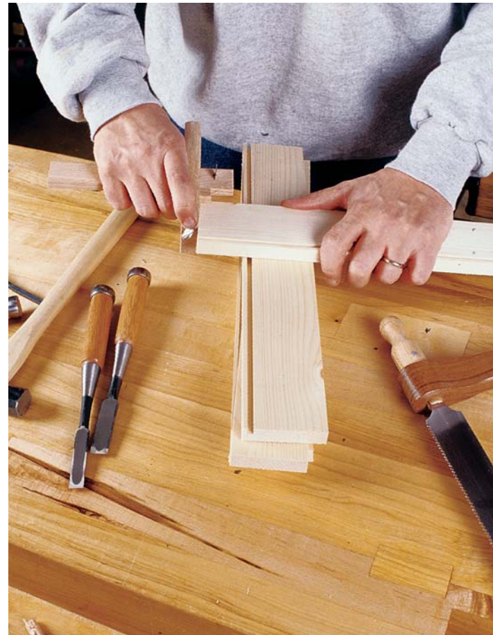
Photo K: Use a marking gauge set to the thickness of the drawer stock to establish the baseline for the pins and tails.
