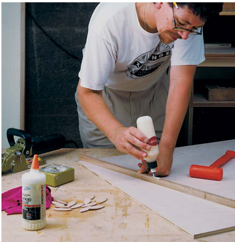
Photo 1: Use biscuits to align the solid butternut strip on the top of the back.
