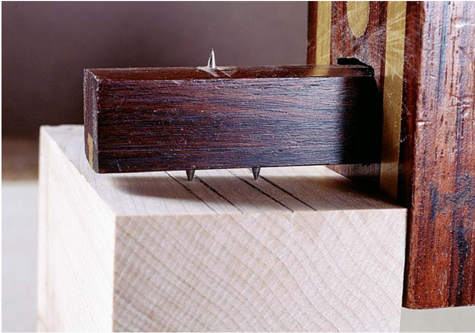
Photo A: It is important to center the mortises on the feet and cleats. Using a piece of scrap the width of the workpieces, mark from both edges, then reset the marking gauge so it splits the resulting lines. Repeat until the lines from the marking gauge overlay when marked from both edges.
