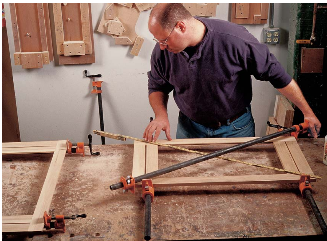
Photo G: To pull a freshly glued assembly into square, squeeze a clamp across opposite corners until opposing diagonal measurements match.
