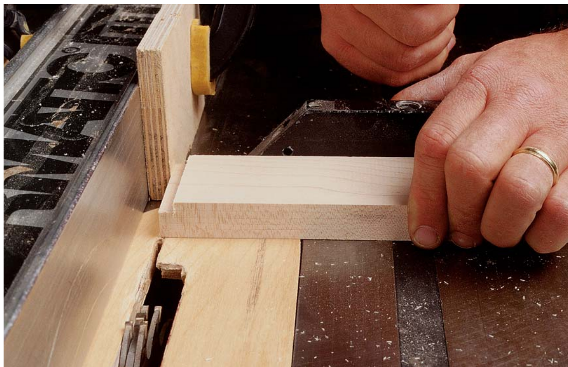
Photo B: When cutting tenons on a tablesaw, use a stop block to prevent having to bury the dado head in an auxiliary fence.
