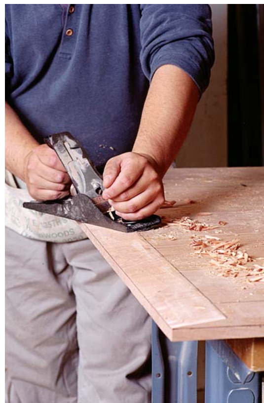
Photo O: If you use a jack plane to cut the bevel, plane the table ends first so any breakout at the end of the cut will be planed off when you bevel the sides.
