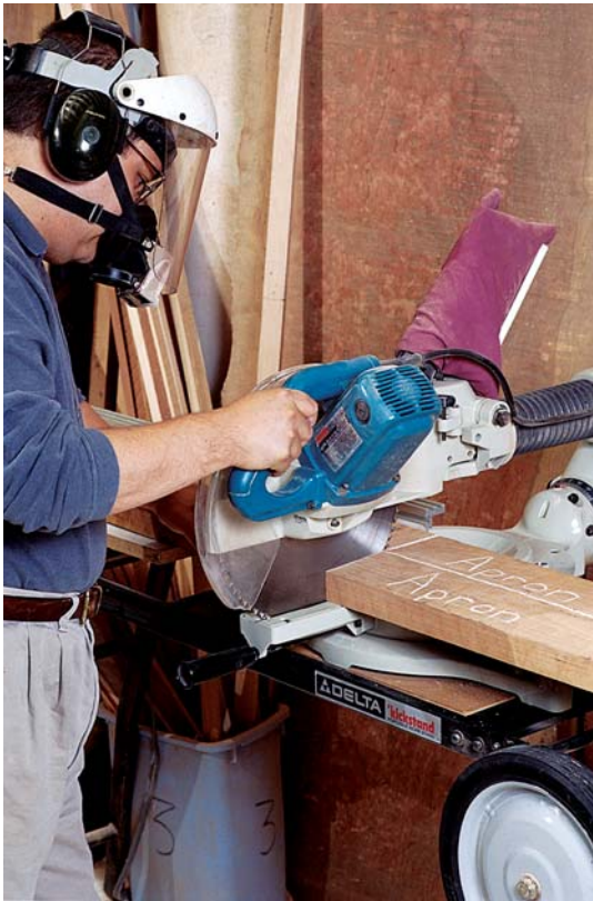
Photo C: Crosscut lumber using a sliding compound miter saw.
