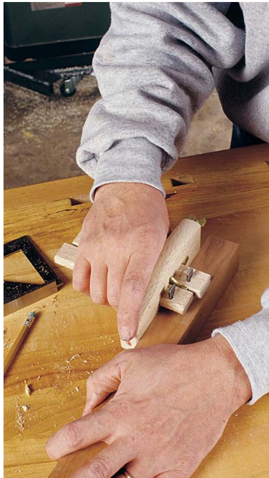
Photo E: Using a mortising gauge is a fast and accurate way to mark out the leg mortises.
