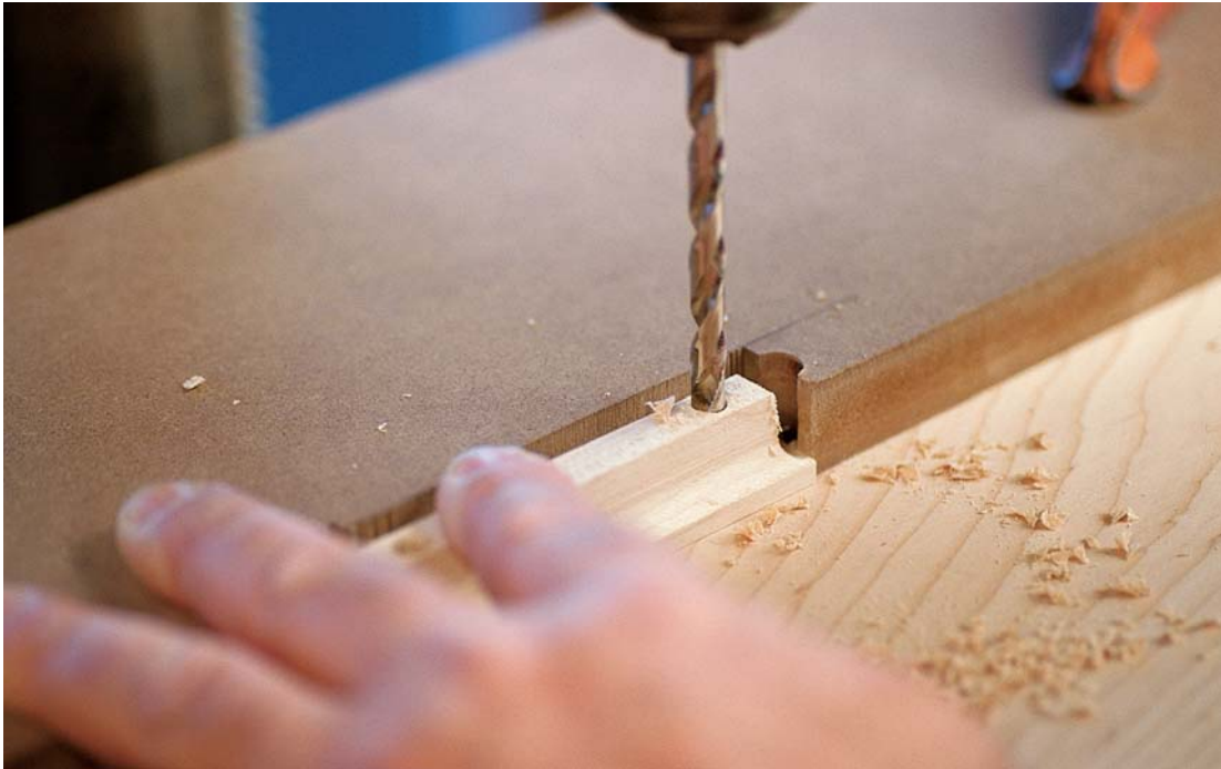
Photo J: Drill dowel holes in the back of each pull. A simple fixture clamped to the drill-press table ensures the holes are located consistently.
