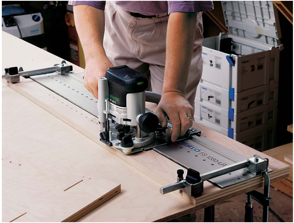
Photo E: The Festo boring jig makes routing accurate holes in the sides quick and easy.
