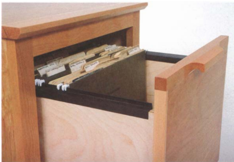
PHOTO F: Plastic file rails slip tightly over the drawer sides to carry hanging file folders. No nails or screws are required.
