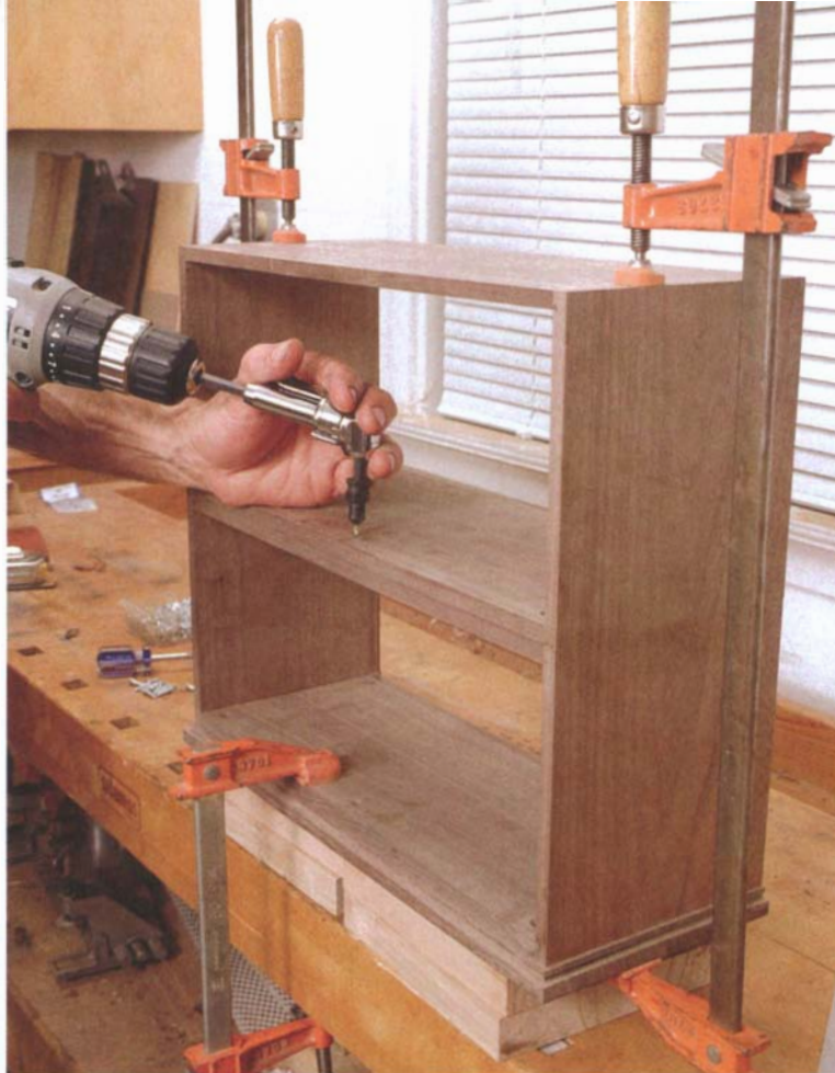
PHOTO F: Drill for the screw holes using a combination pilot/countersink bit. Afterward, enlarge the hole in the countersunk piece to allow the screw to pull the modules tightly together.
