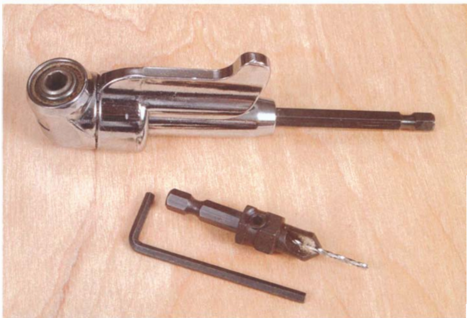
PHOTO G: A right-angle drill adapter is an inexpensive alternative to a right-angle drill. This particular adapter accepts hex shanks. Other types incorporate adjustable chucks.
