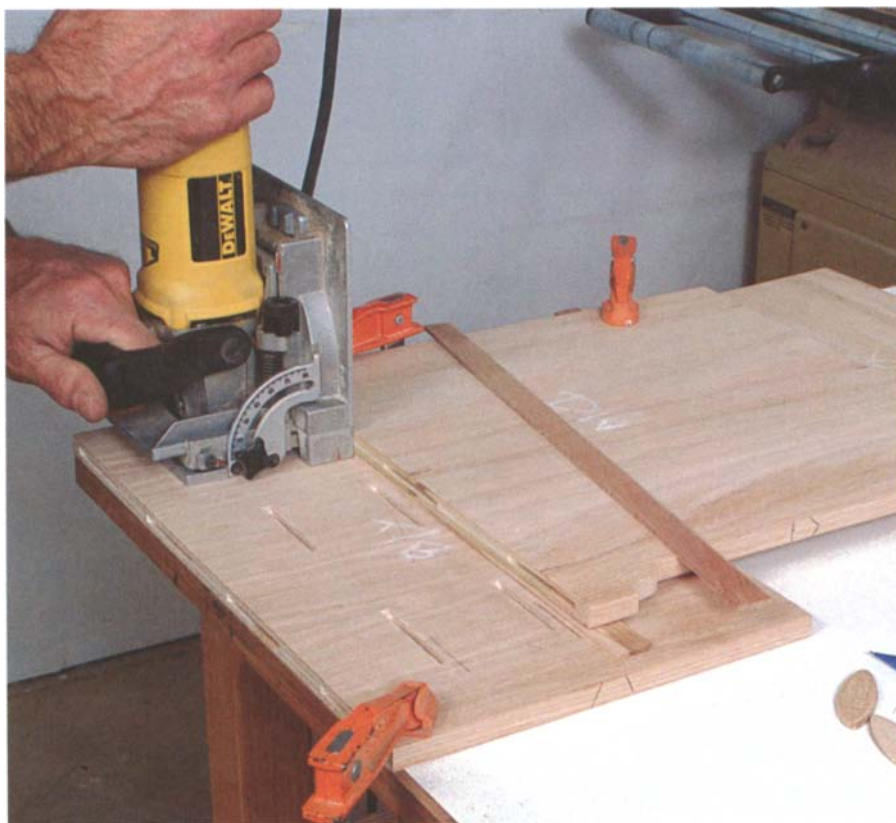
PHOTO G: Square scrap clamped to the case pieces provides bearing for the biscuit joiner fence, preventing angled slots.
