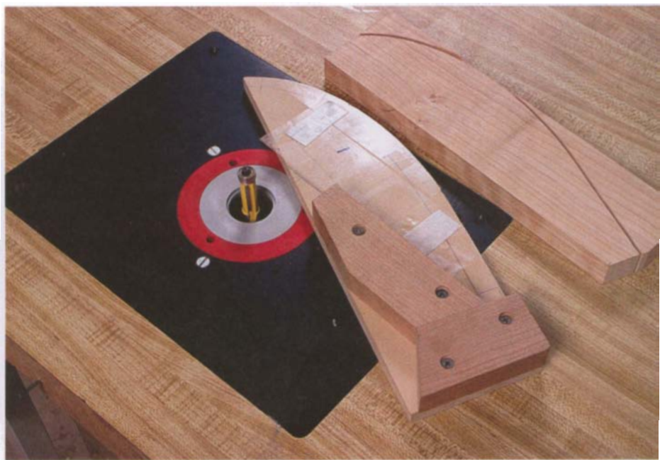
PHOTO 1: After trimming off the bottom corner of the slat blank and bandsawing away most of the waste on the convex edge, the blank is ready for mounting on template jig 1.
