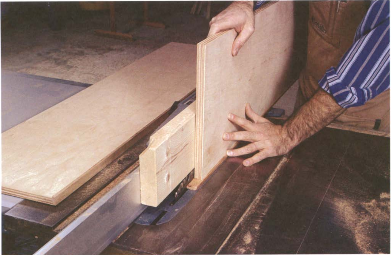
PHOTO A: To rough-trim the solid-wood edging flush to the plywood, screw a shim board to the table-saw fence with the board's face set just a hair past the outside edge of the sawteeth. Afterward, finish up with a block plane.
