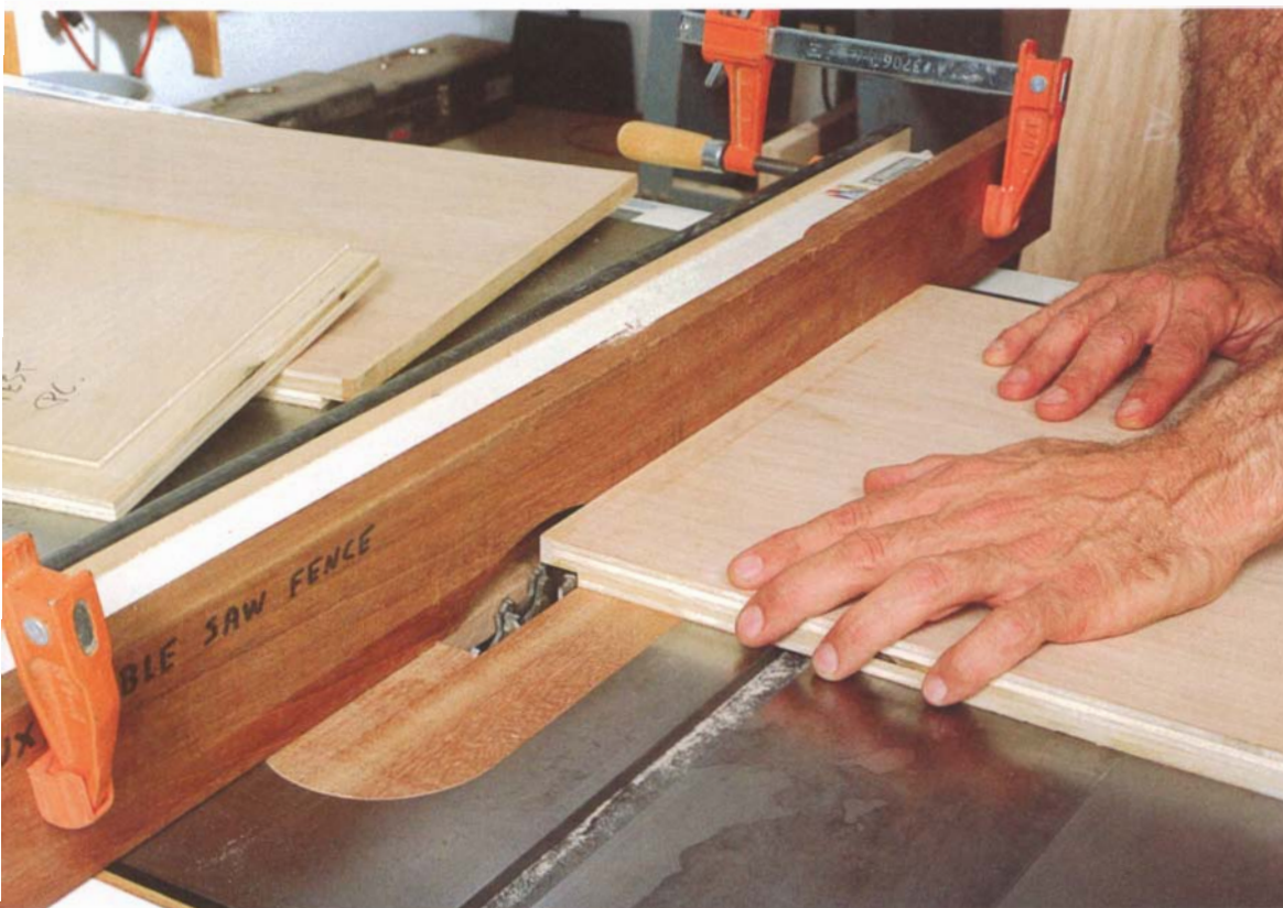
PHOTO A: After applying protective solid-wood edging to the bottom of the side pieces, saw the rabbets in the top and bottom edges using a dado head and an auxiliary rip fence.
