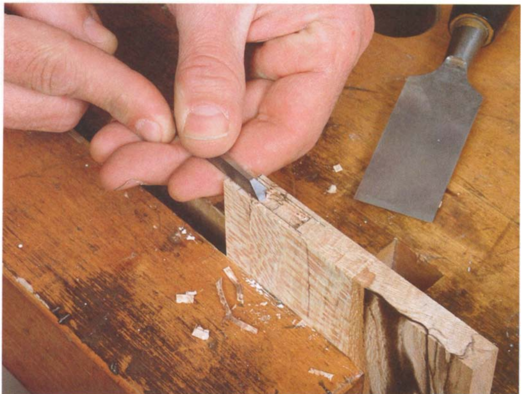
PHOTO E: Clamp the end of the compartment door flush to the benchtop for routing the majority of the waste from the knife hinge mortise.
