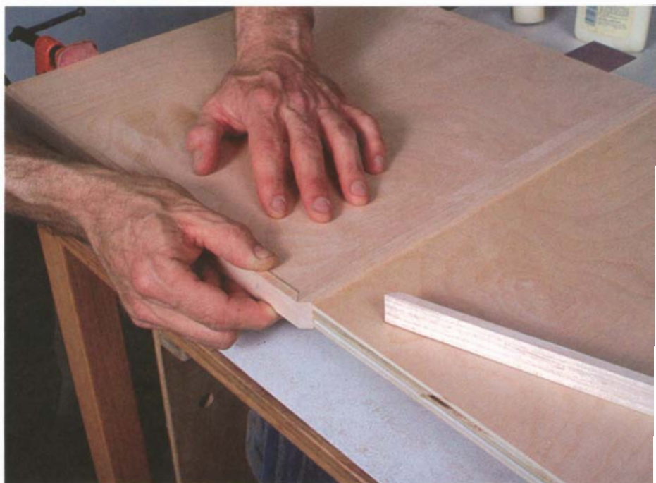
PHOTO C: When fitting mitered edging pieces to length, rest the panels on thin shims and carefully align the inner edge of each miter to its panel corner. Test the fit by holding the adjacent pieces of mitered edging in place against the first miters.
