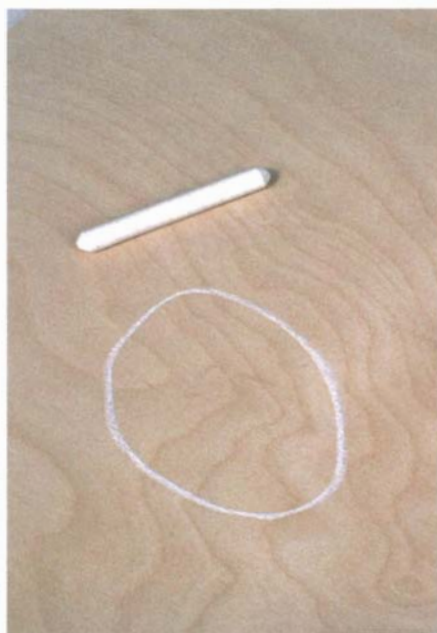
PHOTOS A AND B: Before laying out your plywood, inspect it for flaws using a strong, glancing sidelight in a darkened shop. The scar circled in chalk in the left photo is barely visible in normal light, but under a sidelight (right photo), it's immediately apparent.
