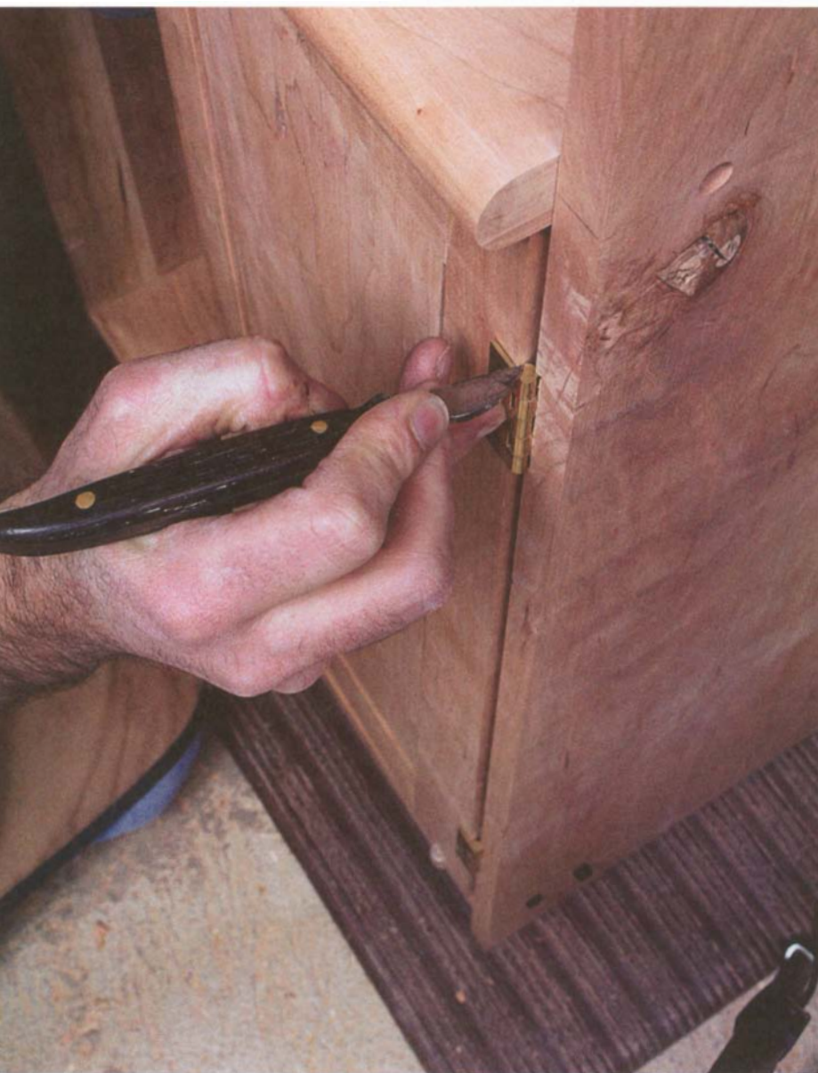
PHOTO K: Replace the door in its opening, straddling a couple of \frac{3}{4} -in.-thick shims. Use a sharp knife to lay out each hinge into the front edge of the stile.
