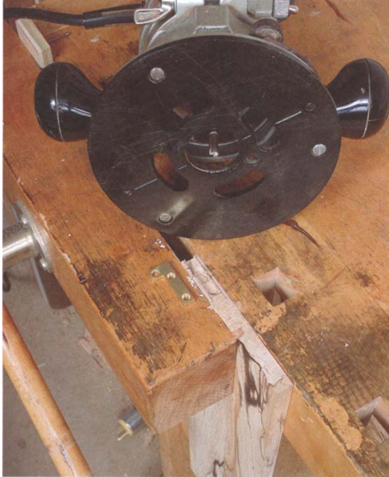
PHOTO E: Clamp the end of the compartment door flush to the benchtop for routing the majority of the waste from the knife hinge mortise.
