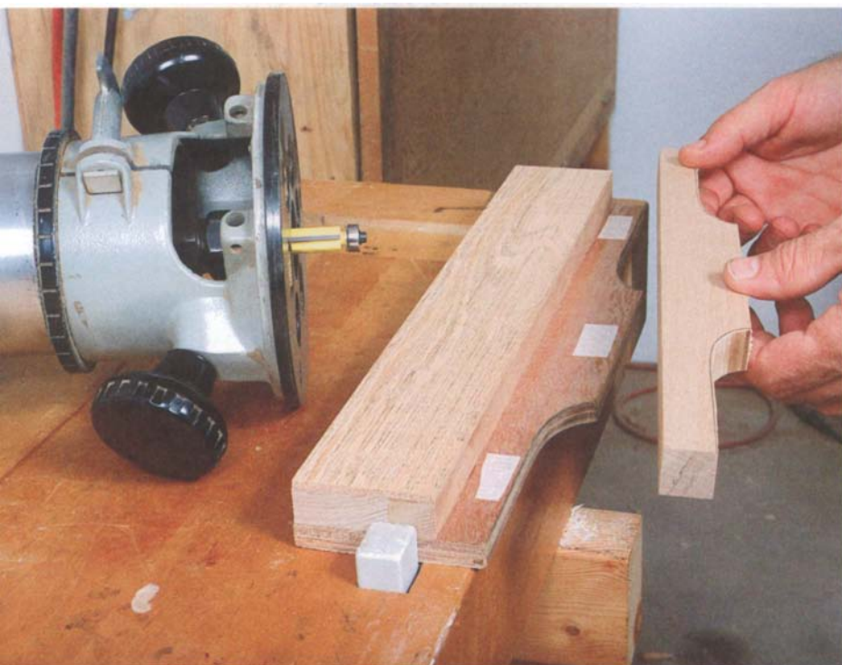
PHOTO D: A template guides a flush-trimming bit for routing the pull to final shape. The wooden fence registers the pull blank and supports the router. Double-sided tape holds the blank to the template.
