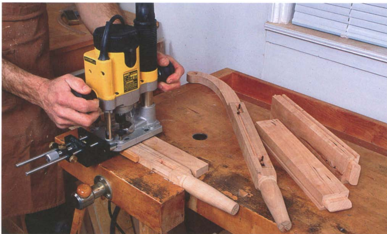
PHOTO H: Rout the side and back panel grooves registering the router edge guide against the inner faces of the legs and rails.
