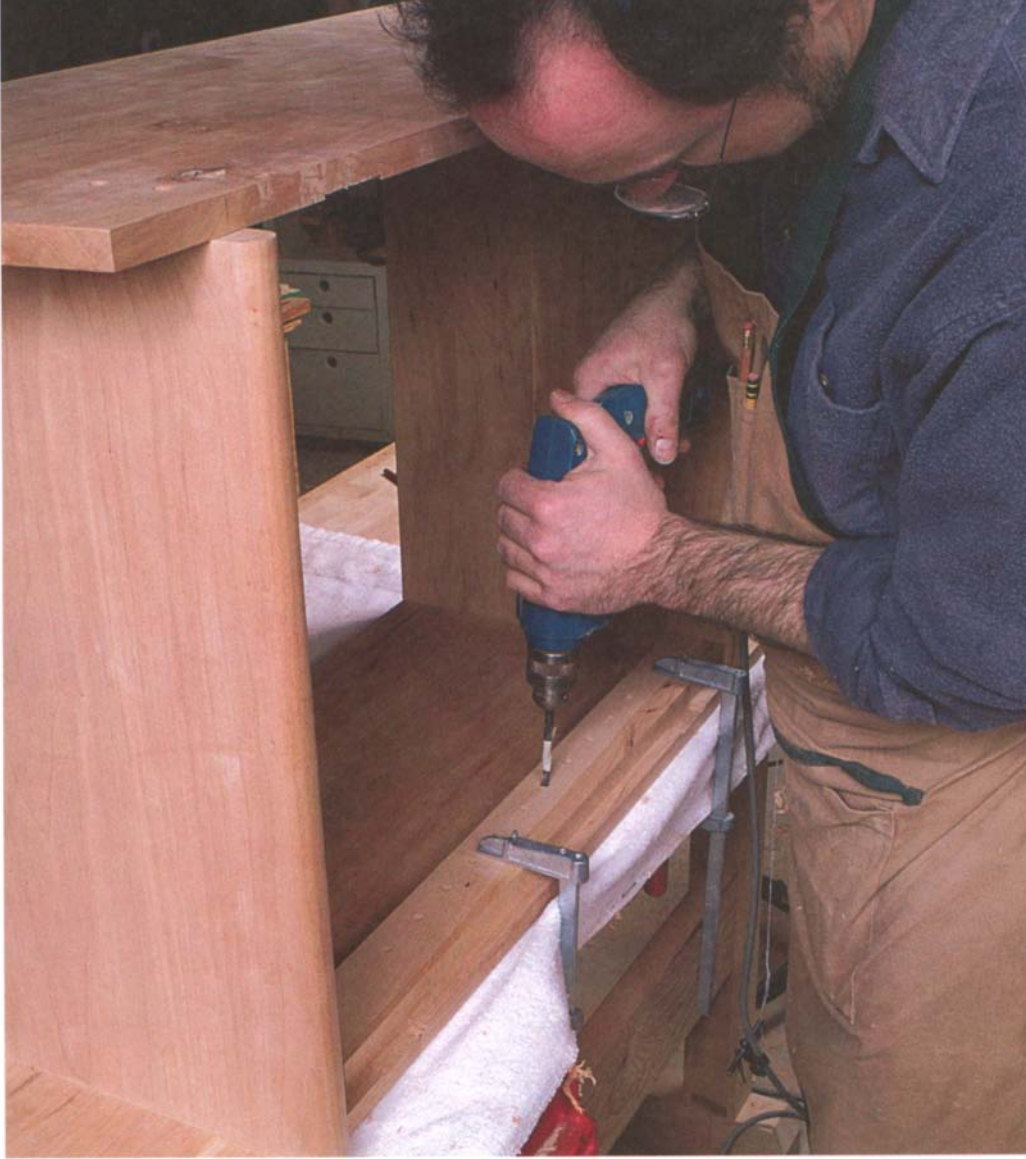
PHOTO H: Burton uses a shopmade drilling template to save layout time and ensure that the shelf support holes are spaced accurately.
