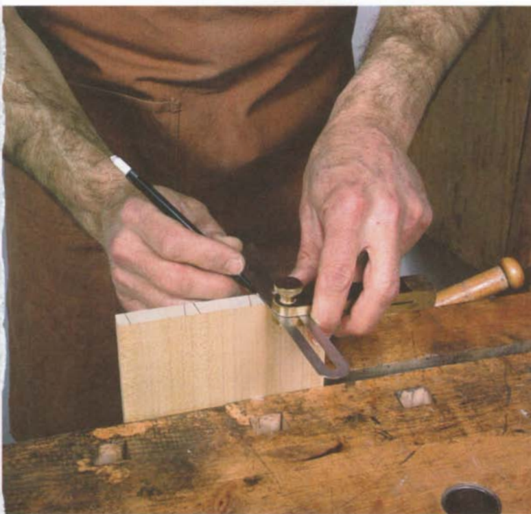
PHOTO A: Lay out the dovetail pins first, setting the bevel gauge to about 82 degrees.
