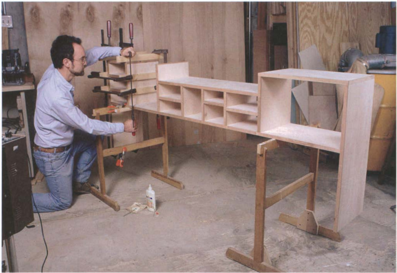
PHOTO D: Burton uses plenty of cauls and clamps to attach the left-hand section to the main shelf. Spring clamps hold cauls in place temporarily for clamping with bar clamps.
