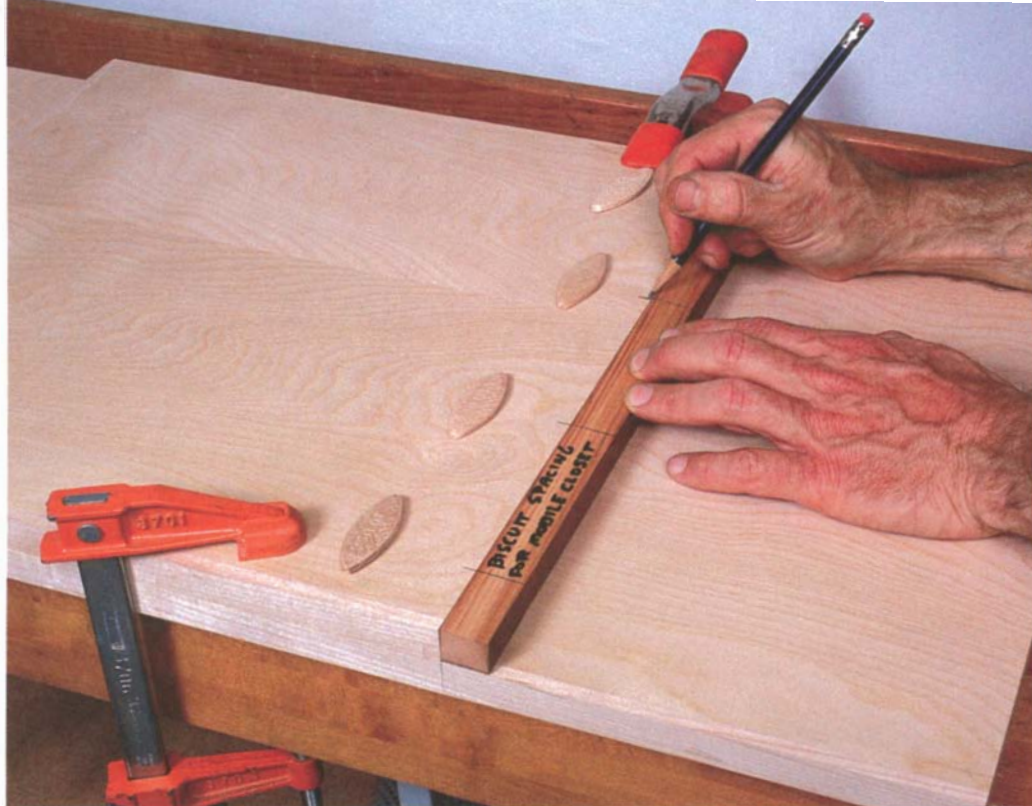
PHOTO F: After laying out the location of the top face of each shelf on the divider, clamp the shelf upside down with its edge aligned to the layout line. Mark the biscuit slot locations on the underside of the shelf.
