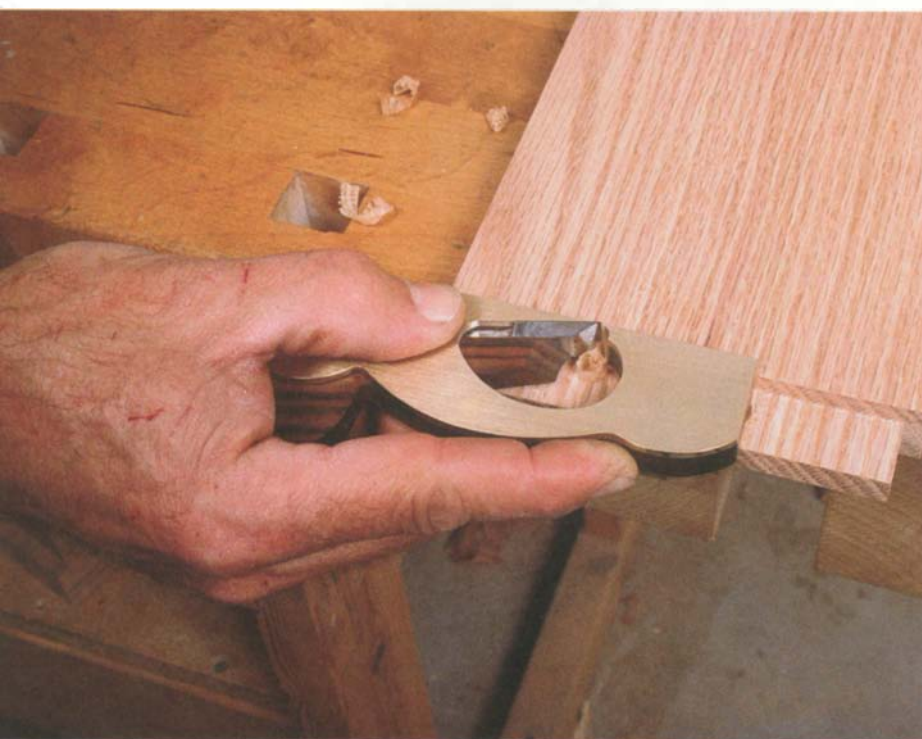
PHOTO C: A shoulder plane makes neat work of trimming tenon shoulders.
