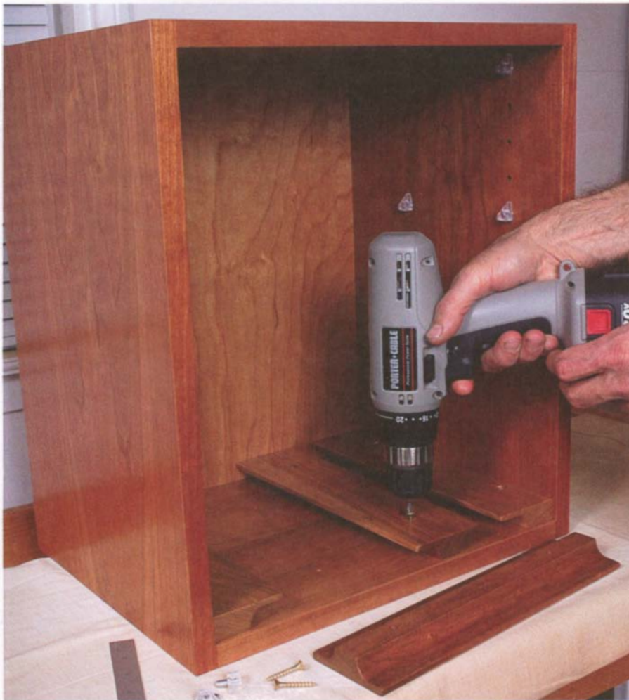
PHOTO D: Screw the wineglass racks to the underside of the case top through predrilled countersunk clearance holes.
