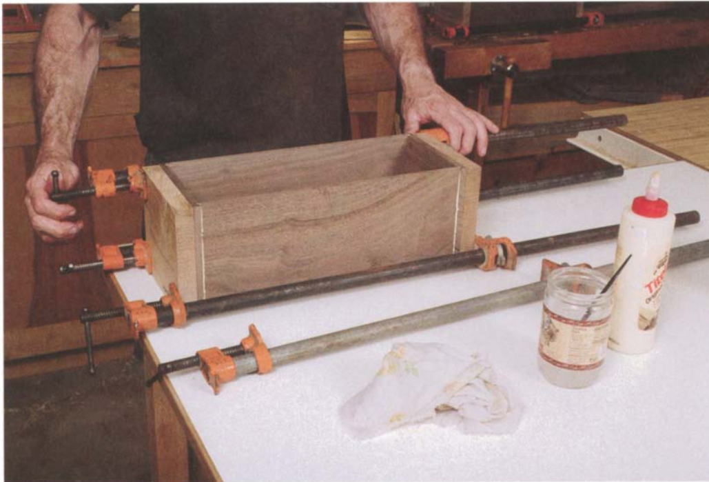
PHOTO D: Place thick hardwood cauls against the box sides to distribute clamping pressure along the joints.
