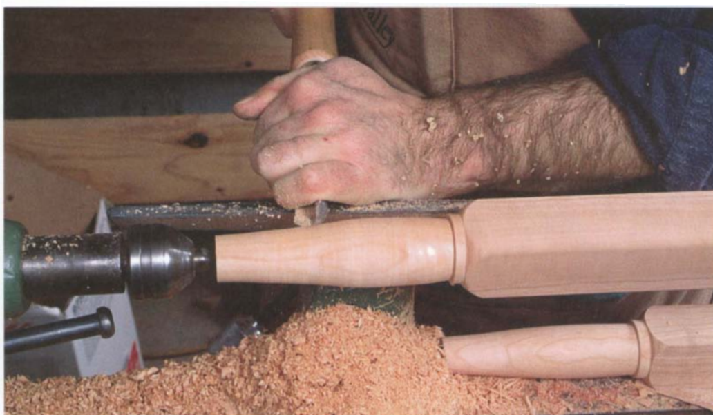
PHOTO E: Shape the rest of the foot profile with a gouge, cleaning up with a skew afterward.
