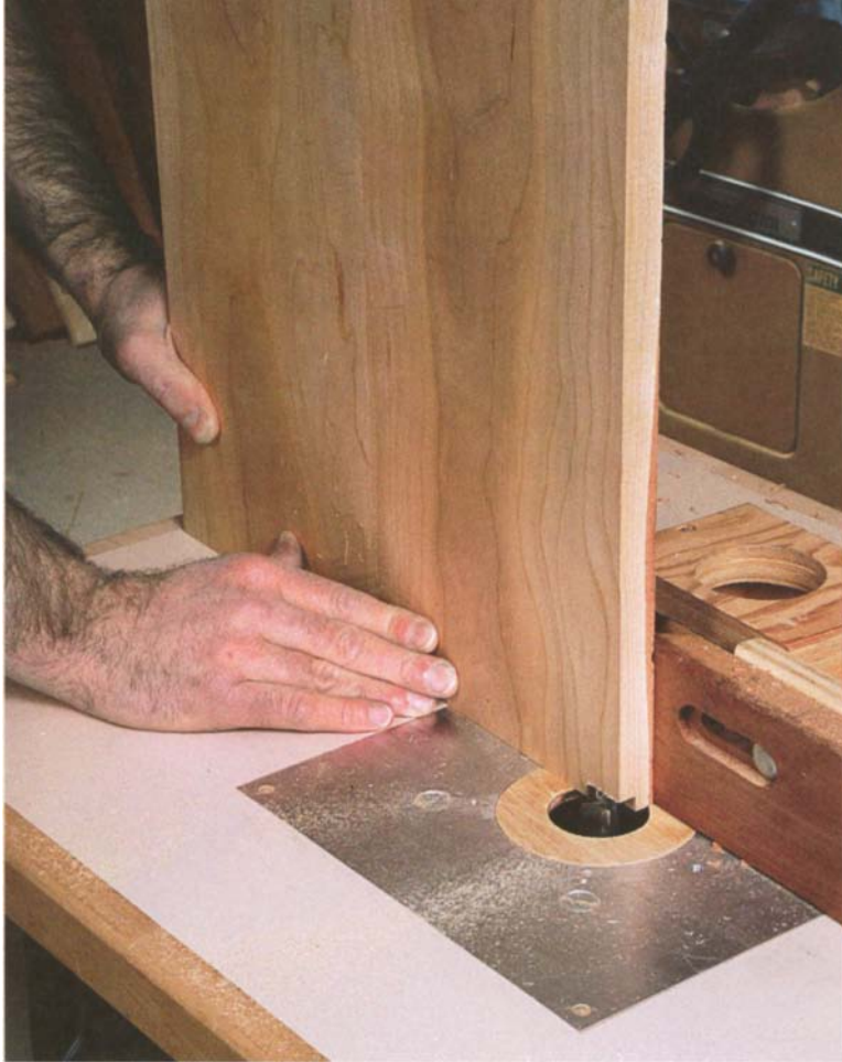
PHOTO A: Cut the rabbet on each end of the top and bottom piece to create the ¼-in. by ¼-in. tongue. Cutting the rabbets on the router table as shown here ensures a tongue of consistent thickness.
