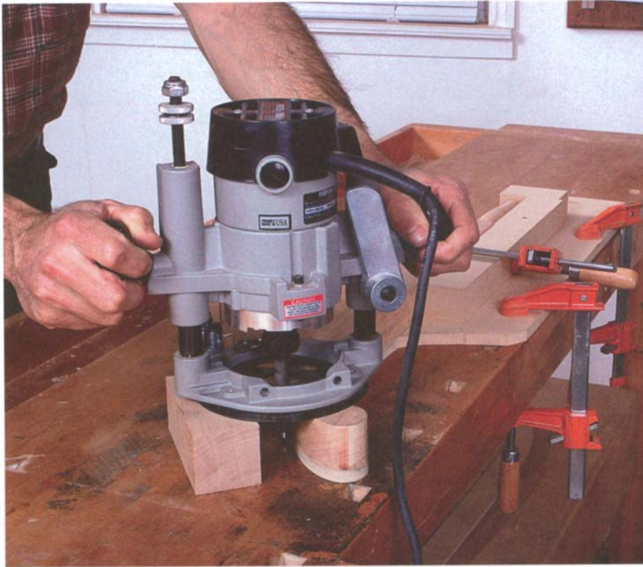
PHOTO F: With the top of the leg held with double-sided tape and the body clamped to the template jig fence, rout the curved section using a flush-trimming bit. A support block taped to the router base keeps the router level.
