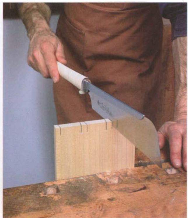
PHOTO B: Saw down carefully to the scribed baseline, keeping the saw vertical.
