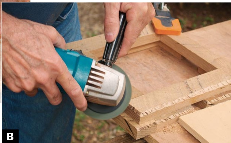
B USE A GRINDER OR RASP TO SHAPE and roughen the edges of the foot assembly. Clamp it tight to a table or workbench. Avoid the temptation to hold it in your hand.
