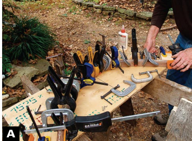
CLAMP THE WALNUT STRIPS TOGETHER EVENLY to the form. This takes a lot of clamps. Start at the middle and work your way to the ends. Apply extra clamps where there are gaps between the strips.
