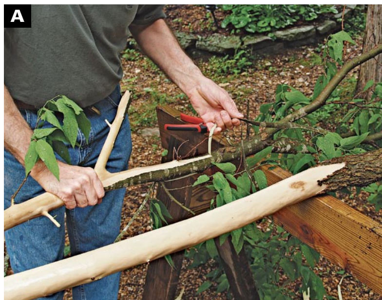
TO PEEL BARK OFF FRESH BRANCHES , start where you cut the branch off. Use a sharp knife to pry under the end of the bark. Then pull strips up toward the top.
