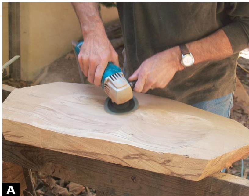
USE AN ANGLE GRINDER TO SHAPE the seat hollows at the center of the slab.
