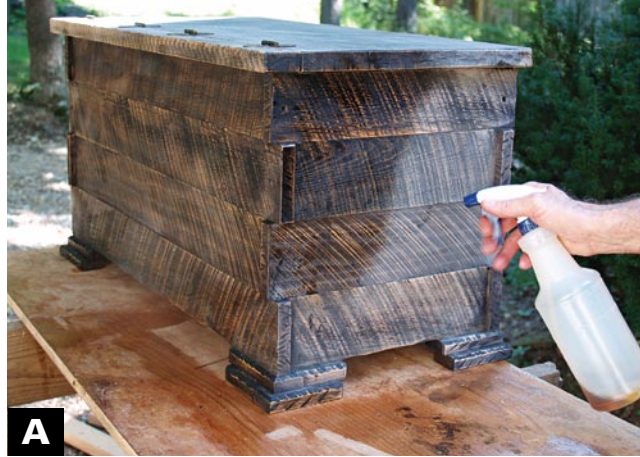
SPRAY DANISH OIL FINISH ON THE CHEST, inside and out, with a spray bottle. Apply two coats 20 to 35 minutes apart, then rub the surface with a dry cloth. A second application and wiping 24 hours later will create a perfect finish.
