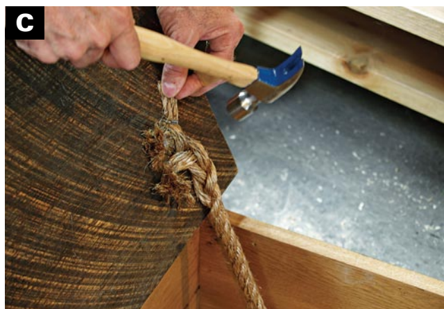
ATTACH EACH END OF THE MANILA ROPE stay to the lid, using large staples. Predrilling is necessary in woods as hard as this oak.
