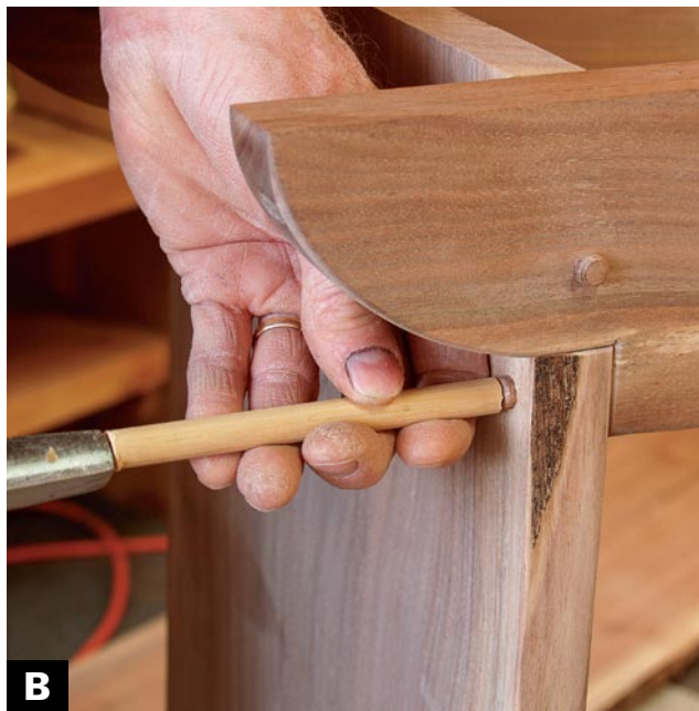
HAMMER THE WALNUT PLUGS IN PLACE with a short dowel as a nail set to avoid damaging them.
