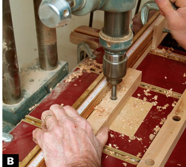
DRILL HOLES IN THE END STRETCHERS for dowels to be used to attach the stump to the frame.
