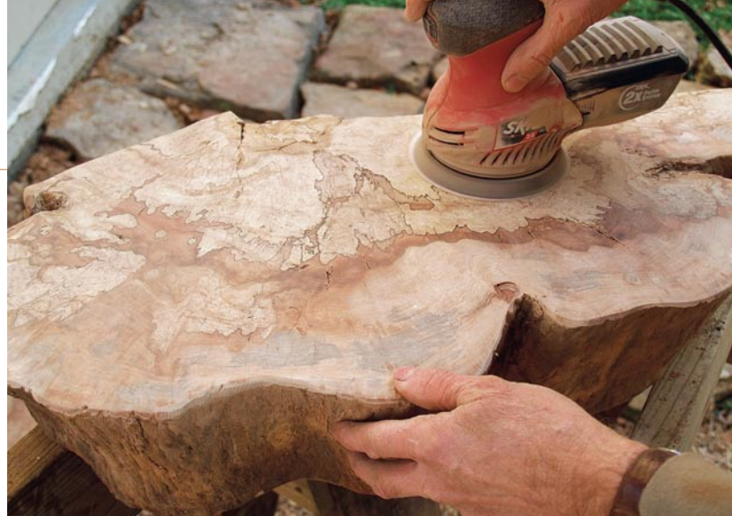
SAND THE END-GRAIN surface of the stump.
