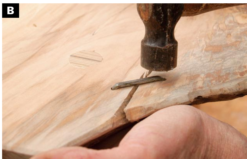
HAMMER THE HANDMADE STAPLE ACROSS the crack, holding the stock from below to prevent further cracking.
