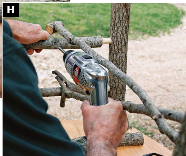
WITH A DIAGONAL STRETCHER CLAMPED in place, use it as a guide to drill the mortise at the proper angle.
