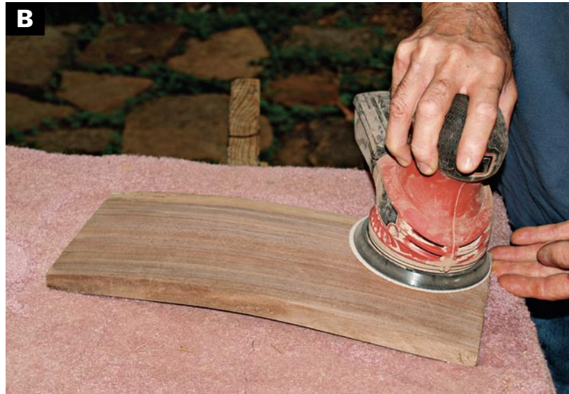
FINISH SAND THE SEAT BACK with a random-orbit sander after you've shaped it.
