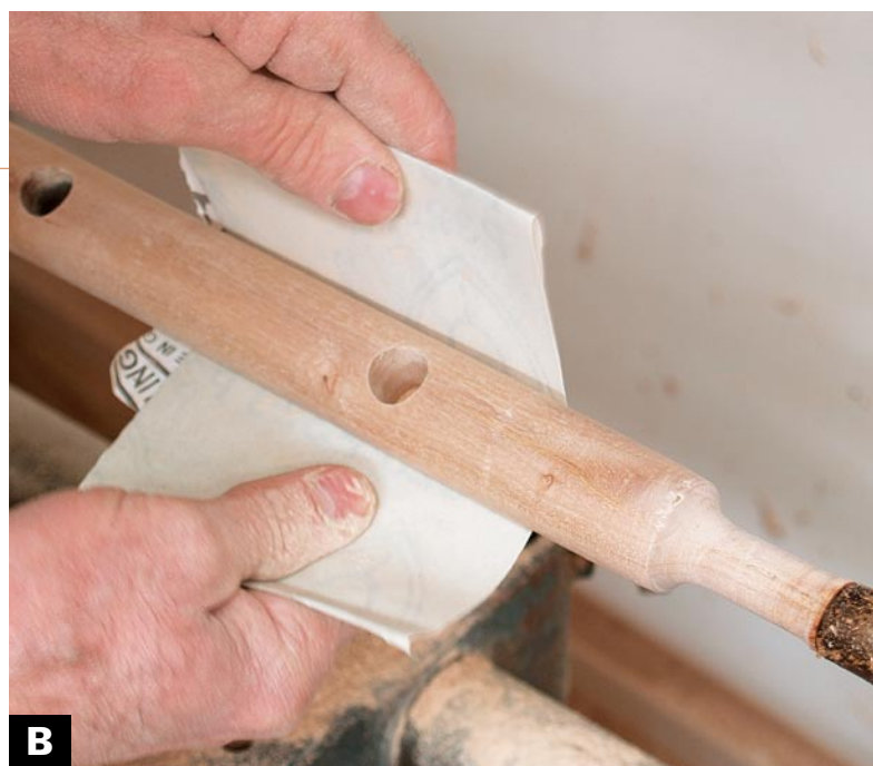
SAND THE STRETCHERS ON THE LATHE. Work your way through the normal grits, with the lathe running, of course.
