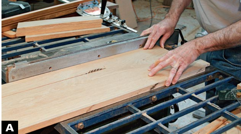
A RIP STOCK INTO PIECES FOR THE TRESTLE BASES according to the dimensions in the materials list.
