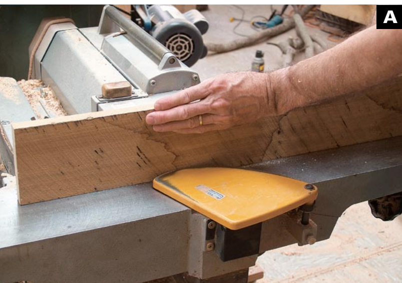
EDGE-JOIN EACH BOARD. A power jointer is most effective, particularly where the boards may be slightly warped.
