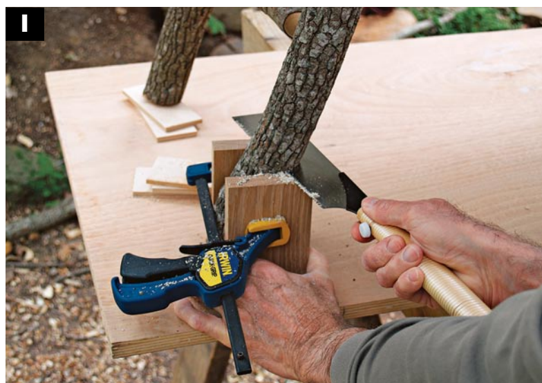
TRIM THE LEG ENDS with the table leveled. Clamp guide blocks to the legs as a saw guide and trim all the legs the same distance from the bench top.
