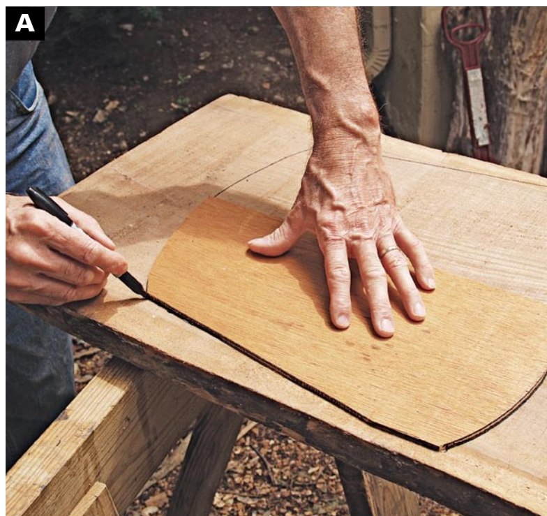
MARK OUT THE SEAT on the blank with a half-template.
