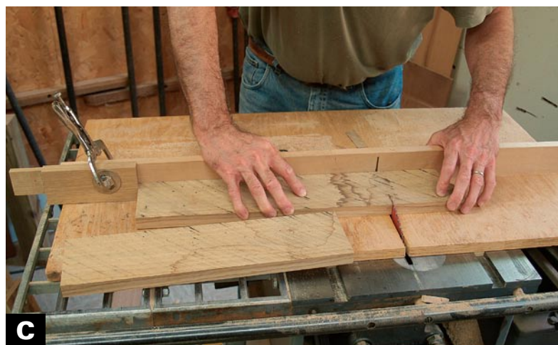
CROSSCUT THE BOARDS TO THEIR FINISHED lengths. I use a sled on the tablesaw for the most accurate results.
