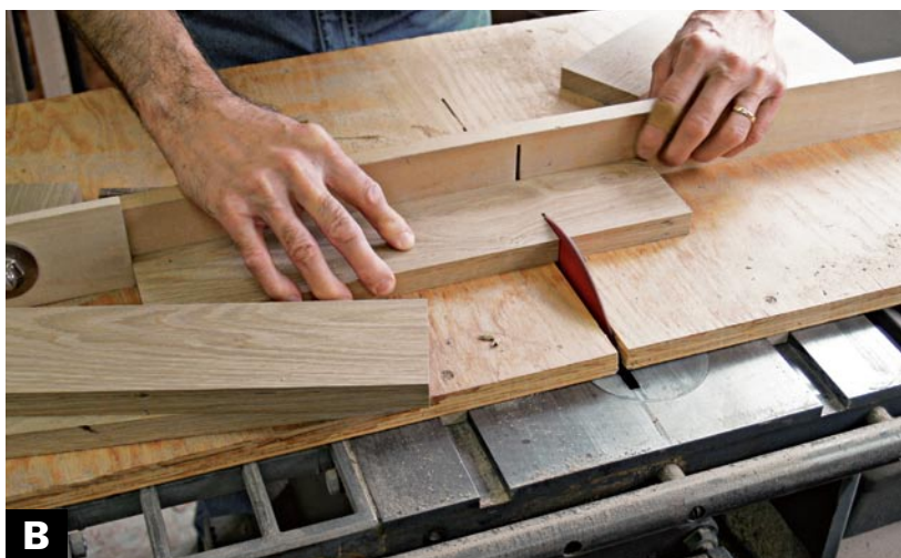
B USE A SLED AND STOP BLOCK ON THE TABLESAW to cut the parts to length. First trim one end square, then slide the stock against the stop block and cut. Each piece cut in this manner will be exactly the same length.
