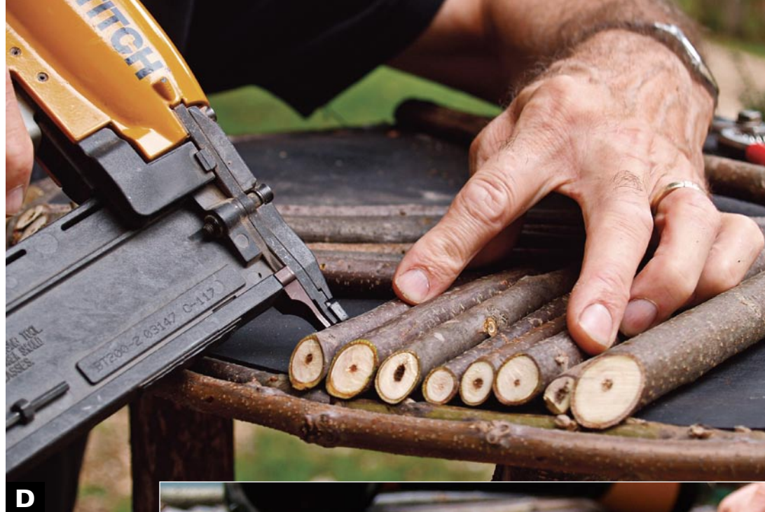
ARRANGE AND NAIL TWIGS in place on the top.
