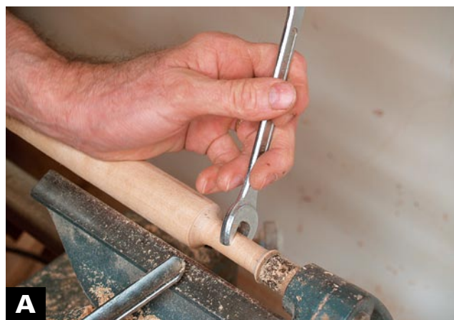
I USE AN OPEN-END WRENCH TO CHECK the measurements as I turn to make sure I don't turn the tenons too small. An exact fit of the open-end wrench often results in a too-tight fit. But a little sanding will make it just right.
