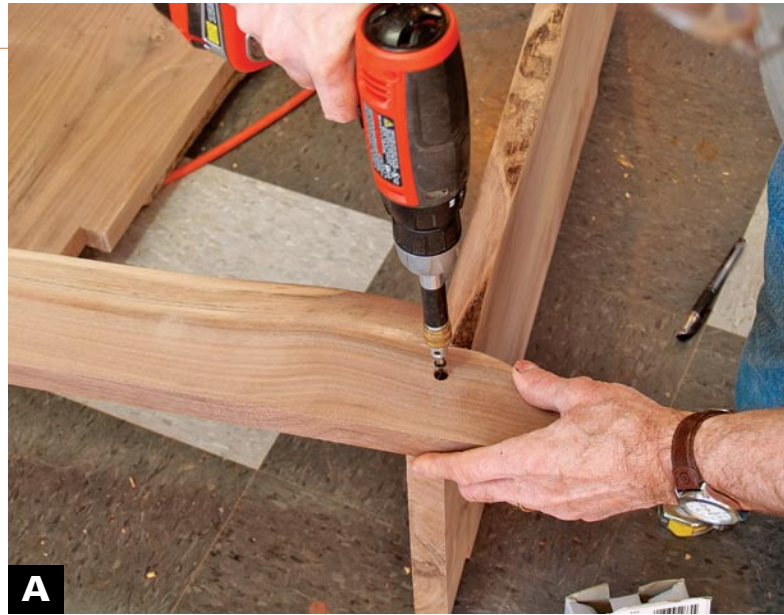
COUNTERSINK WOOD SCREWS to secure the joints. The screws will be hidden with raised walnut plugs.
