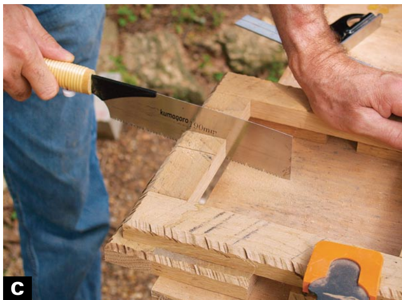
C USE A HANDSAW TO CUT the foot assembly into four separate feet.
