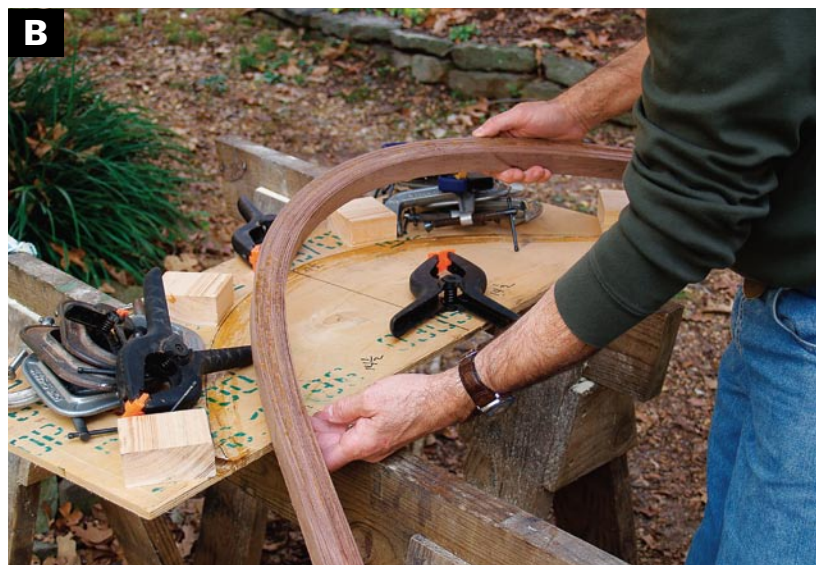
CLAMP THE WALNUT STRIPS TOGETHER EVENLY to the form. This takes a lot of clamps. Start at the middle and work your way to the ends. Apply extra clamps where there are gaps between the strips.
