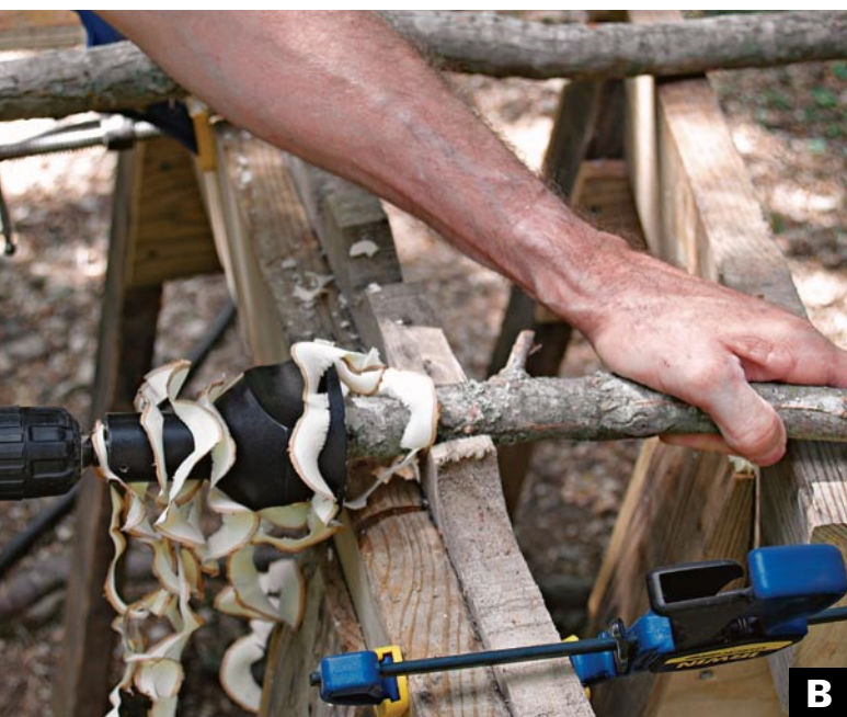
CUT \frac{5}{8} -IN.-DIA. TENONS on the cross stretchers for the front and back.
