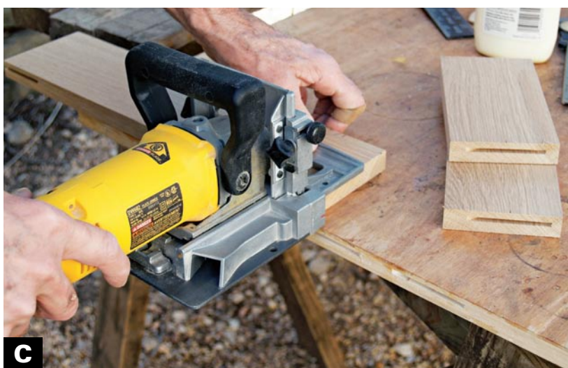
C CUT #20 BISCUIT SLOTS IN THE middle-layer pieces to join the parts.
