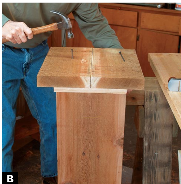
B NAIL THE TABLE ENDS TO THE BOTTOM SHELF using the same technique as used for the side table. To keep the longer coffee table steady while nailing, I use a sawhorse instead of a crate.
