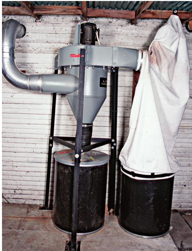
The funnel-shaped cyclone on this 3-hp central collector separates out chips and larger dust particles, depositing them in a drum under the unit for easy disposal.
