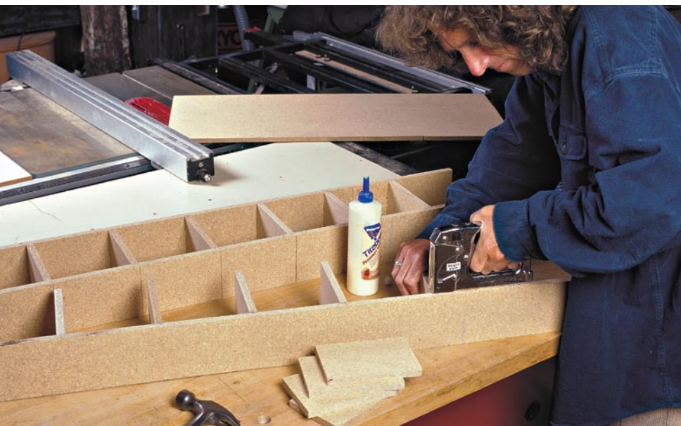
Shop assistant Stu Sutcliffe uses glue and staples to assemble the \frac{1}{2} -in. particleboard inner gridwork for a torsion-box worktable top. Despite its cheap inner construction, the tabletop—once skinned with \frac{3}{4} -in. plywood on both sides—will be light, flat, and incredibly rigid.
