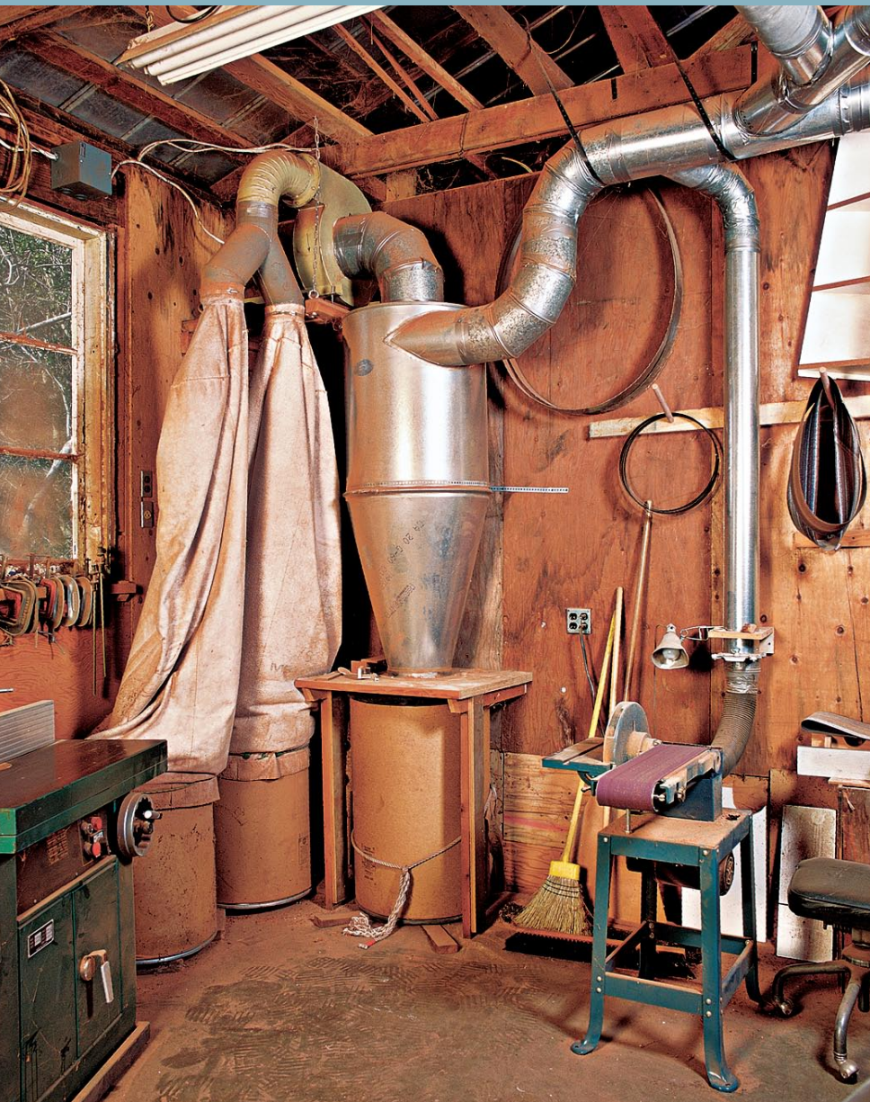
The essential components of a return-air central dust-collection system—preseparator cyclone, blower, and filter bags—are mounted inside the shop in a corner where ductwork brings chip-laden air from machines all around the shop.
