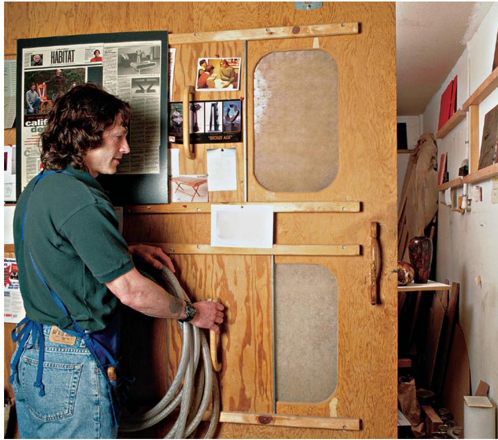
Woodworker David Marks uses inexpensive furnace filters fitted into cutouts in the door to his finishing room to allow proper ventilation yet prevent dust generated in his adjoining woodshop from ending up in a freshly finished turning or furniture piece.
