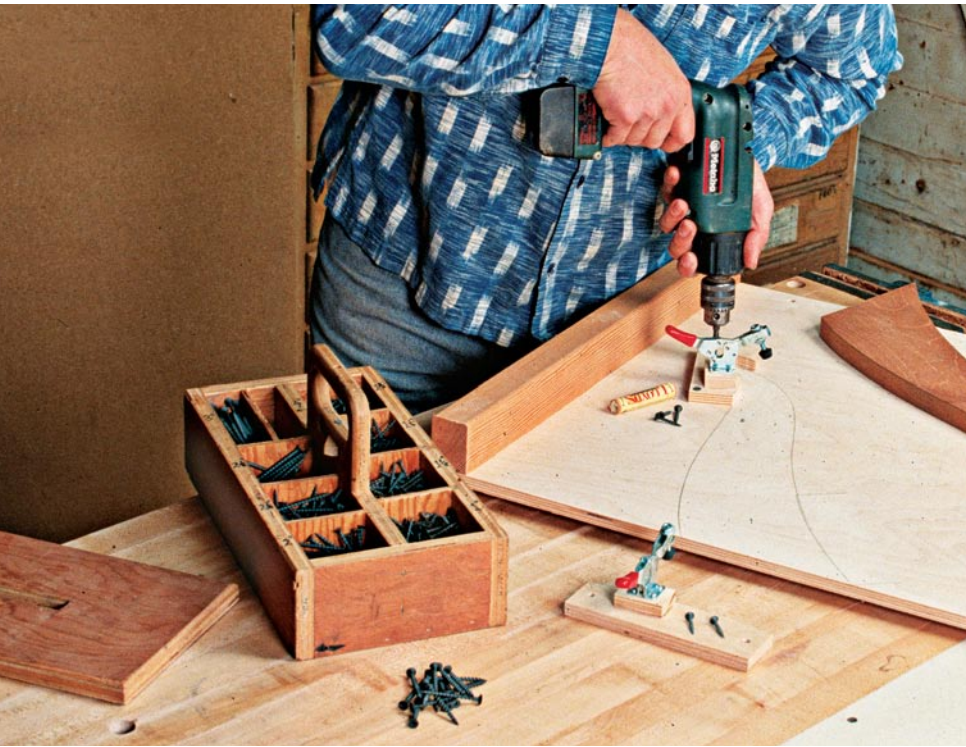
Not only does this shopmade plywood screw box house and organize nine different sizes of screws but its locking lid keeps them from spilling or getting mixed up if the box is dropped or inverted.
