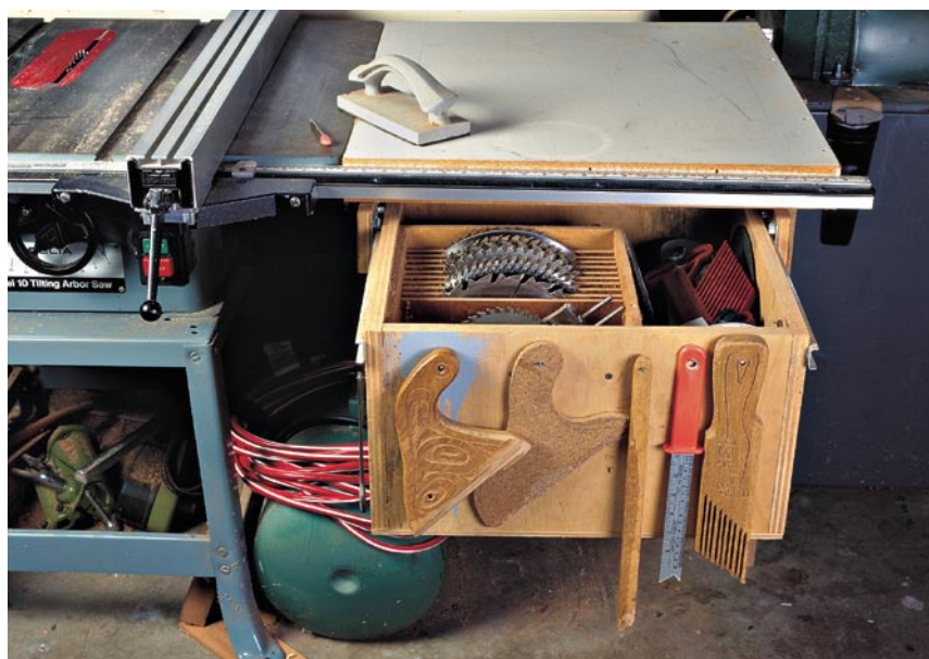
A drawer mounted on full-extension glides beneath the extension table of this tablesaw has divided compartments that hold extra sawblades safely and has room to store saw accessories—throat plates, push sticks, and safety devices—right next to the machine.
