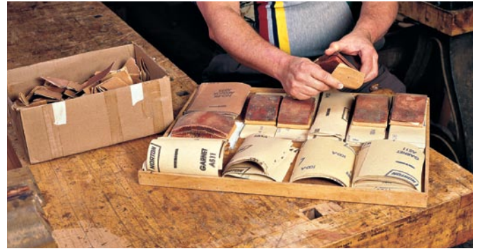
A simple wood tray keeps sanding blocks and various grits of sandpaper from getting mixed up as well as provides an easy way to move all these hand-sanding supplies to wherever they're needed in the shop.
