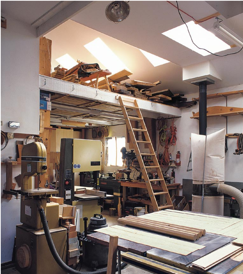
Adding a loft to a shop with a tall, vaulted ceiling is one way to add storage in a small space. A sturdy ladder that engages hooks on the edge of the loft to keep it from sliding provides ready access to the lumber stored in this good-size loft.
