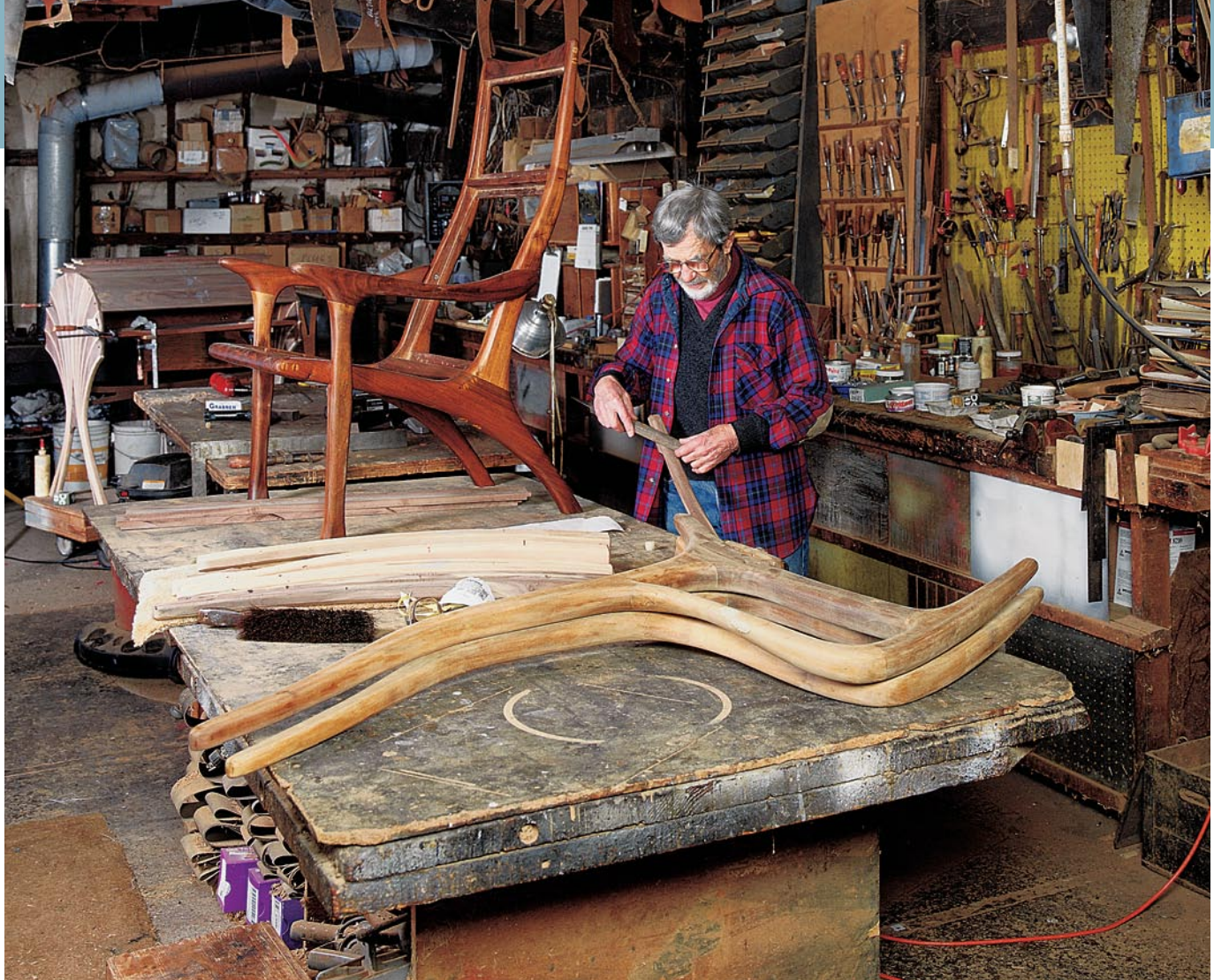
California master woodworker Art Carpenter's versatile workbench serves multiple functions. With a particleboard cover, it becomes a work table for assembling projects, such as these walnut armchairs. With the cover removed, the thick subtop is riddled with holes used for positioning and clamping bent-wood laminations.
