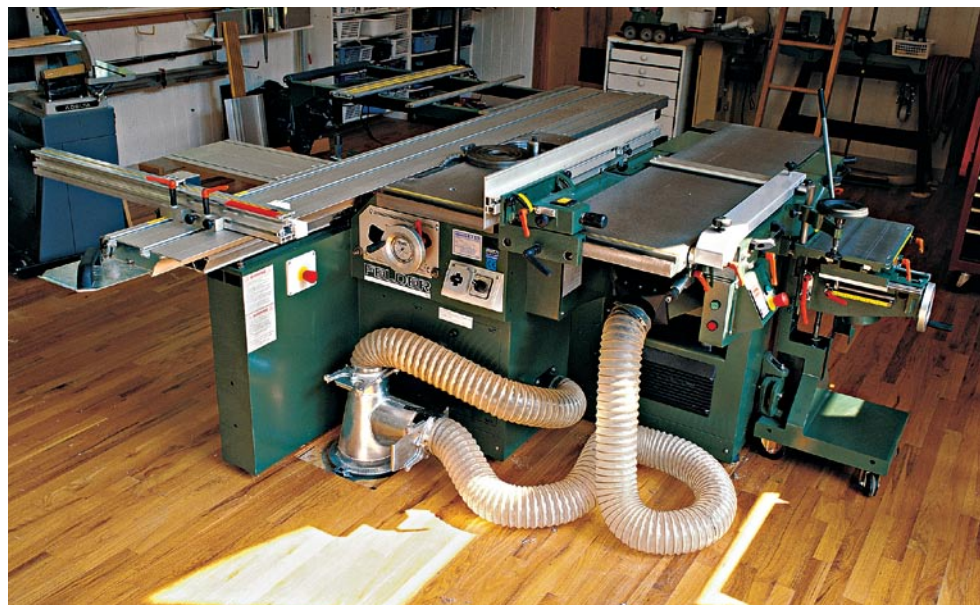
When workshop space is scarce, a combination machine can provide all the machinery you need in a very compact package. This Felder® machine integrates a big tablesaw (with a panel-cutting attachment) with a planer/jointer, shaper, and horizontal mortiser.
