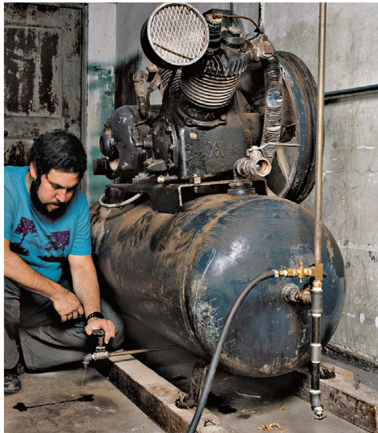
Even the largest, professional-model compressors condense moisture from the air they pressurize. Hence moisture must be drained from the compressor regularly via a valve or petcock at the base of the tank.
