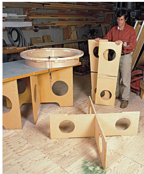
California master woodworker Art Carpenter's versatile workbench serves multiple functions. With a particleboard cover, it becomes a work table for assembling projects, such as these walnut armchairs. With the cover removed, the thick subtop is riddled with holes used for positioning and clamping bent-wood laminations.
