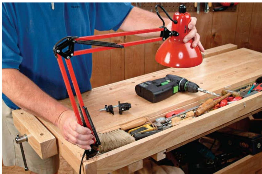
Adjustable, drafting lamps are ideal task lighting fixtures for the workshop. Most lamps come with a base that clamps onto a thin tabletop, or you can fit the lamp's base stem into a 1/2-in. hole drilled into a benchtop or wooden mounting block.
