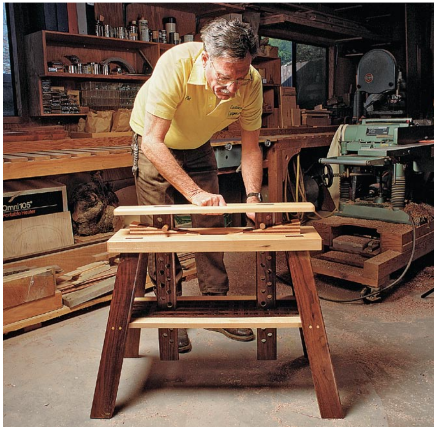
Portable, versatile, and sturdy—a pair of good sawhorses can elevate and support workpieces in lieu of a worktable or bench. To make his beautiful walnut and maple sawhorses more versatile, Pat Curci added a wedge-locking adjustable-height mechanism.
