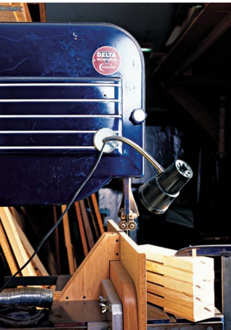
A gooseneck lamp with a magnetic base makes a handy task light that can be quickly mounted to the metal body or table of a machine, such as this band-saw set up for resawing, to shed light exactly where it's needed.
