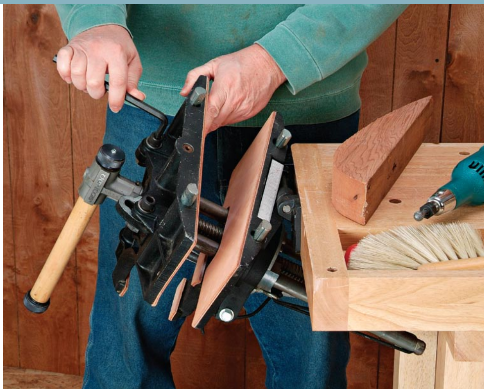
The extremely versatile Veritas Tucker vise has jaws that can rotate, tilt, and even be set out of parallel to hold irregular workpieces.
