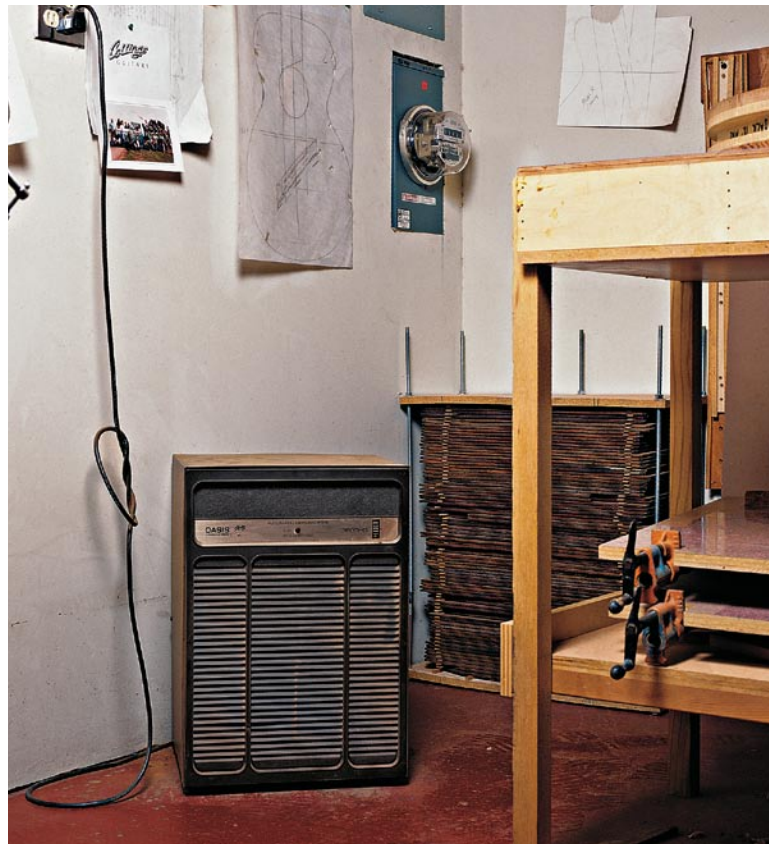
A portable dehumidifier can help you control excess humidity in your shop, which can rust tools and wreak havoc on the moisture content of lumber, wood parts, and projects.
