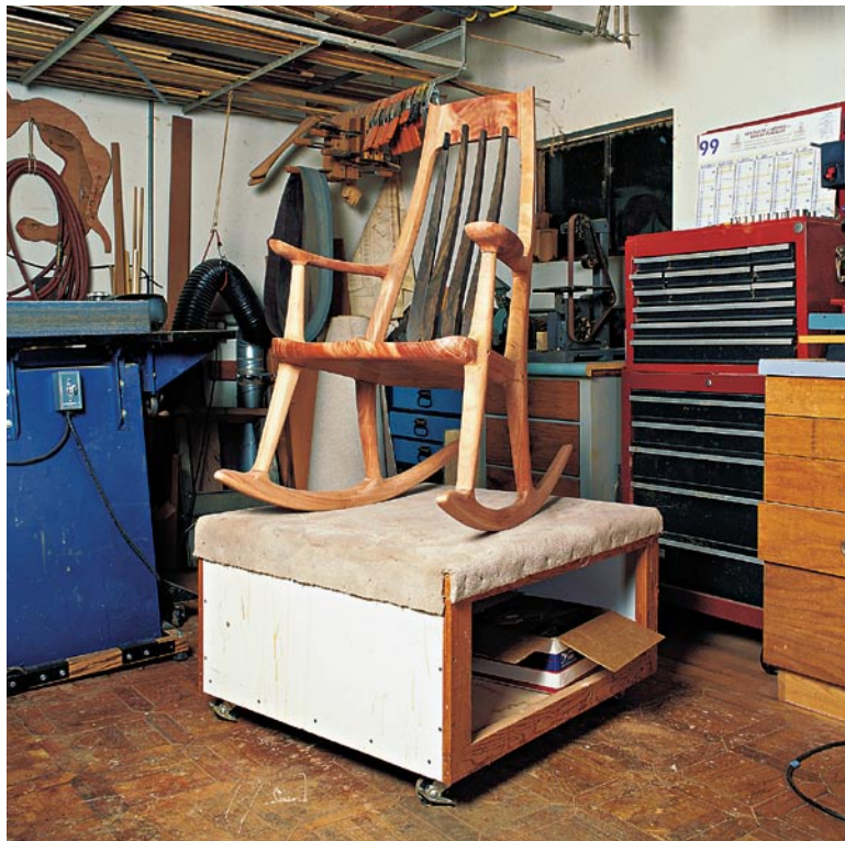
Del Cover covered the top of a simple boxlike wood cabinet with carpeting and fitted locking wheels on the bottom to create a mobile workstation that he uses when assembling and completing projects, such as this handsome mahogany and ebony rocking chair.
