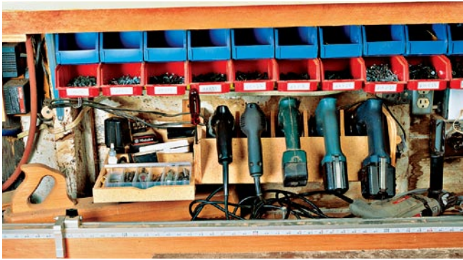
A shopmade electric drill rack, with separate slots for corded and battery-powered drills, keeps the tools and their accessories handy. Colored bins above the rack hold different-size screws—a size for practically every occasion.
