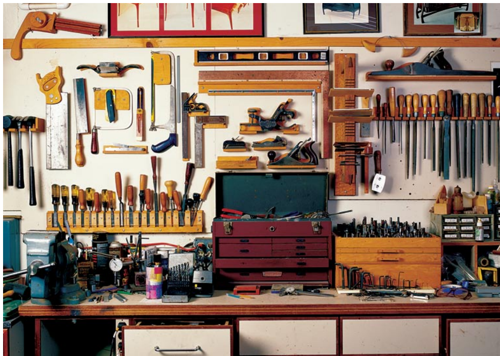
A traditional shop organizer, a pegboard nailed to the wall and fitted with all manner of hooks, loops, and racks is a flexible system for storing tools large and small. Holes bored directly into a post next to the drill press in this shop store dozens of drill and auger bits.
