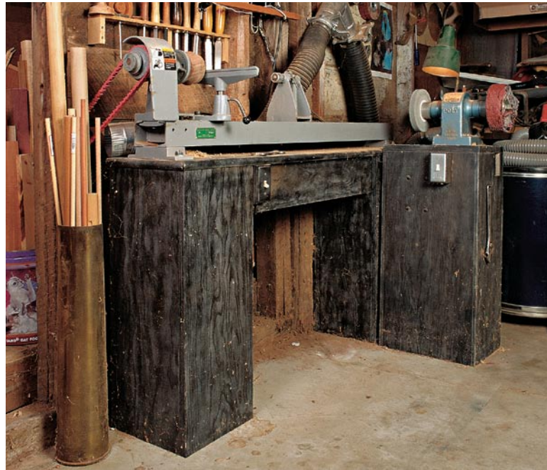
Three simple plywood boxes bolted together and filled with beach sand provide a heavy, stable base for this small wood lathe, actually improving its performance by dampening vibrations that occur during turning.
