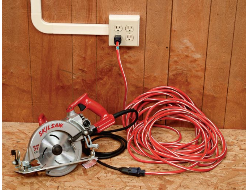
Using a thicker extension cord with heavier-gauge wires (a 12-gauge cord shown here) for large portable power tools not only prevents overheating and fire danger but ensures better tool performance.
