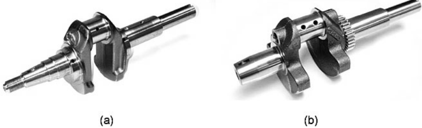
FIG. 7-37 Forged (a) and cast-iron (b) crankshafts used in Dr. Fatemi's study.
