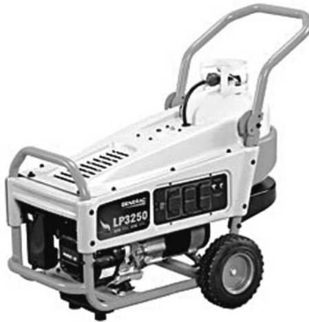
FIG. 1-5 A Generac residential generator, rated at 3250 W and adapted for propane use. The 20-lb tank provides 9 hours of half-load running time between refills. Gempler's
