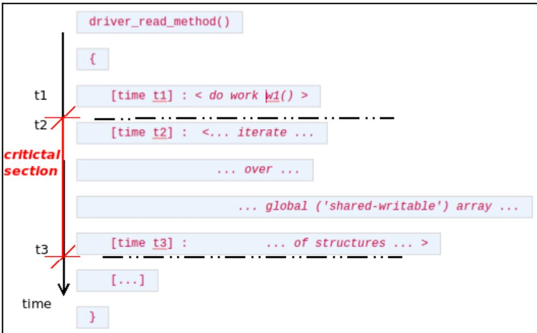
Figure 12.5 – Pseudocode – a critical section within a (fictional) driver's read method; it's wrong as there's no locking
