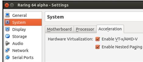
Figure 1.2 – Enabling hardware virtualization options within the VirtualBox VM settings
