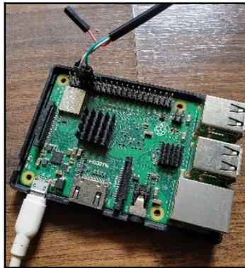
Figure 1.5 – The Raspberry Pi with a USB-to-serial adapter cable attached to its GPIO pins
