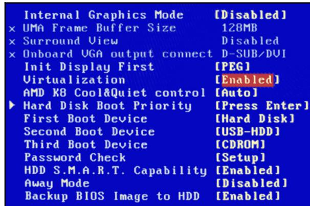
Figure 1.1 – Setting the BIOS Virtualization option to the Enabled state
