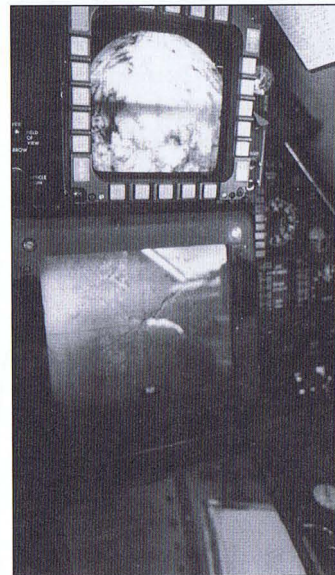
The RSO's view-sight display can be seen at the top of this photograph, with the Synthetic Aperture Radar (SAR) display screen immediately below it. When re-equipped with SAR, the SR-71 was used extensively to obtain extremely high-resolution imagery of target areas obscured by cloud (Curt Osterheld)
