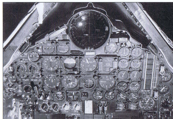
In spite of its radical external appearance and awesome capabilities, in the cockpit the A-12 was generally conventional, as this 8 November 1965 shot taken by Lockheed technicians illustrates (Lockheed)
