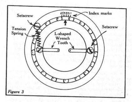
The outer race is engraved with one of the burglar etching tools to a scale of 1-7 and a mark engraved in the inner race to match the scale. The coil spring can be changed at will and made shorter/longer to provide a true scale reading and different pressures. The outer race is fixed to wooden doors with two light nails or spikes, and a couple of magnets epoxied to the outer race (clean of all grease first) will hold it to a steel-clad door for light pressure applications.
