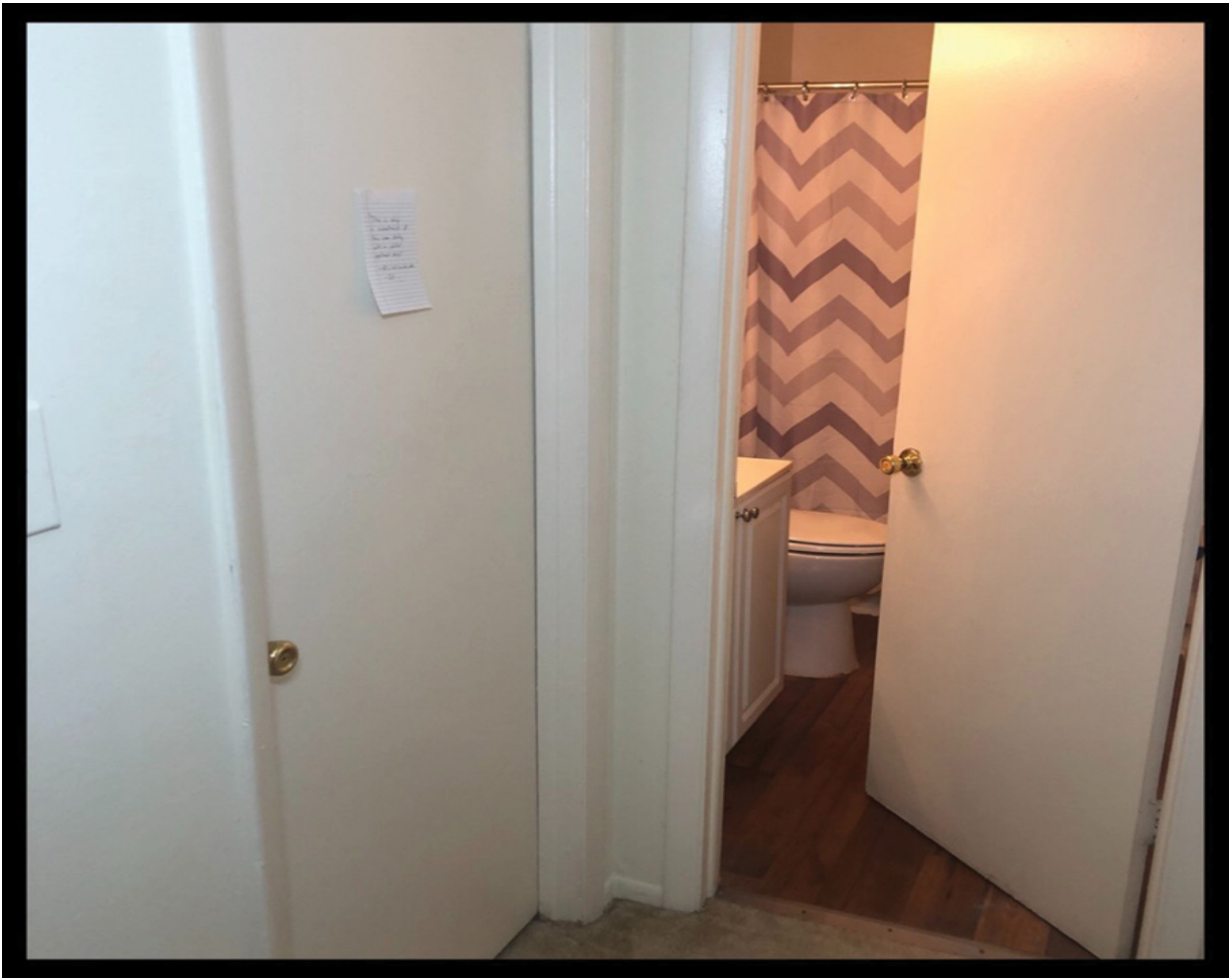
Master bedroom door and an adjacent bathroom. Old and inexpensive privacy knobs like these usually have a twist lock or a push-button lock on the inside, and on the outside they have a small hole that can be used to access a lock override.
