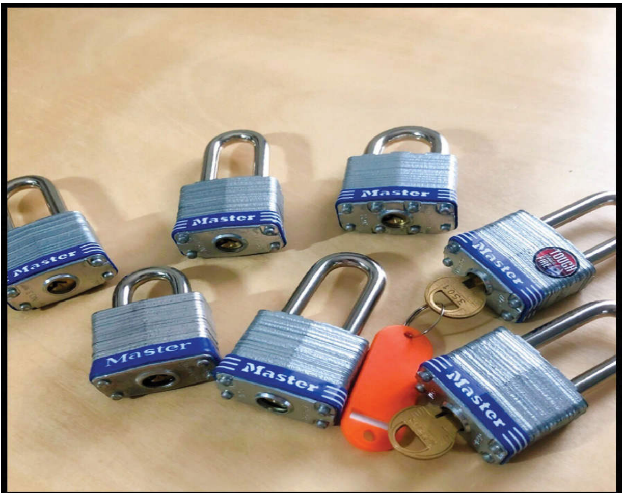
Seven padlocks of the same make/model (with some slight variances) that can all be opened with just two keys.
