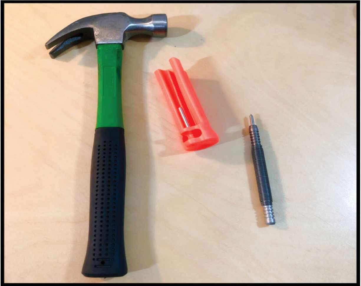
A very inexpensive setup that can get you through a lot of doorways where the locks may be too tough to pick (left to right): a hammer, Bang-It hinge-pin-removal tool, and spring-loaded hinge-removal tool.
