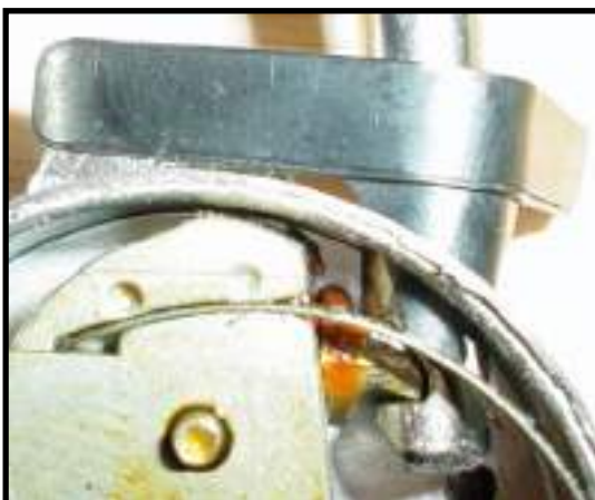
Locked – Bolt Extended/Shim Inserted.
