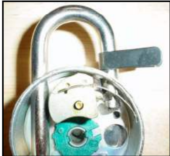
Unlocked – Bolt Retracted/Shim Turned.
