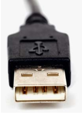
Universal Serial Bus (USB) is an open standard for the connection of computer peripherals to personal computers.
