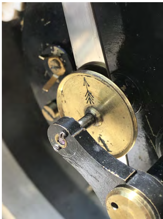
Figure 6.1 The jewelled pivots holding in place the needle of a George-built Fox type, dating from around 1845. Note the groove around the edge of the needle's central wheel (Author's picture, 2020).
