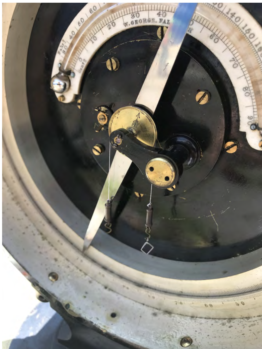
Figure 6.12 An intensity experiment with a George-built Fox type, showing the suspension of weights by silk thread from the grooved wheel of the dipping needle. Weights could be added to the hanging hooks to coerce the needle to its original dip (Author's image, 2020).
