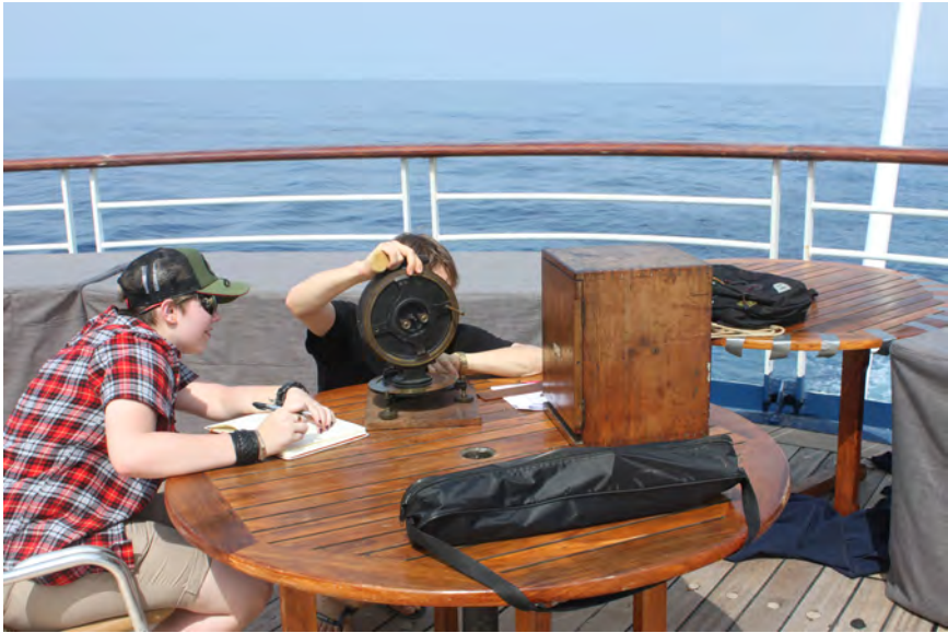
Figure 8.2 Performing a magnetic measurement with a Fox-type dipping needle on a calm Indian Ocean, off the east coast of Madagascar in February 2020 (Author's image, 2020).
