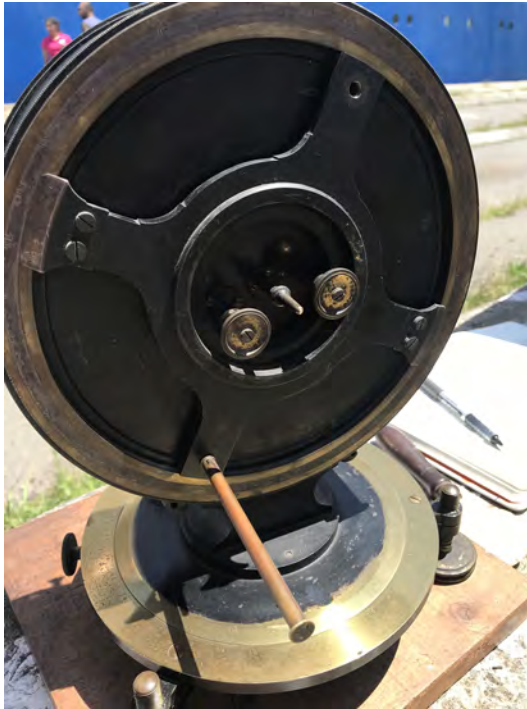
Figure 6.2 The back of a Fox type showing the insertion of one of the cylindrically encased deflector needles. At the top of the circle is a second hole for the second deflector, which can be screwed in. Note that both sit on a disc that can be rotated to an angle in reference to dip (Author's image, 2020).
