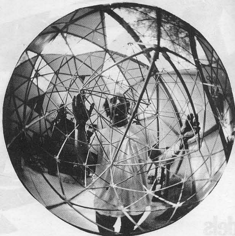
Three-frequency sphere with icosahedron suspended inside.
