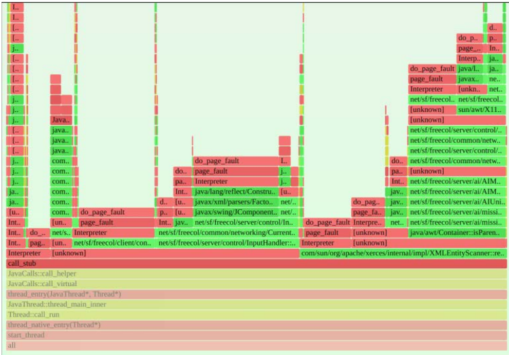
Figure 12-8 Page fault flame graph
