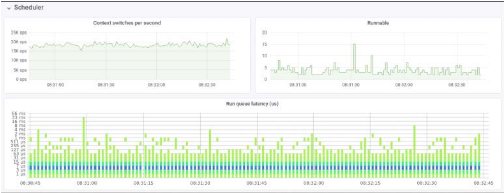
Figure 17-12 Grafana PCP, showing standard PCP metrics (context switches, runnable count) as well as run queue latency (runqlat) BCC metrics
