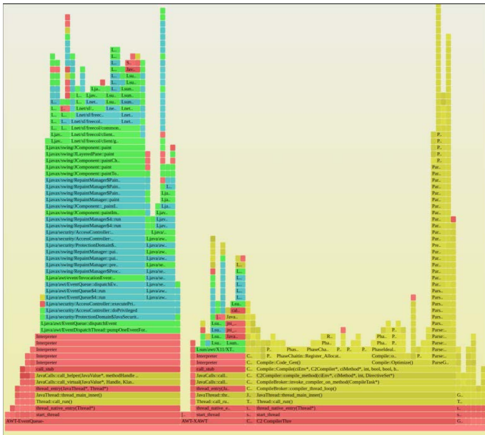
Figure 12-4 CPU flame graph with uninlining
