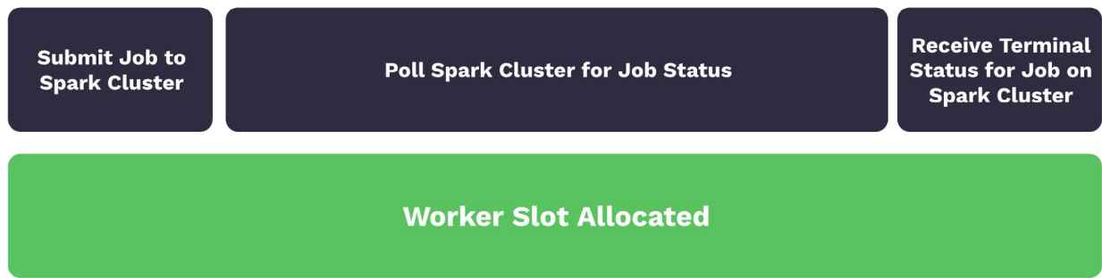
Figure 3: Graph showing a regular operator using up a worker slot while polling a spark cluster for a job status.
