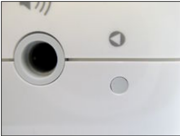
Figure 1: The reset button is located below the reversed-out white triangle; here, it's next to the audio port of an AirPort Express.
