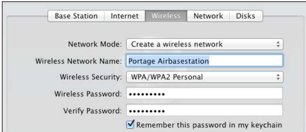
Figure 75: Set up a main base station by letting it create a network and allow its extension.
