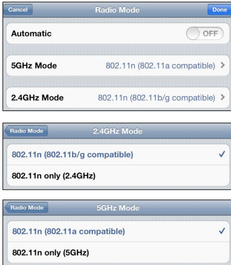
Figure 33: The Radio Mode screen (top) lets you choose from two major options for the 2.4 GHz band (middle) and for the 5 GHz band (bottom).
