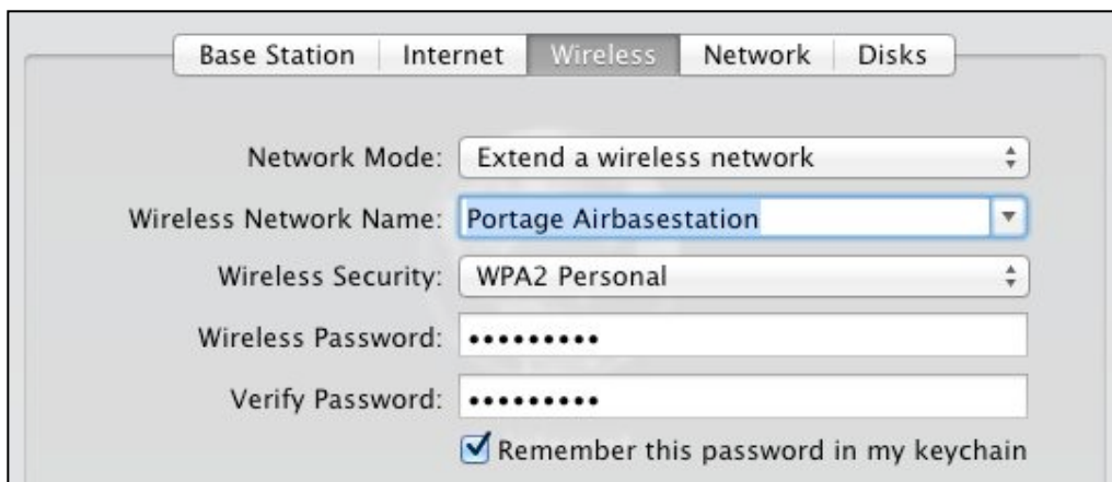
Figure 76: Other base stations connect to the main by its network name, and can optionally allow Wi-Fi connections from clients.
