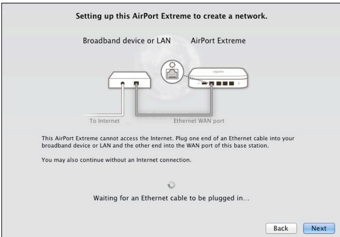
Figure 20: Plug in your Ethernet cable if you haven't already, or check your cables.
