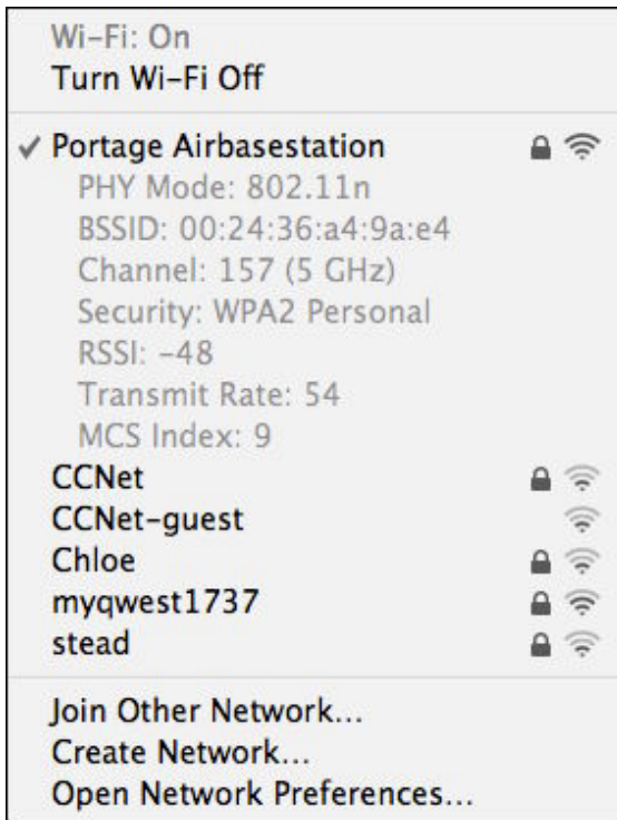
Figure 57: Hold down Option while opening the Wi-Fi menu to see additional details about the network that you’re connected to.
