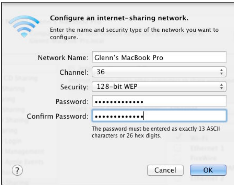
Figure 102: Set the wireless options you want for your software base station, including a WEP password.
